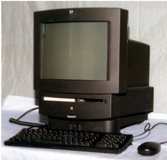
Figure 11.3. The Macintosh TV was made by assembling a Sony Trinitron TV and an Apple Performa computer (source: http://archive.wired.com/gadgets/mac/multimedia/2008/01/gallery_apple_flops?slide=4&slideView=2 )
