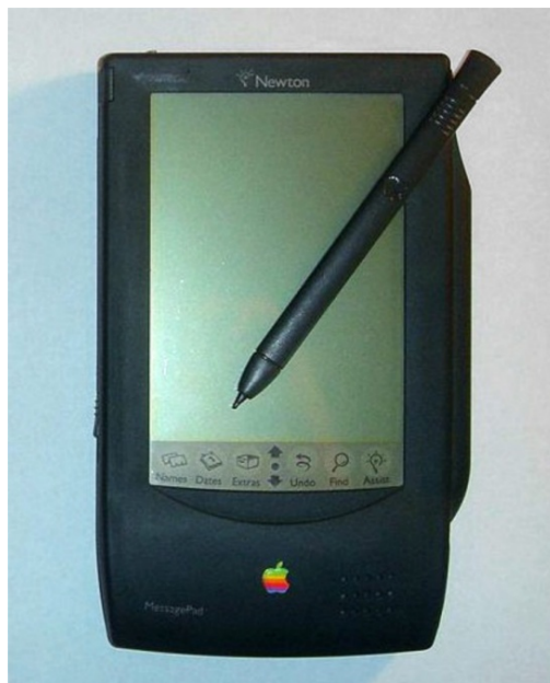
Figure 11.2. The so-called Newton pad had a stylus and could access databases (source: http://archive.wired.com/gadgets/mac/multimedia/2008/01/gallery_apple_flops?slide=4&slideView=2 )
