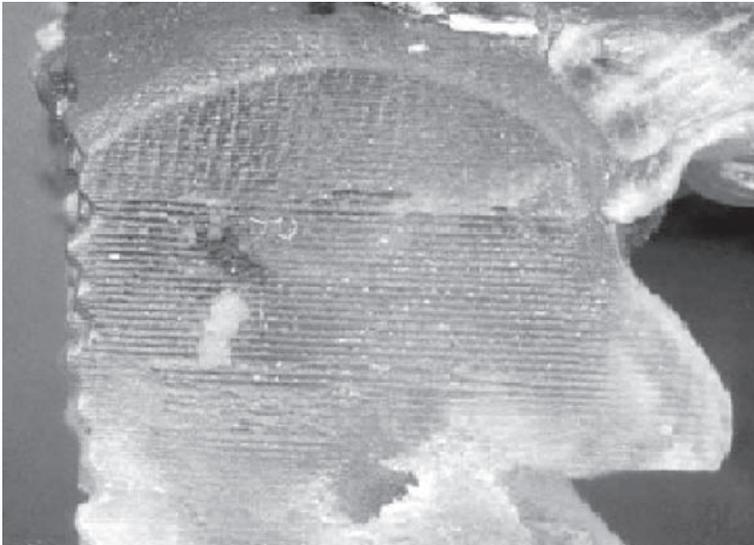
6.8 Showing surface roughness on an SL model attributed to support structures.
