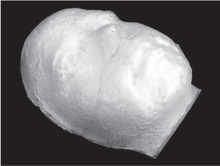
6.49 Plaster filled SL mould.
