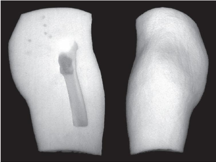
5.27 CNC machined foam model of the soft tissue of the hip.
