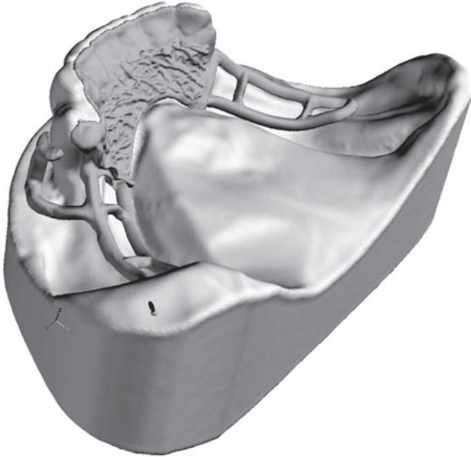
6.86 The RPD framework designed in FreeForm® CAD.
