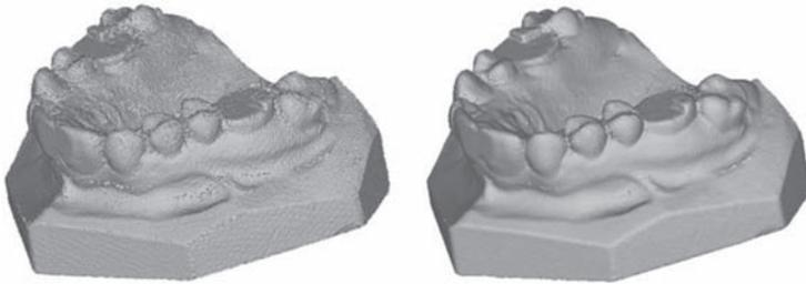
2.17 Scan data showing noise (left) and the same data with noise reduced (right).
