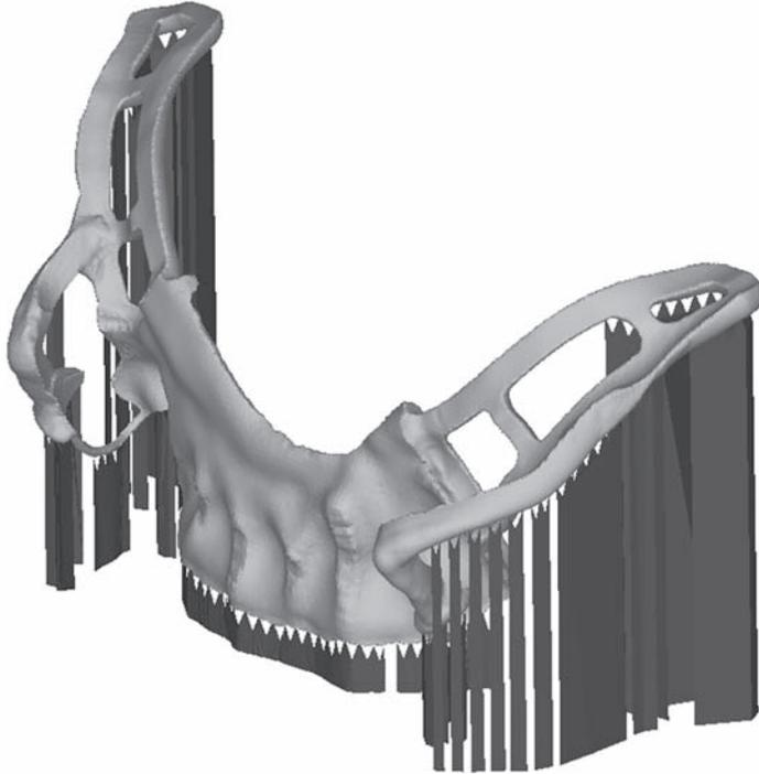
6.87 RPD oriented and supported to avoid the fitting surfaces.
