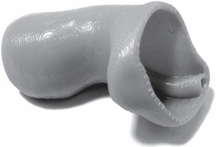
5.14 A hearing aid shell manufactured using DLP™.
