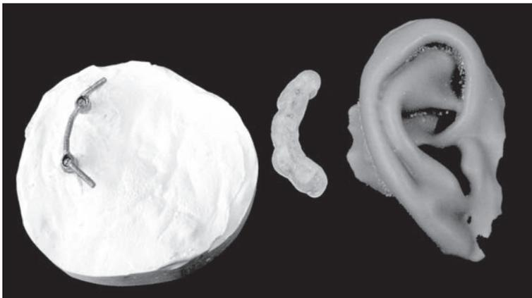
6.75 The manufactured components: SLM<sup>™</sup> bar (left), Stereolithography sub-structure (middle) and ThermoJet<sup>®</sup> pattern (right).
