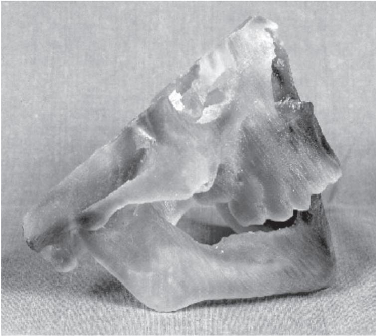
*6.9a* Smooth surface due to high-resolution meshing algorithm.
