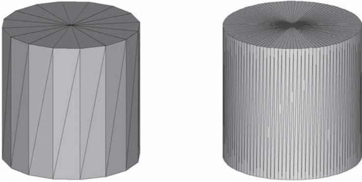
4.20 The effect of deviation settings: (left) large deviation = small file and (right) small deviation = large file.
