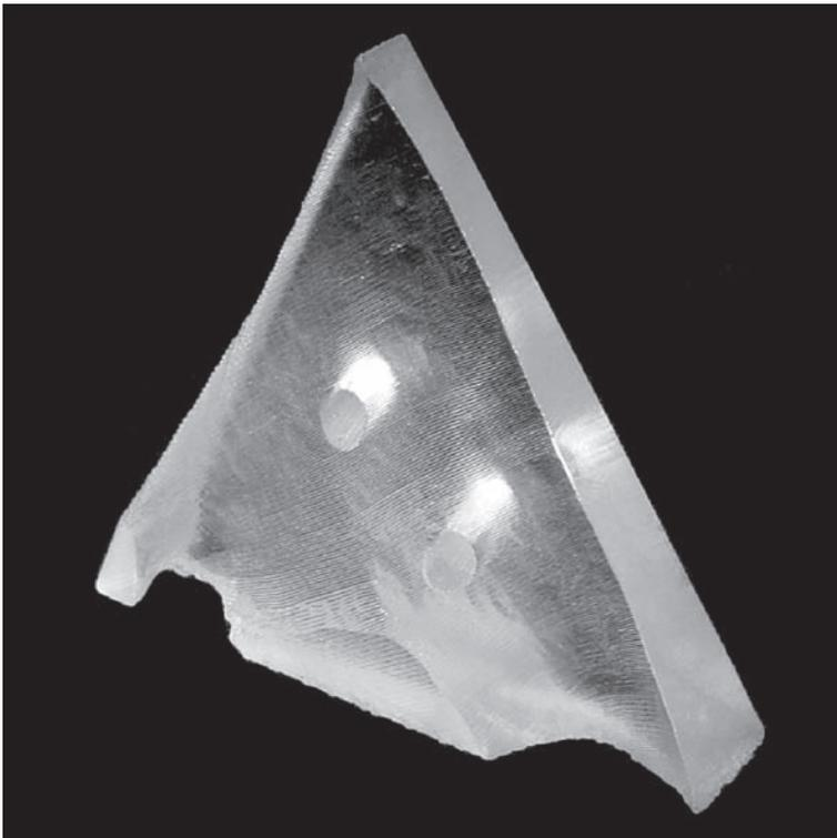
6.19 The final template produced directly using stereolithography.
