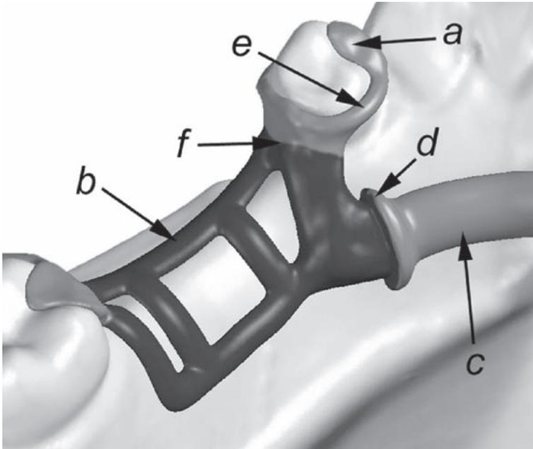
6.80 a = occlusal rest, b = polymeric retention frame, c = lingual bar, d = acrylic line, e = non-active clasp, f = guide plate.
