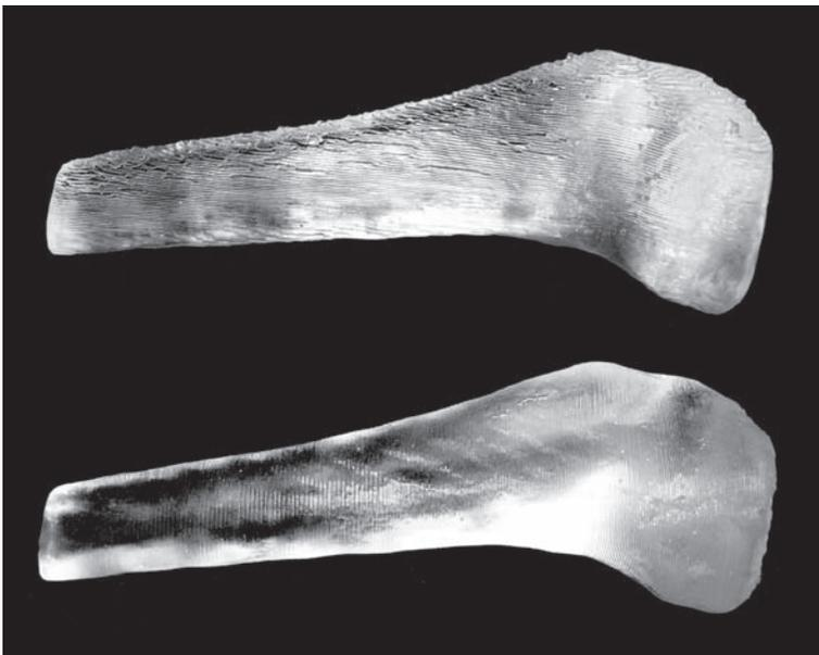
5.5 The stair step effect of build orientation.
