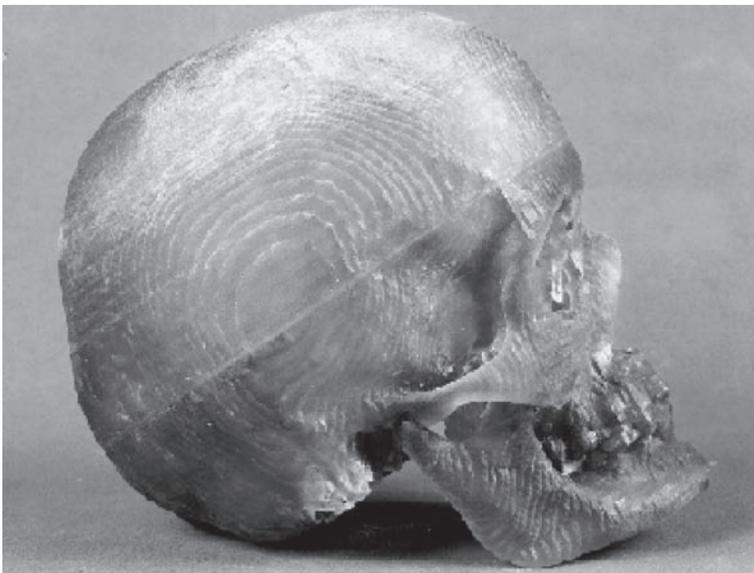
*6.9b* Meshing contours visible due to low-resolution meshing algorithm.
