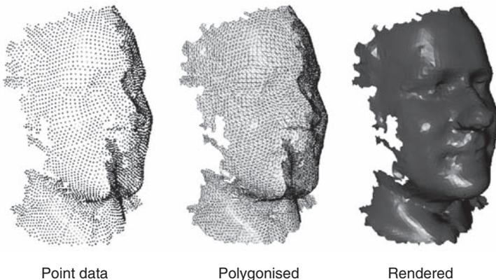
4.11 A triangular polygon mesh created from a point cloud.
