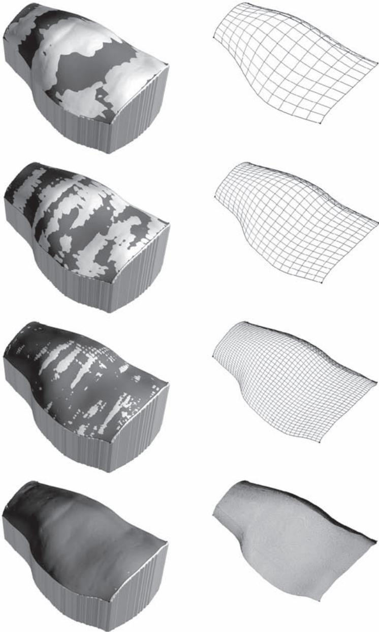
4.22 The effect of the number of control points on IGES patch quality, (from top) 6 control points, 10 control points, 20 control points and 100 control points.
