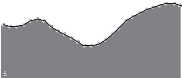
2.16 The effect of filtering to remove noise from optical scan data.
