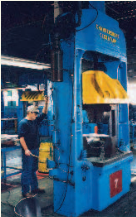
Figure 3. A drop hammer used for sheet metal forming. A finished part is shown in the lower left-hand corner.
