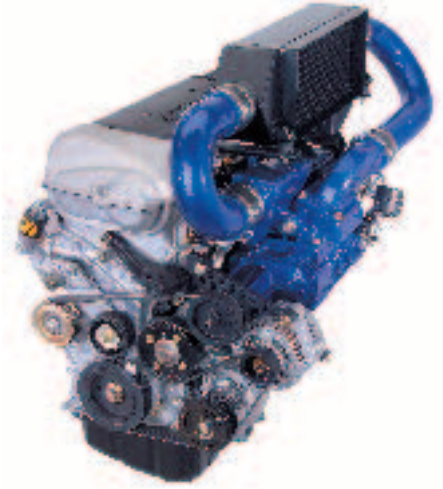
Figure 9.8 Engine for a Lotus Sport Exige 240R sports car. This engine has 4 cylinders and produces 243 hp. The belt wraps around 7 pulleys and is needed to operate a variety of essential engine accessories such as the power steering pump and alternator. The belt and pulleys must be designed so there is no slip.
