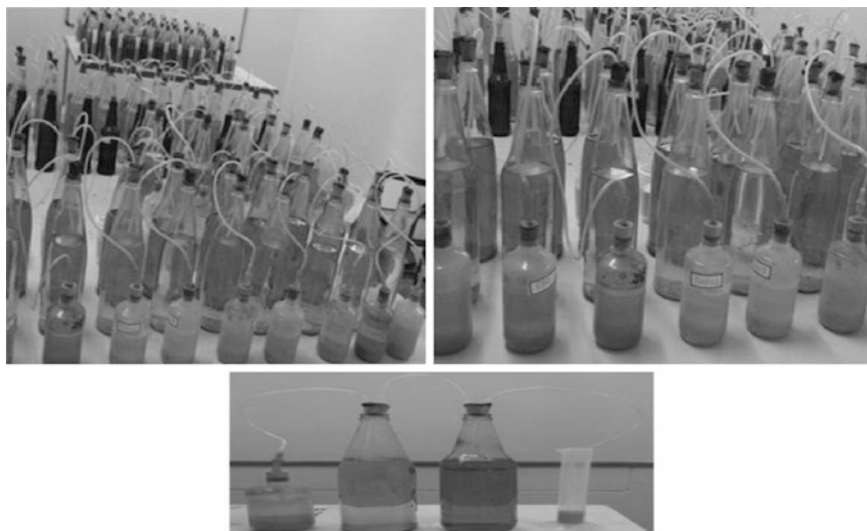
Fig. 1 Biochemical methane potential assay setup for methanogen screening
