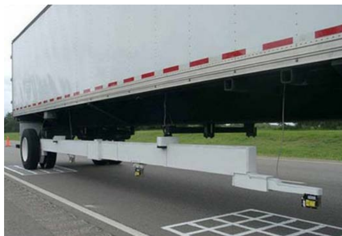
Figure 4-7. Rolling Wheel Deflectometer (FHWA 2008d)
