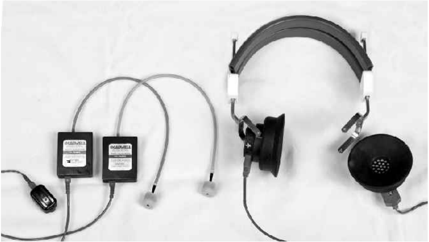
Fig. 6.2. Auditory stimulus transducers used to elicit the brainstem auditory evoked response (BAER). Headphone cups can be removed from the headband and held over the ear canal opening. Insert earphones can be inserted into the ear canal, but are usually held at the canal opening. The bone stimulus transducer is held against the skull over the mastoid process.
