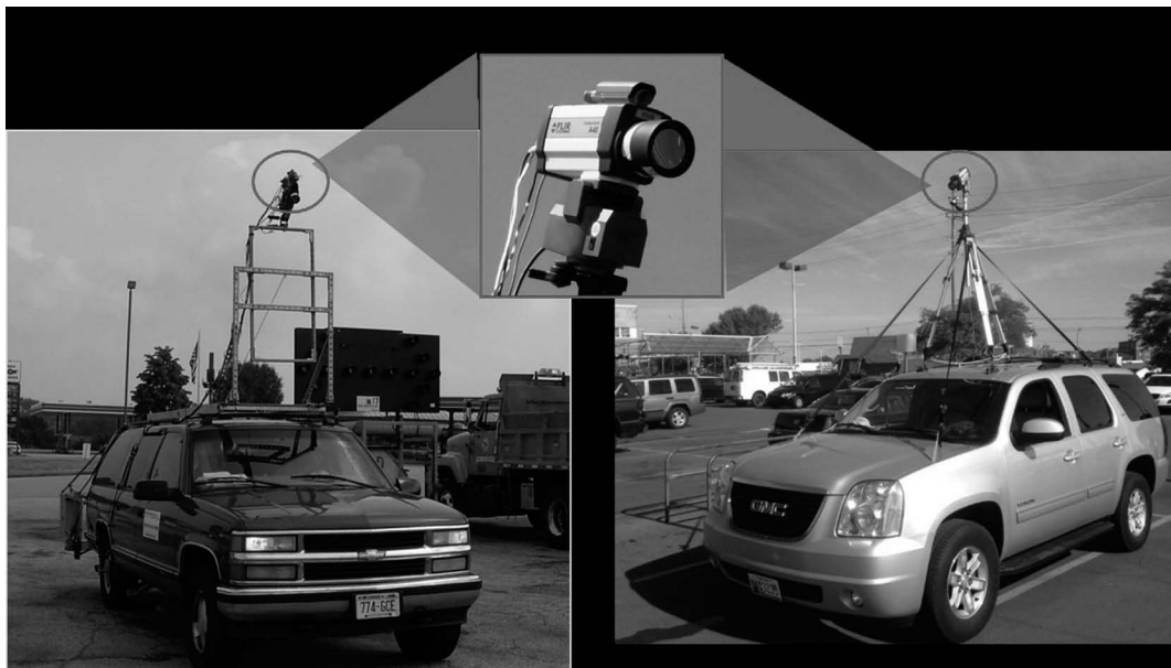
FIGURE 22.12 Infrared camera used for pavement survey. (Courtesy of Dr. Ken Maser.)
