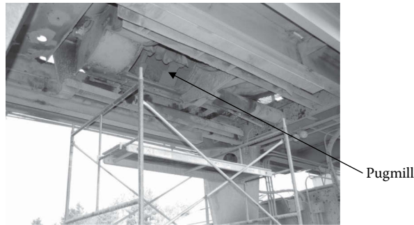
FIGURE 13.7 Pugmill, view from the bottom with discharge door removed. (Courtesy of Matthew Teto, All States Asphalt, Sunderland, MA.)
