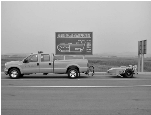
FIGURE 20.5 Skid tester. (Courtesy of David Morrow, Dynatest Consulting Inc., Ventura, CA.)
