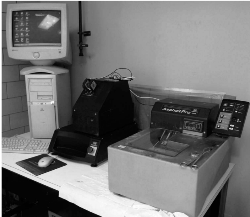
FIGURE 9.14 Direct tension testing equipment. (Courtesy of Denis Boisvert and Alan Rawson, New Hampshire Department of Transportation, Concord, NH.)
