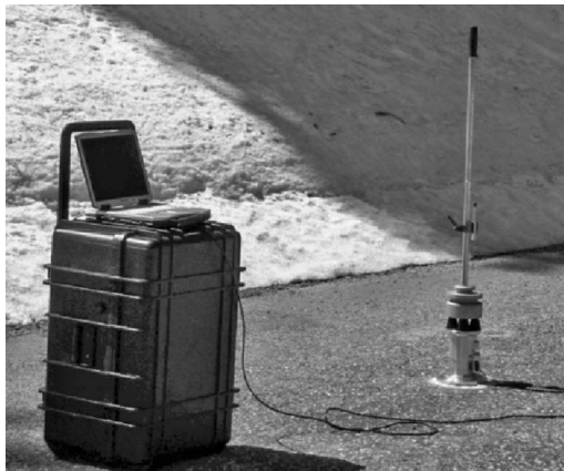
FIGURE 22.4 Portable falling weight deflectometer. (Courtesy of Maureen Kestler/Michael Santi.)
