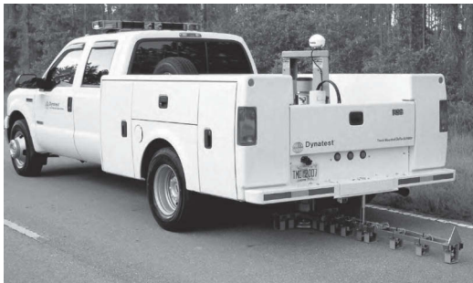
FIGURE 22.3 Truck mounted deflectometer (tmd) and fast falling weight deflectometer (ffwd). (Courtesy of Dynatest.)
