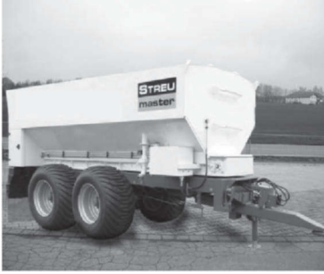
Wirtgen SW 16TA lime spreader Tank capacity: 16.5 m 3 , Spreading width: 2500 mm Spreading quantity: 2–50 L/m 2 , Manual operation spreading auger
