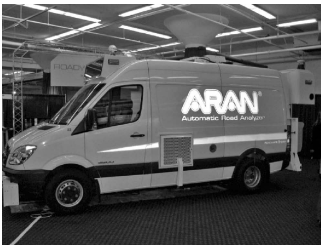
FIGURE 20.3 Automatic road analyzer.
