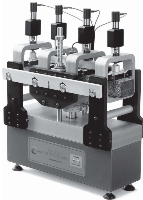
FIGURE 11.1 Fatigue tests of asphalt mix beam. (Courtesy: IPC global.)
