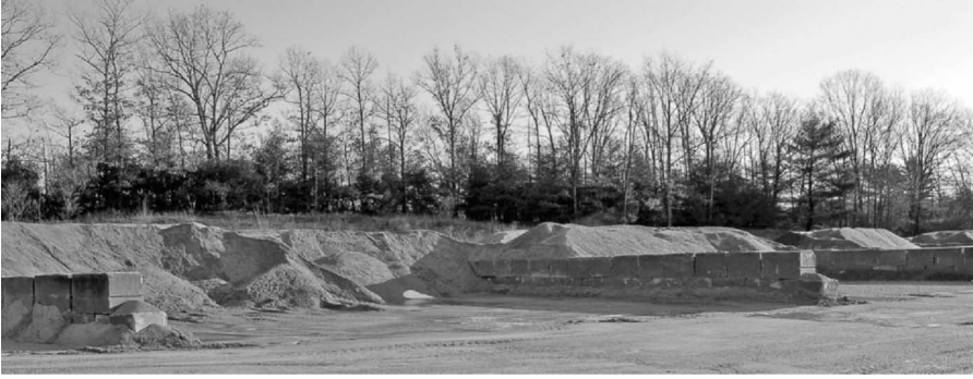
FIGURE 13.3 Aggregate stockpiles. (Courtesy of Matthew Teto, All States Asphalt, Sunderland, MA.)
