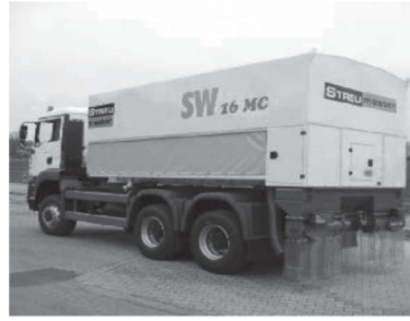
Wirtgen SW 16MC lime and cement spreader Tank capacity: 16.5 m 3 , Spreading width: 2460 mm Spreading quantity: 2–50 L/m 2 , Cellular wheel automatic operation
