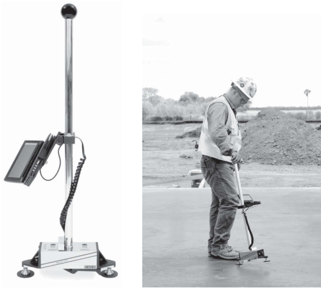
FIGURE 19.4 Dipstick. (Courtesy of Face Construction Technologies, Norfolk, VA.)
