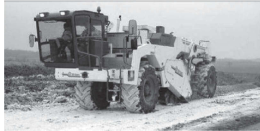
Lime stabilization with Wirtgen WR 2000 Working width: 6 ft 7 in., Working depth: 0–20 in. Engine output: 400 HP, Weight: 49,060 lb
