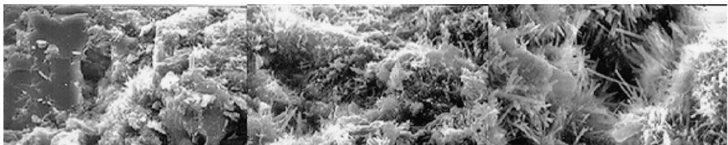
FIGURE 14.3 Scanning electron micrograph showing cement hydration products at various ages; phases include CSH, Ca(OH)_2 , and Ettringite.
