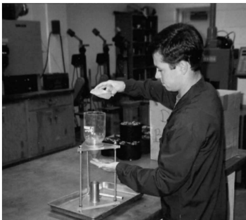
FIGURE 8.8 Testing for uncompacted voids for fine aggregates.
