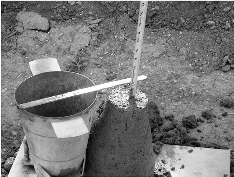
FIGURE 17.24 Field testing of concrete consistency using the slump test. (Courtesy of James Cable.)
