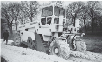
Lime stabilization with Wirtgen WR 2500 Working width: 8 ft, Working depth: 0–20 in. Engine output: 690 HP, Weight: 63,000 lb
