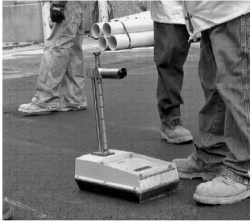
FIGURE 22.1 Schematic of backscatter operation and nuclear gage equipment gage used on HMA.
