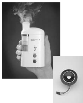
B. Ultrasonic nebulizer with illustrative transducer
