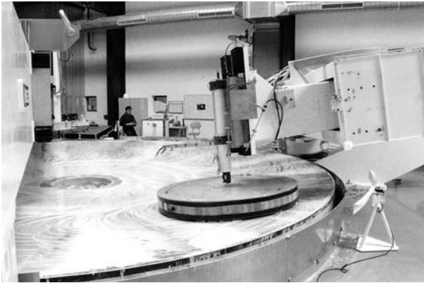
Fig. 4.39. Computer-controlled lapping of an 8-meter mirror for the VLT (Courtesy of REOSC).
