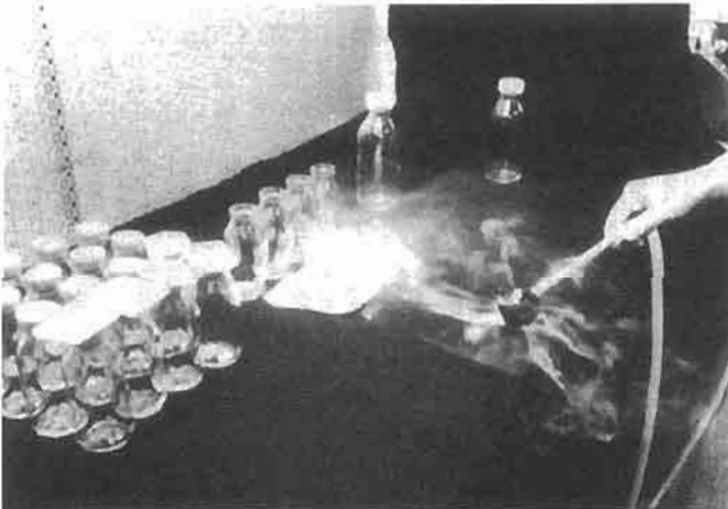
FIGURE 10.60 Dispersion of smoke in a horizontal flow bench (wake region behind small bottles).
