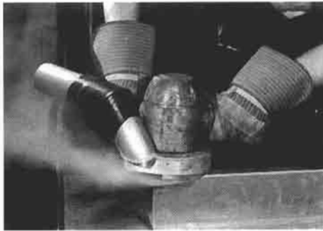
(b) Roughly fabricated nozzle for a hand-held cup-wheel grinder
