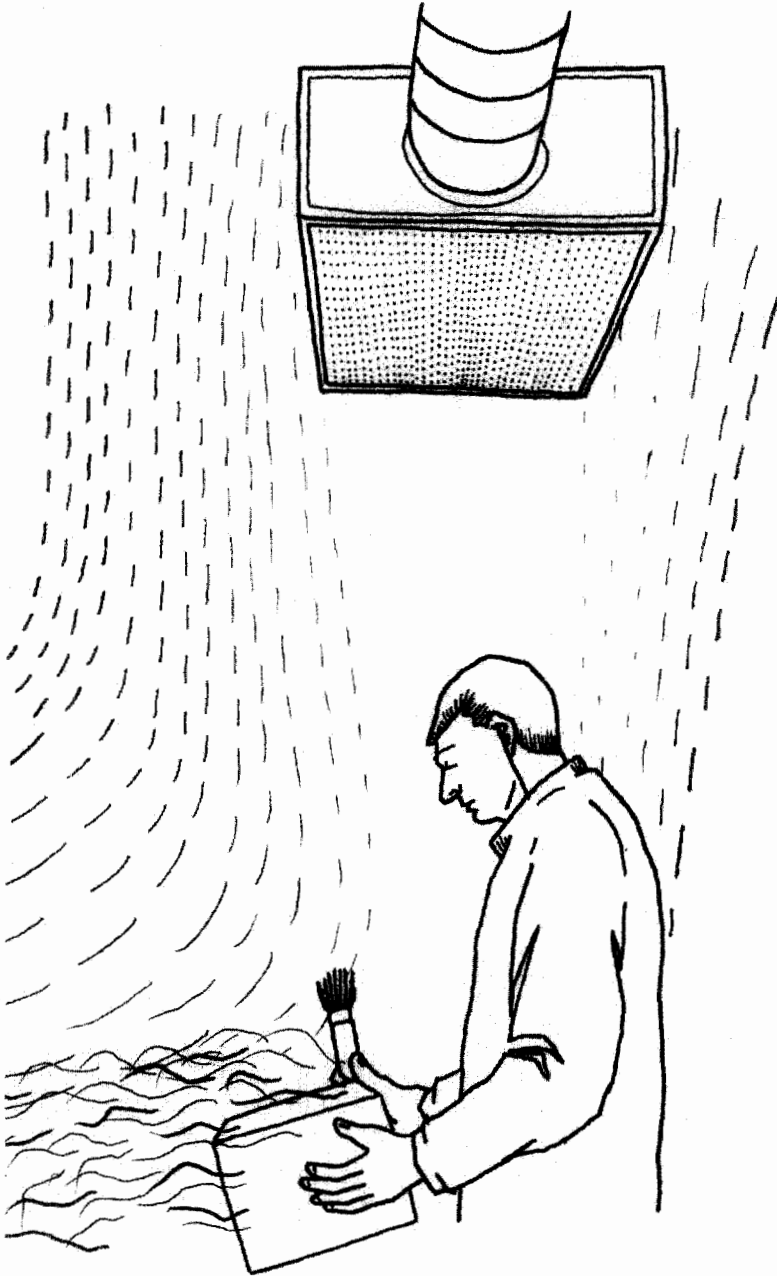
FIGURE 10.48 The air shower principle creates a zone of clean air around the worker and pushes the contaminant plume away from the breathing zone.
