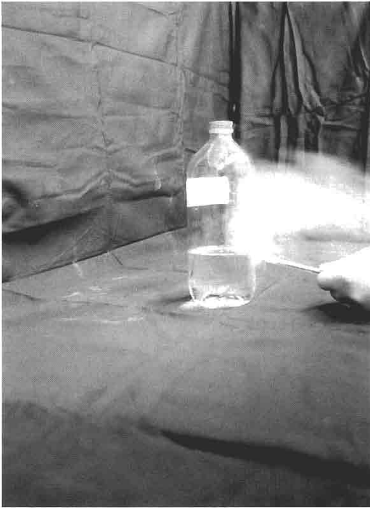
FIGURE 10.58 Dispersion of smoke behind a bottle placed in the bench shown in Fig. 10.57.
