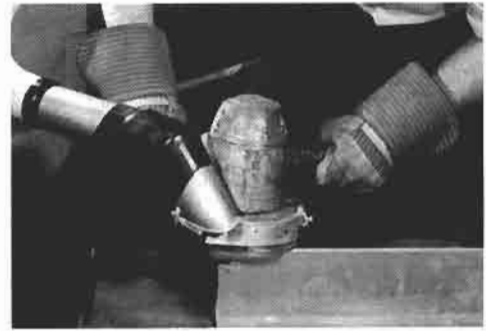
(b) Roughly fabricated nozzle for a hand-held cup-wheel grinder
