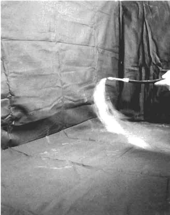
FIGURE 10.57 Undisturbed smoke dispersion in the bench shown in Fig. 10.53 at an air velocity of 0.45 \text{ m s}^{-1} .
