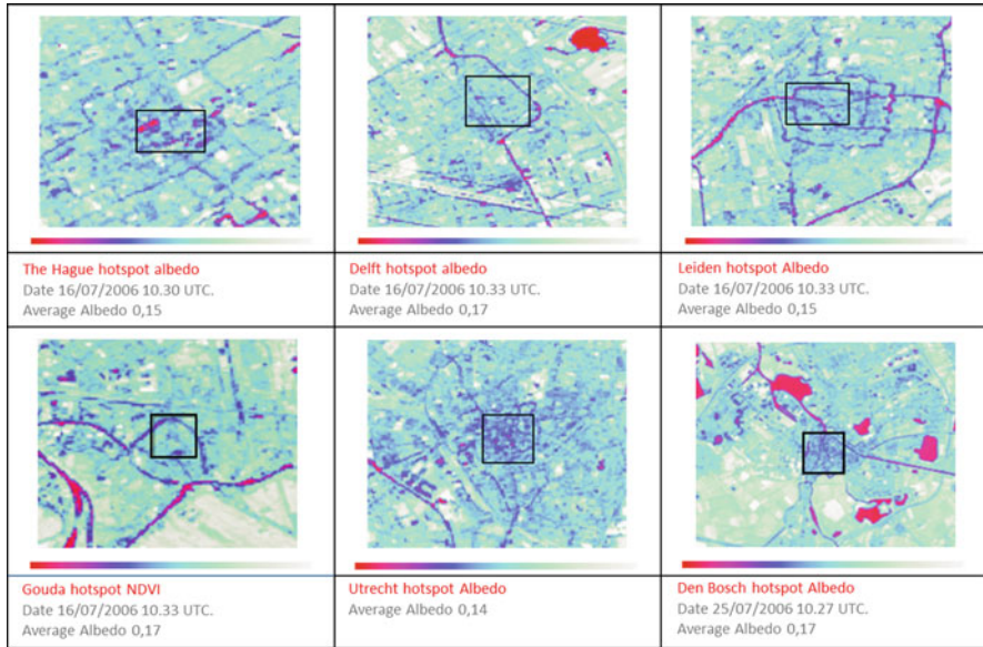
Fig. 7.10 Albedo of the different Dutch cities. Landsat image (Courtesy of the U.S. Geological Survey. USGS/NASA Landsat) further processed with ENVI 4.7 and Atcor 2.3
