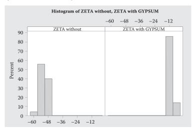
The addition of calcium/gypsum increases the values of the zeta potential of silica. All of the values of zeta potential for the specimens containing calcium/gypsum are greater than all of the values of zeta potential for the specimens without calcium/gypsum.
