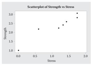
The relationship between shear strength and precompression stress appears to be linear. As precompression stress increases, shear strength tends to increase.
