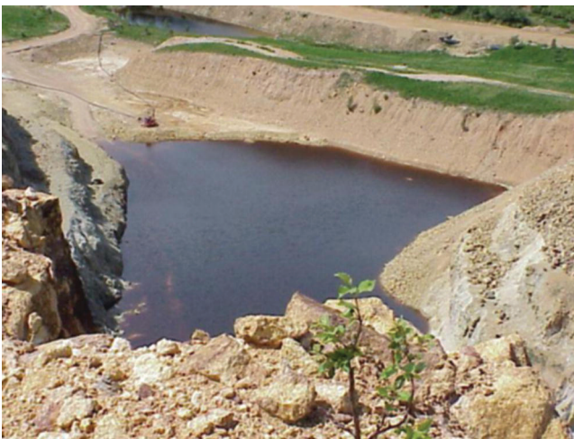
FIGURE p10.28 An acid rock drainage pit at an abandoned gold mine in sulfide-bearing rock.
