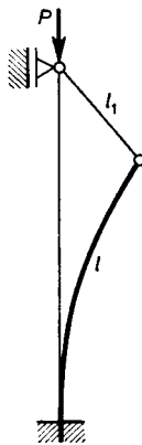
Fig. 2.13. Example of a bar whose postcritical behaviour may be unstable
