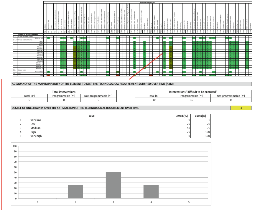
Fig. 6.12 Example of traceability of a level of risk to its causes: the “ease of operation and handling” of the window 1 in building 2
