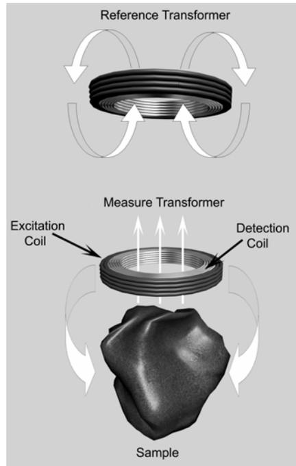
Figure 12. Functional diagram of the single sensor AC Biosusceptometer.
