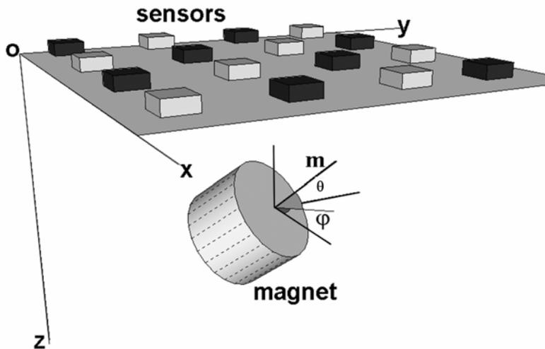
Figure 11. Magnetic tracking system. (Modified from Schlageter et al., 2002, with permission).
