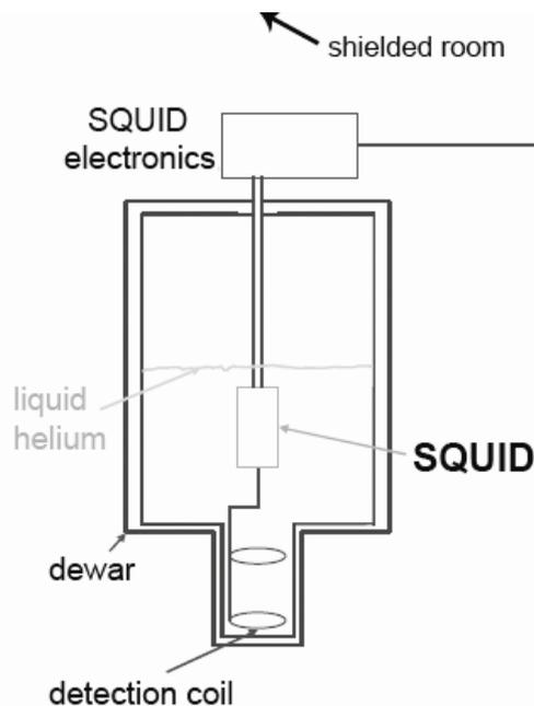
Figure 5. Schematic diagram of a single channel SQUID system. (Modified from Pizzella et al., 2001, with permission).
