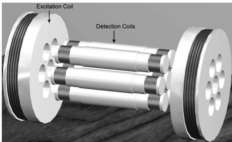
Figure 13. Multisensor AC Biosusceptometer system with the pairs of detection coils in hexagonal symmetry.
