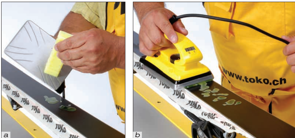
Waxing the ski with an iron. Wax is dripped onto the base and then ironed.
