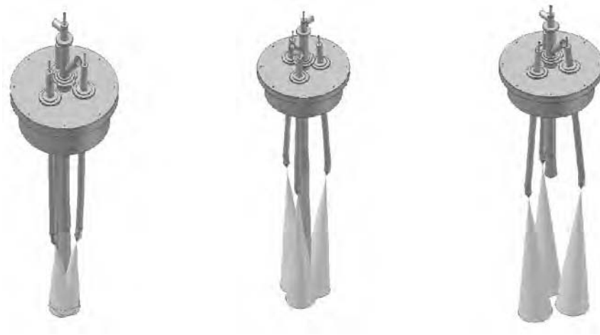
Fig. 16.6 Nozzle set (three nozzle sticks and one central fines return) having the possibility to alter the pitch of the nozzles relative to the fines return. Narrow pitch (left) will lead to maximal primary and secondary agglomeration. Wide pitch and switching off fines return to the atomisation zone (right) will lead to minimal primary agglomeration and no secondary agglomeration (courtesy of Carlisle Processing Systems – Friesland, patent pending).
