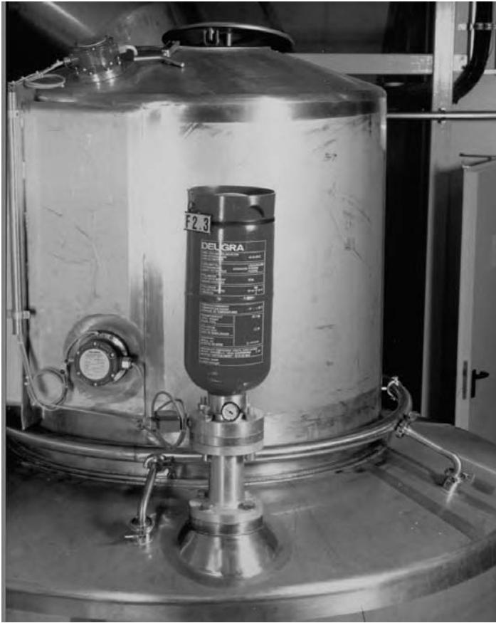
Fig. 16.19 Commercial explosion suppression system mounted on top of a cyclone (courtesy of Anhydro A/S).
