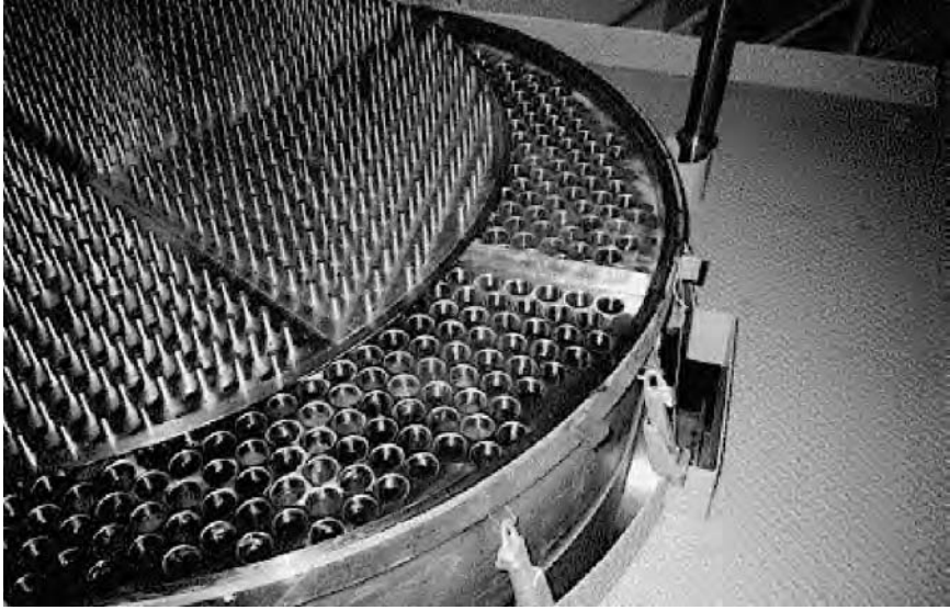
Fig. 16.2 Example of an industrial liquid distribution device (courtesy of Carlisle Processing Systems – Friesland).
