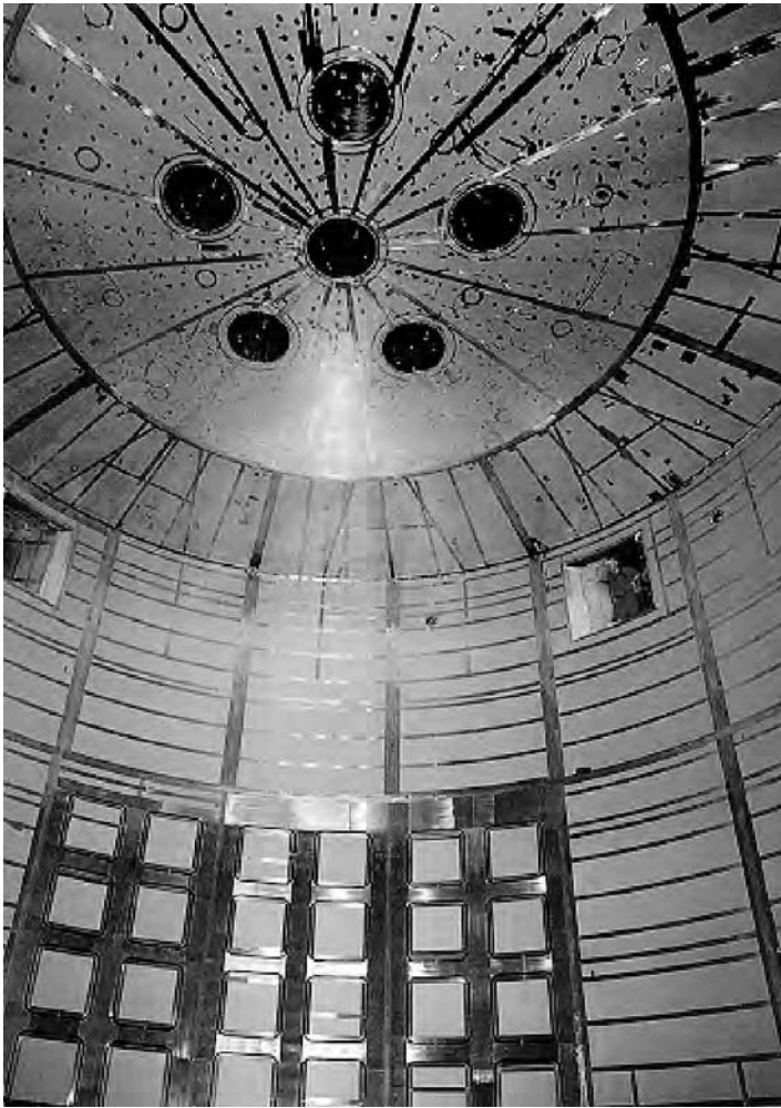
Fig. 16.18 Inside of an industrial spray dryer with atomisation units at the top and explosion venting panels at the spray chamber wall (courtesy of Carlisle Processing Systems – Friesland).
