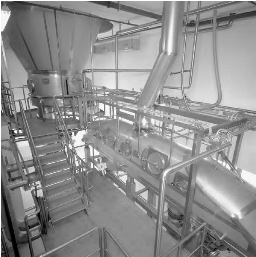
Fig. 16.4 The bottom of a spray chamber incorporating an internal fluid bed and an external fluid bed (courtesy of Anhydro A/S).
