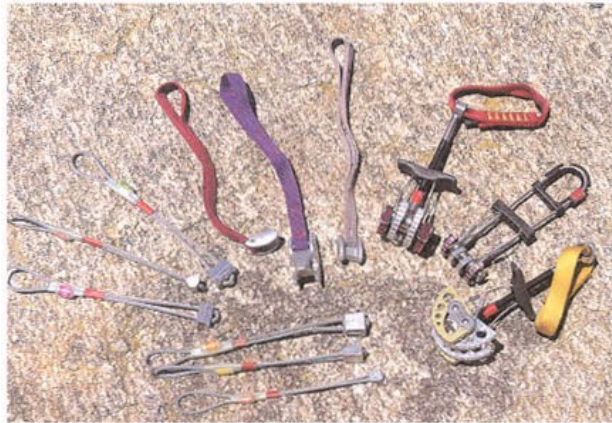
Artificial anchors (clockwise from bottom): wired nuts, wired hexcentrics, Tri-Cams, SLCDs.
