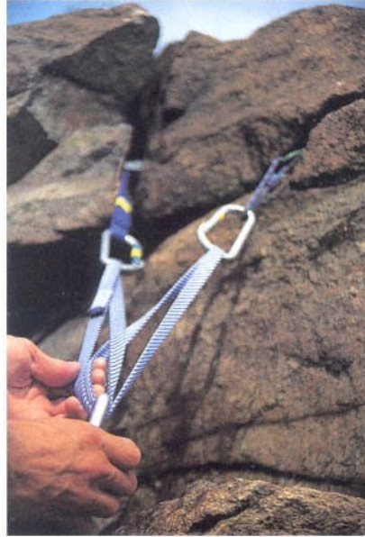
Using a single runner as a self-equalizing slider to connect two anchor points.
