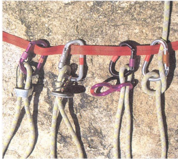
Belay devices (left to right): ATC plate, Sticht Plate, Figure-8 ring, Munter Hitch.
