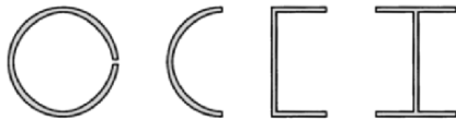
Figure 6.33 Open thin-walled cross-sections can be considered to be built up of thin-walled strips. So the formulas derived for a thin-walled strip can also be applied to open thin-walled cross-sections. Circular or other curved parts can be considered as strips, on the condition that the wall thickness is far smaller than the radius of curvature of the strip.
