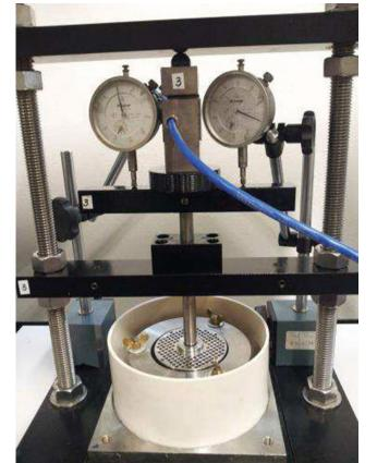
Fig. 154.1 Axial swelling stress in manual press
