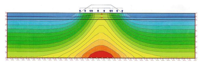
**Fig. 54.3** SIGMA/W solve analysis results with isolines of vertical H = 10 m; water table depth:  $h_w = -5$  m; thickness of compressible
