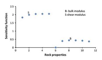
Fig. 79.7 Variation of sensitivity factor with bulk and shear modulus
