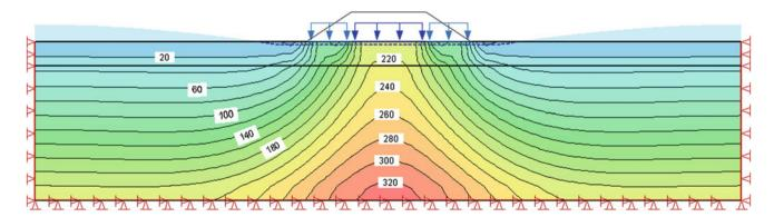
Fig. 54.4 SIGMA/W solve analysis results with isolines of vertical stresses distribution (kPa) for an hypothetical embankment. Height H = 10 m; water table depth:  $h_w = -1$  m; thickness of compressible
