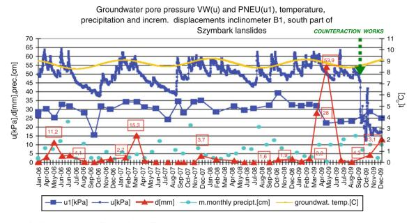
Fig. 32.5 Monitoring measurements Szymbark landslide
