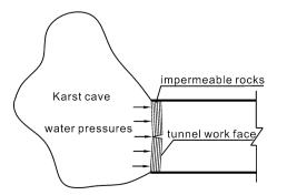
Fig. 78.2 Water inrush due to bending failure of impermeable rock wall
