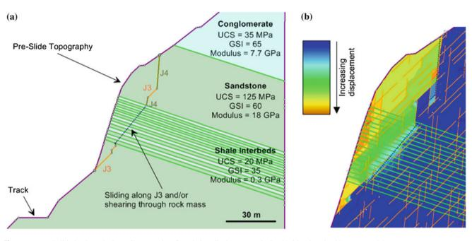
Fig. 36.4 Rockslide back-analysis. a Cross section. b Relative displacement obtained with Phase2 with DFN model
