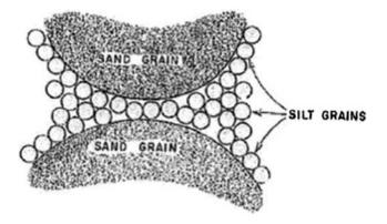
Fig. 1.3 Schematic arrangement of silt grains between two sand grains
