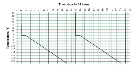
The testing process consists of two freezing-thawing cycles. The bottom temperature remains stable at 4 °C, while the top of the soil column is gradually cooled by 2 °C per day until it reaches -20 °C. After each cycle stage, 3 columns of soil are collected for further tests. The experiment is run using different de-icing agents and with deionized water, to permit a comparison.
