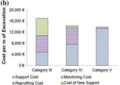
installation of new support) for each liner category (costs are per metre of tunnel)
