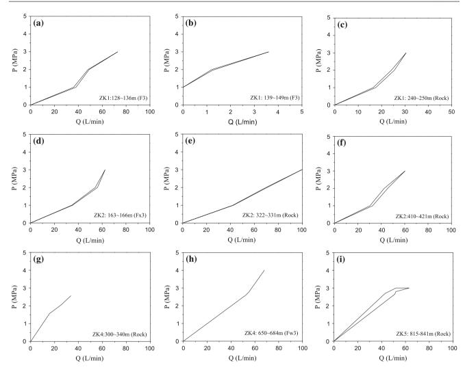
Fig. 104.3 The P-Q curves of high-pressure water injection test in tunnel site area
