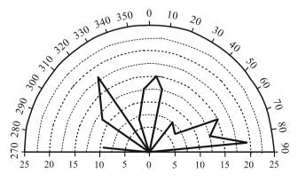
Fig. 104.2 The strike of joints rose diagram in tunnel overlay surfaces area
