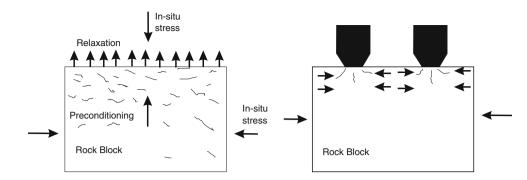
Fig. 76.3 Schematic of numerical models used to investigate the effect of stress on: (*left*) preconditioning at face; (*right*) fracture initiation and propagation at cutter-rock interface; face is at *top*
