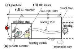
Fig. 187.2 Conceptual diagram of the measurement
