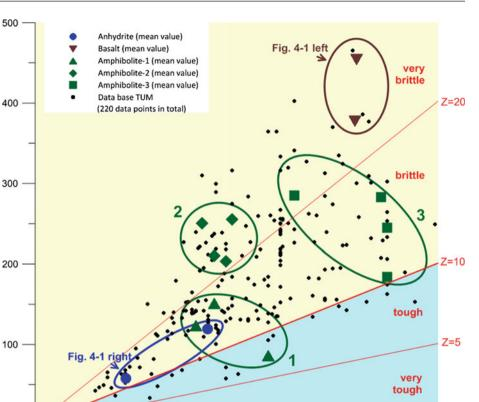
**Fig. 82.4** Mean Z coefficient of analyzed rock types plotted against the ratio of destruction work to failure energy. Colored background describes post failure behavior at uniaxial compression test
