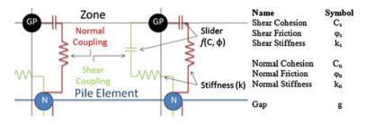
Fig. 157.3 Ideal illustration of normal and shear interaction of the pile element on the zone. Interface elements connecting the forepole (pile element) with the rock (zone)
