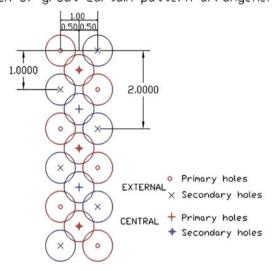
Fig. 14.3 Grouting pattern
