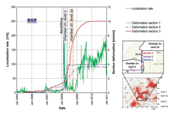
Fig. 99.3 Results of AE and deformation measurements before, during and after backfilling of chambers 2a on level 2 and level 2a
