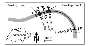
Fig. 75.1 Analyzed cross-sections and swelling zones of the Chienberg tunnel
