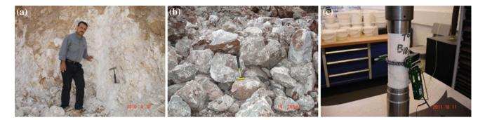
Fig. 139.2 a Gypsum outcrop, Bazyan/Iraq b Bantycock Mine/UK gypsum blocks c The extensioneter in the mid-length of a cylinder
