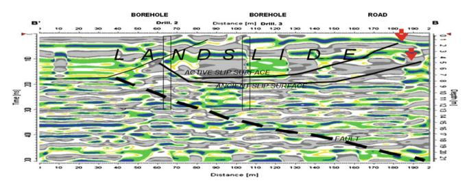
Fig. 32.3 GPR profile Sekowa landslide
