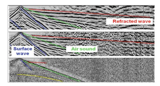
**Fig. 189.2** Raw data of the different tested sources *top* accelerated weight drop, *middle* sledgehammer, *bottom* air sound
