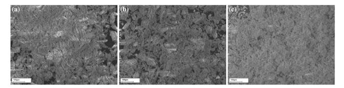
Fig. 139.4 Variations in gypsum crystal size, visualized using SEM: a The white/Bantycock gypsum. b The pink/Bantycock gypsum. c The Iraqi gypsum
