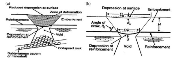
Fig. 68.3 a Conceptual role of reinforcement in limiting surface deformations due to subsidence, BS-2006. b Parameters used to determine reinforcement, BS-2006
