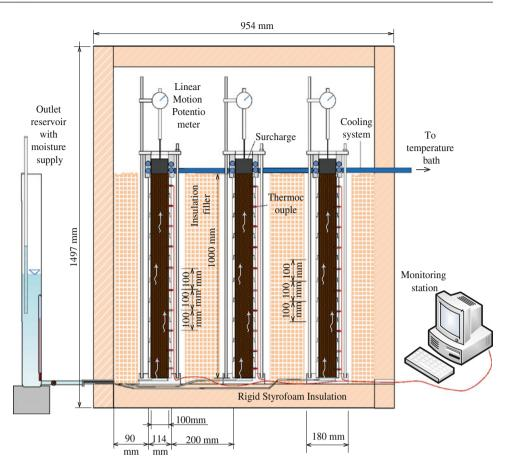
temperature controlled cabinet are connected to a constant head (Mariotte) supply reservoir, and chilled from the top. A schematic representation of the test equipment is presented on Fig. 39.4.
