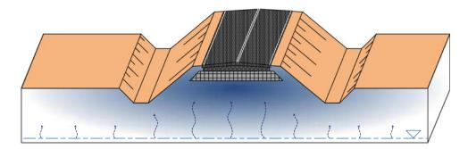
Deposition of de-icing salts in the roadside inevitably changes the chemical content and moisture regime of the subsoil. This may have a great effect on its bearing capacity, especially during seasonal freeze-thaw cycles. Furthermore, it keeps the moisture of the nearby soil in a liquid state (Kane et al. 2001).
