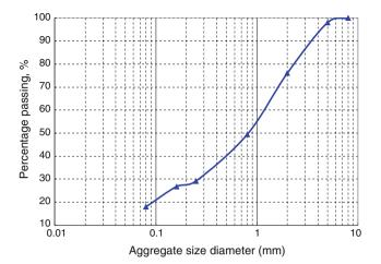
Fig. 85.2 Aggregate size distribution of the crushed soil
