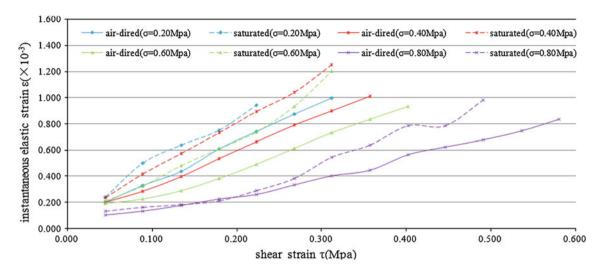
Fig. 158.2 The curves of shear stress-instantaneous strain
