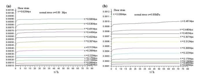
Fig. 158.1 Sheer creep curves under the normal stress of 0.800 Mpa a air-dried sample D#<sub>1</sub>, b saturated sample D#<sub>2</sub>
