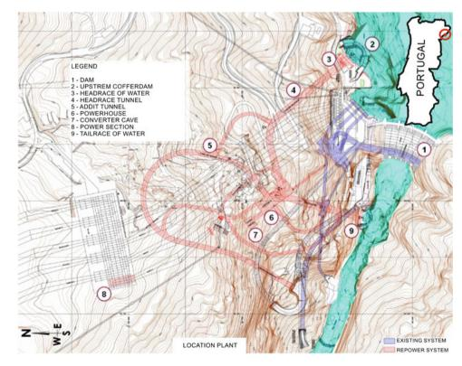
**Fig. 72.1** Components of Picote II (Portugal) repowering scheme (EDP 2006, modified)
