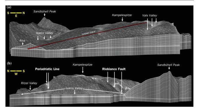
Fig. 177.3 3D geometry and meshes used for the numerical model of the Aica-Mules tunnel
