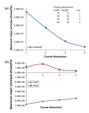
Fig. 79.4 a Variation of maximum principal stress with excavation volume of the arched-roof tunnel. b Variation of maximum principal stress magnitude and type with varied height to width ratios
