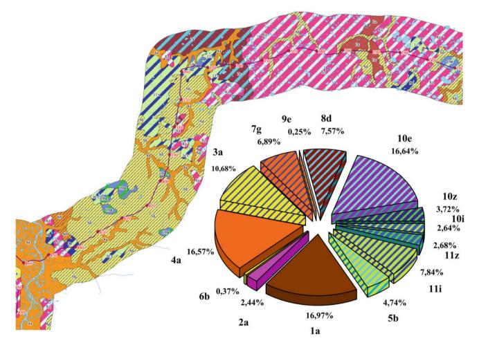
**Fig. 64.2** The schematic geotechnical cartographic model (fragment of the design solutions map of pipeline route). Diagram presents percentage of the total length of all selected areas with different design solutions. Indexes (1a, 2a, ..., 11z) show types of engineering-
