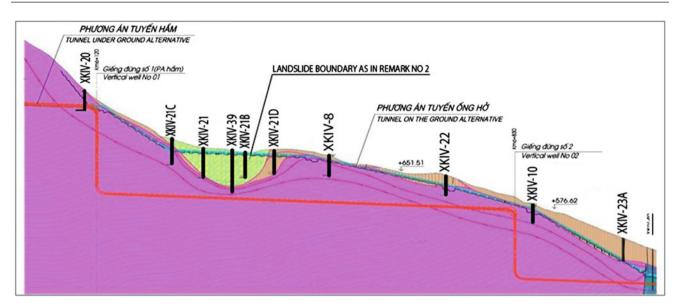
Fig. 65.1 Landslide boundary at penstock based on Remarks No 1 and No 2
