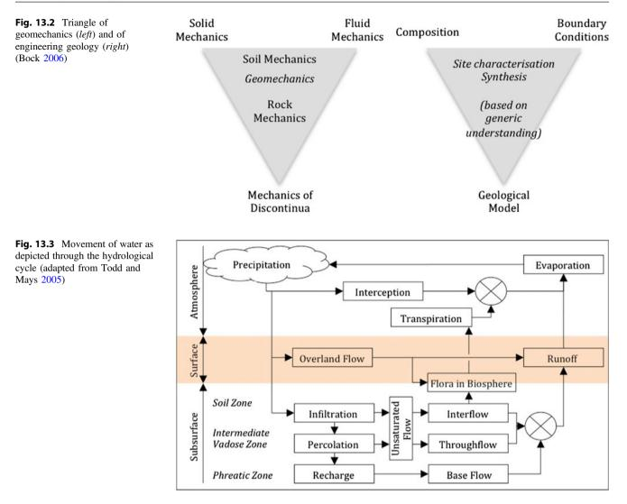
distinct exclusion of the deeper intermediate vadose zone (Fig. 13.3). Numerous aspects have to be considered when compiling a comprehensive vadose zone model. Some of these are illustrated in Fig. 13.4 and indicate the vast range of input in such conceptual models (Dippenaar et al. 2014):
