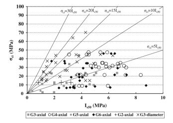
**Fig. 71.3** Correlation between the results  $I_{s(50)}$  and  $\sigma_{ci}$  values for the rocks: (i) G2: Schists, (ii) G3: Metasiltstones, (iii) G4: Limestones, (iv) G5: Gabbro, (v) G6: Peridotite
