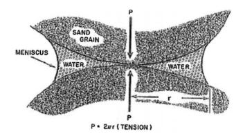
Fig. 1.2 Capillary produced contact pressure
