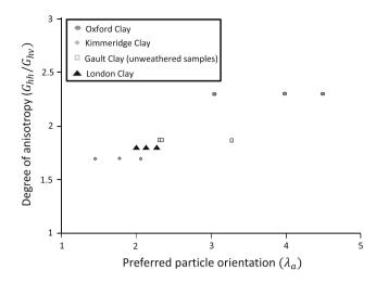
Fig. 144.3 Plot of the degree of anisotropy of stiffness and measurements of preferred particle orientation
