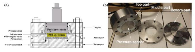
Fig. 85.1 a Schematic diagram of the constant-volume cell; b picture of the three parts of the constant volume cell
