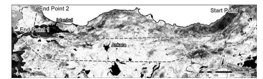
Fig. 48.2 Combined constraint map, costs increase from white to black, *dashed line* indicates derived project corridor
