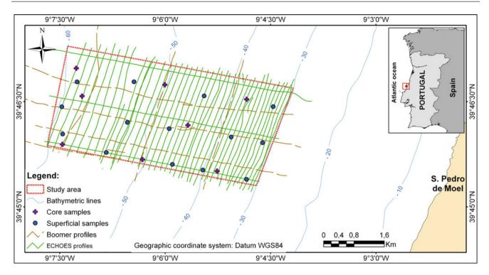
Fig. 69.1 The study area and location of seismic profiles, superficial and vertical sediments sampling
