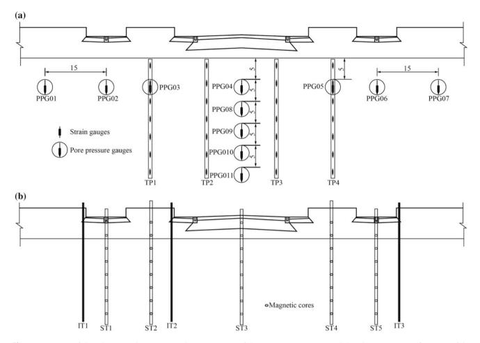
Fig. 29.4 Layout of the substructure instruments (unit: m). a Layout of the pore pressure gauges and the wire stress gauges, b Layout of the settlement tubes ST and the inclinometer tubes IT
