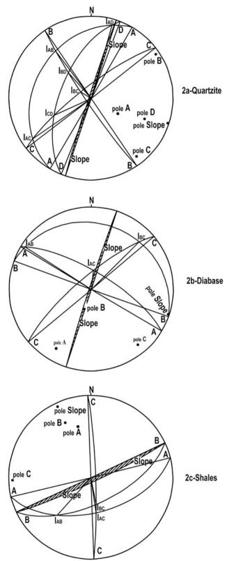
**Fig. 43.2** Stereographic projections on system cracks and slope. A-A-projection of the system cracks A; pole A-pole cracks of the system A;  $I_{AB}$ -projection of the intersection of the systems cracks A and B
