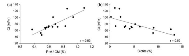
Fig. 12.4 The influence of the ratio of selected phenocrystals to groundmass on CI. P + A, represents the sum of the normalized areas of plagioclase and amphibole. GM represents the groundmass area (Ündül et al. 2013)
