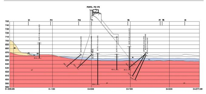
Fig. 106.5 Geological section along the dam spillway (river bed)
