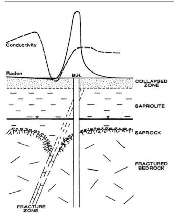
Fig. 57.1 Radon technique illustrated, after Wright (1992)
