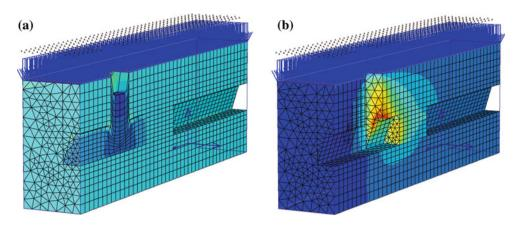
**Fig. 77.4** L = 5 m long dam after infilling. **a** Compaction due to 8 MPa pressure and **b** the axial deformation and displacement (the slurry material is not presented)
