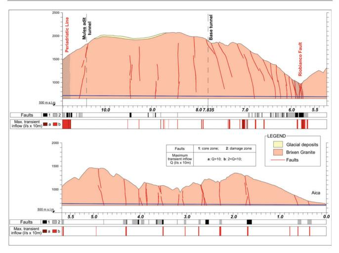
Fig. 177.2 Geological cross-section along the Aica Tunnel with the main water inflows occurred during the excavation
