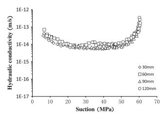
Fig. 94.3 Unsaturated hydraulic conductivity evolves with suction
