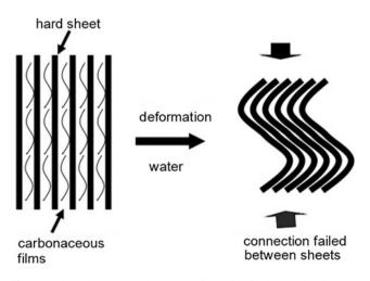
Fig. 3.5 Sketch showing the mechanism of softening and anisotropisation of slate
