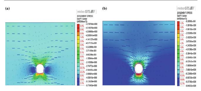
**Fig. 3.7** The differences in rock pressure between hard rock and soft rock. **a**  $E_m = 20$  GPa, v = 0.25,  $\varphi = 40^\circ$ , **c** = 12 MPa,  $\sigma_t = 6$  MPa; **b**  $E_m = 5$  GPa, v = 0.4,  $\varphi = 30^\circ$ , **c** = 1 MPa,  $\sigma_t = 0.5$  MPa
