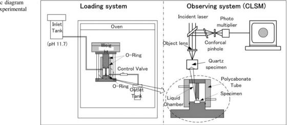
**Fig. 159.1** Schematic diagram of the flow-through experimental setup
