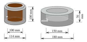
Fig. 39.5 Plastic mould section and base plate for testing a soil sample
