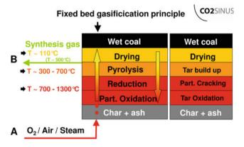
Fig. 193.2 Main UCG chemical processes and related tar behaviour during fixed bed gasification (Klebingat et al. 2013)
