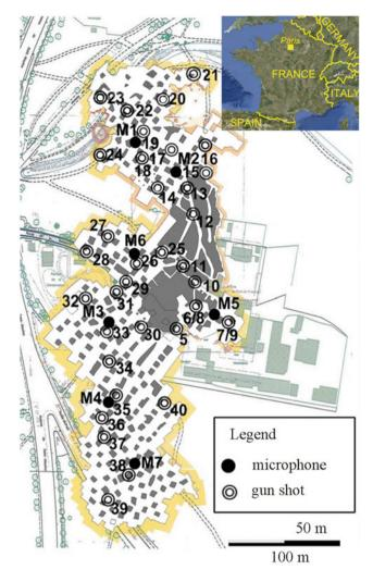
Fig. 123.1 The microphone array and the gun shot spatial distribution inside the quarry
