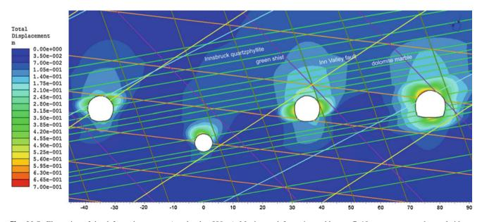
Fig. 80.5 Illustration of the deformation pattern (overburden 890 m). Maximum deformations add up to 7–10 cm at crown and tunnel sides
