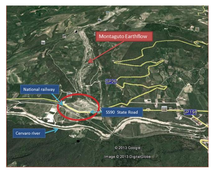
Fig. 54.1 Montaguto earthflow (Irpinia, Southern Italy). Note the State Road SS90 and the national railroad in the Cervaro river valley which were covered by the landslide debris
