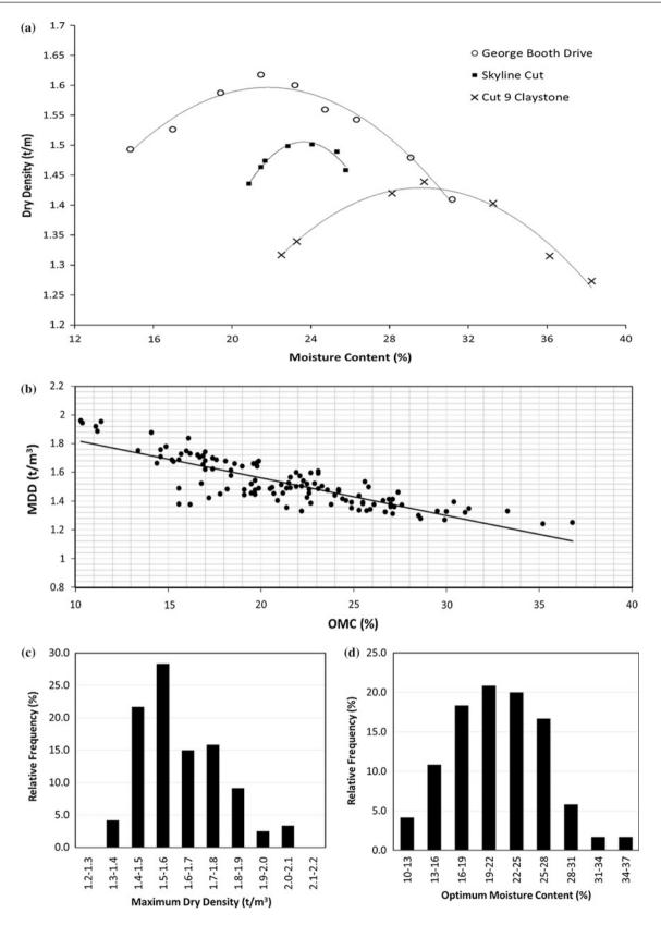
Fig. 45.3 Compaction data for NCM tuffs. a Standard proctor compaction curves for three typical NCM tuffs. b Maximum dry density versus optimum moisture content for 120 samples. c Relative frequency of MDD. d Relative frequency of OMC
