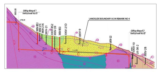
Fig. 65.2 Landslide along the axis of tunnel section after adjustments according to Remark No 4
