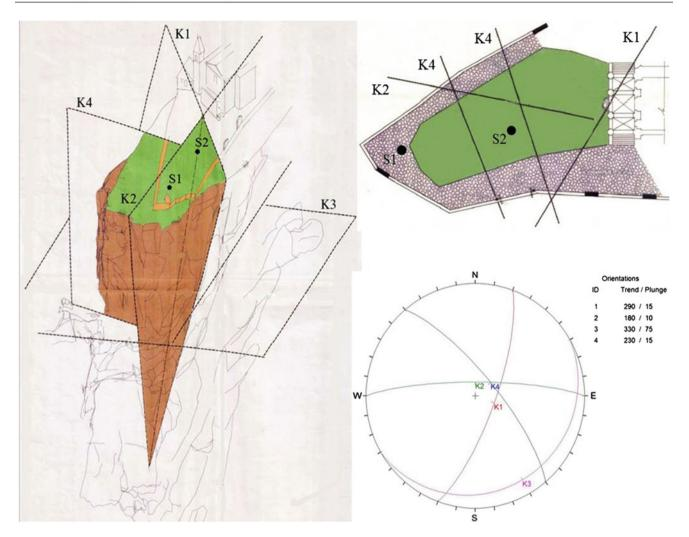
Fig. 125.1 Slope schematic structure: a assonometric and b plan views together with c surveyed joint sets after Lancellotta et al. 1991
