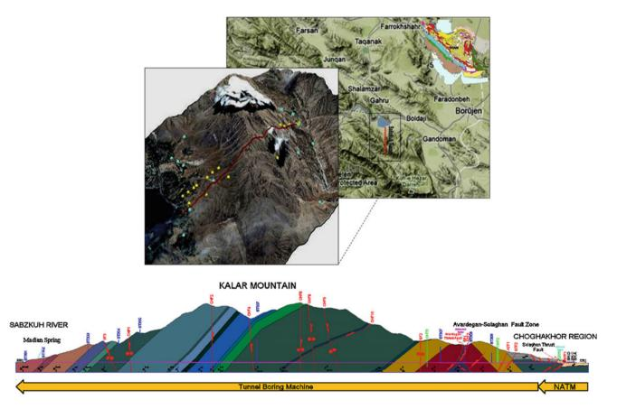
Fig. 107.1 Sabzkuh tunnel location (above) and longitudinal geological profile (below) (Taromi et al. 2013)
