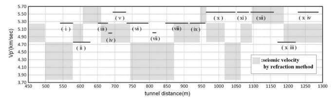
Fig. 187.6 Interval seismic velocity
