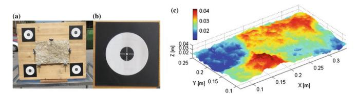
Fig. 150.1 a Experimental setup with joint sample and registration targets; b target zoom-in; and c triangulated surface from 1 mm ATOS grid (c)
