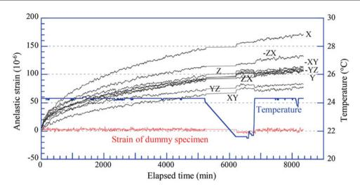
**Fig. 15.2** Anelastic strain curves (labels of X, Y, Z etc. showing its measurement direction) were measured in nine directions during approximate 1 week of a core sample taken from 1,469 m in WFSD-2 as an example of anelastic normal strain recovery raw data
