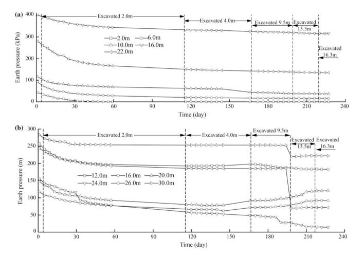
Fig. 30.7 Earth pressure variations with excavation and time
