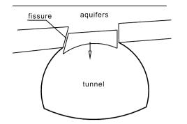
Fig. 78.4 Water inrush due to the instability of key block of rockmass
