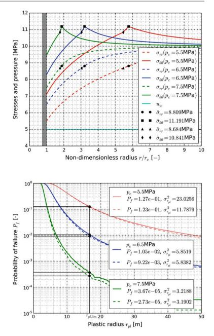
**Fig. 98.3** Probability of failure, i.e.  $P_f = P[r_{pl} > r_{pl,lim}]$ . The *solid line* corresponds to the uncorrelated case and the *dashed line* to the correlated case
