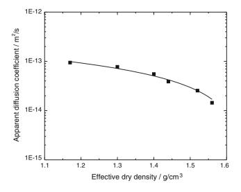
Fig. 89.4 Effect of effective dry density on the apparent diffusion
