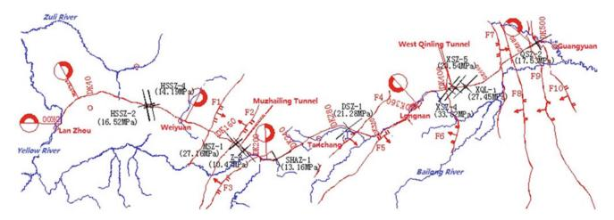
Fig. 3.2 Geological stresses measured along the railway line from China Railway First Survey and Design Inst
