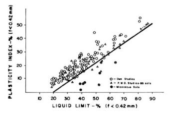
Fig. 33.1 Established variability in Atterberg limits tropical and lateritic soils from Ghana (Gidigasu 1974)
