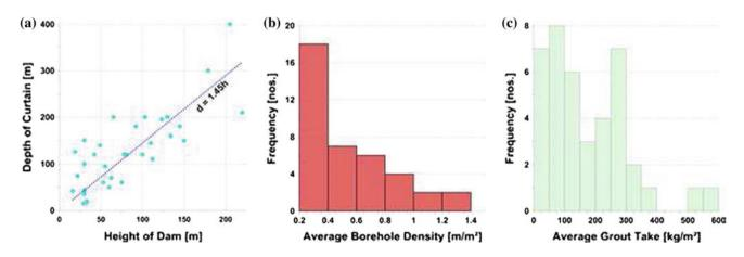
Fig. 138.3 Statistics of grout curtains in karst foundations of dams. a Depth of curtain versus height of dam. b Density of boreholes per square meter of curtain. c Grout absorption per square meter of curtain
