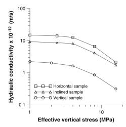
Fig. 87.3 Anisotropy of hydraulic conductivity of Boom Clay
