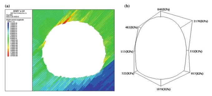
Fig. 3.8 Deformation Rock pressure of tunnel in layered rock. a Deformation of layered rock tunnel simulated by 3DEC; b Rock pressure measured at a tunnel of Lan-Yu railway
