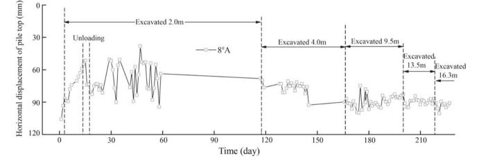
Fig. 30.5 Horizontal displacement-time curve of pile top with excavation and time
