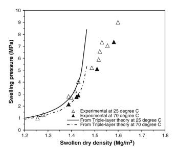
Fig. 96.2 Dry density versus experimental and theoretical swelling pressure plot
