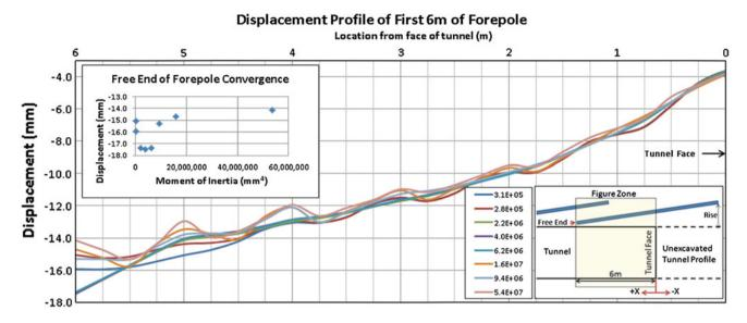
Fig. 157.2 Displacement profile of first 6 m of forepole from numerical analysis of varying size with 6 m of overhang. The plot illustrates the values of displacement of the free end of the forepole
