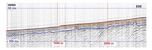
Fig. 69.4 Extract of a representative boomer seismic profile. *Blue line* corresponds to the top of bedrock and *orange line* to the top of the coarser unit and base of the finer deposit; brown reflector is the sea bed
