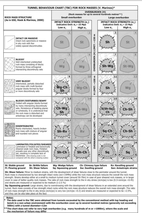
Fig. 155.1 Tunnel behaviour chart (TBC). Stress-controlled problematic behaviour that corresponds to weak rock masses is highlighted (Marinos 2012)
