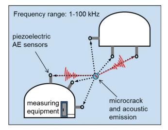
Fig. 99.1 Principle of acoustic emission measurements in mines
