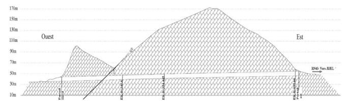
Fig. 38.6 Geotechnical and geological cup of the tunnel T1
