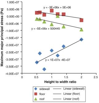
Fig. 79.3 Variation of maximum principal stress with aspect ratio of the arched-roof tunnel
