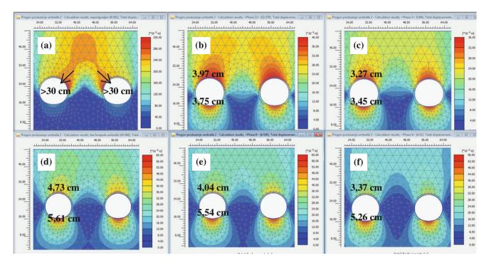
Fig. 55.4 Shadings of total displacements around tunnel excavations **a** Unsupported tunnel excavations,  $\beta = 0.83$ , **b** Tunnel excavation with forepoles according to design,  $\beta = 0.5$ , **c** Forepoles extended towards
