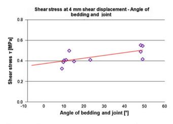
**Fig. 163.2** Shear stress at 4 mm shear displacement for samples in which the plane of the bedding encloses an angle with the plane of the natural joint (angle greater than  $0^{\circ}$  and less than  $50^{\circ}$ )
