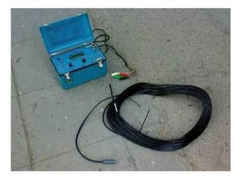
Fig. 49.2 Electrical thermometer tool
