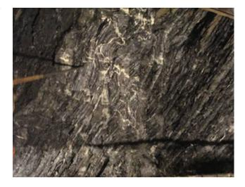
Fig. 3.3 Structure of the carbonaceous slate at Muzhailing tunnel
