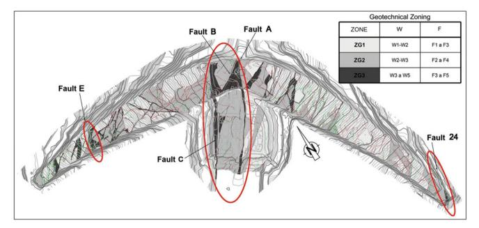
Fig. 10.4 Geoárea's simplified geological map and dam foundation geotechnical zoning. Fault zones referred in text are inside red ellipses
