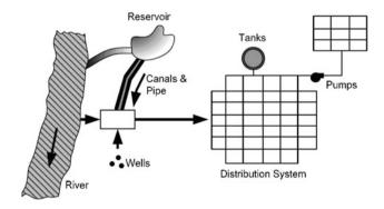
**Fig. 116.1** Elements and vulnerable points in a general water supply system (*source* Haestad et al. 2003)
