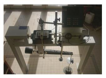
Fig. 145.4 Experimental shear test equipment
