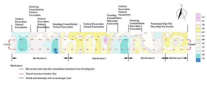
Fig. 105.9 Municipal road pavement longitudinal settlement isoline
