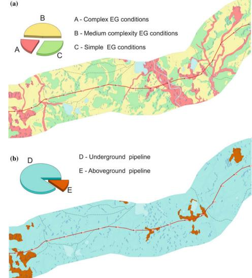
So, the first important step of the pipeline route investigations is the development of the GIS-based cartographic models of engineering geological conditions in the permafrost areas and consistent specification of those models and their characteristics.
