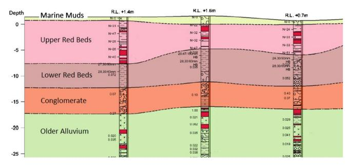
Fig. 50.2 Typical geological profile in Port Hedland Harbour
