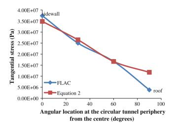
**Fig. 79.2** Tangential stress at the periphery of a circular tunnel in biaxial stress field (k = 0.63) from similar locations solved using closed form equation and FLAC
