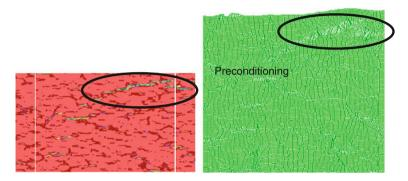
Fig. 76.4 Numerical model outputs of strain (*left*) and deformed grid (*right*, 5x vertical magnification) after 'excavation' showing potential face instability; model is 100 mm wide, face is at *top*
