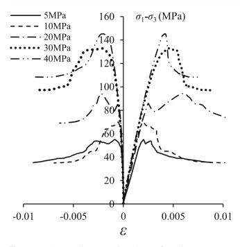
**Fig. 149.1** Stress-strain curves of specimens ( $\beta = 15^{\circ}$ )
