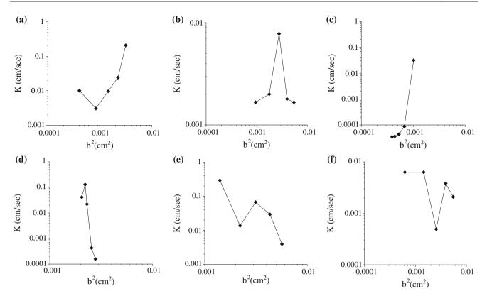
Fig. 160.4 Relationship between the C-permeability coefficients and the aperture square. a GRA, b GRB, c GRC, d GRD, e GRE, and f GRF
