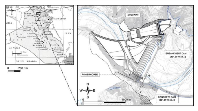
Fig. 148.1 Dam location map and general layout of works
