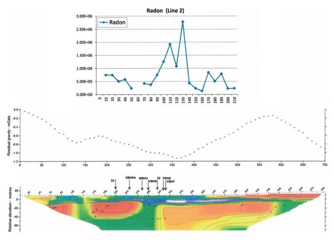
Fig. 57.2 Radon concentration profile (right bank)
