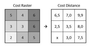
**Fig. 48.3** Example for "cost distance" calculation: lowest accumulated cost distance to move from start point x to upper-right cell = (3 + 6) \*SQRT(2)/2 + 3.5 = 9.9
