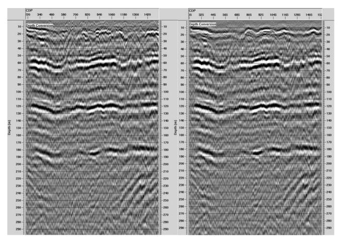
Fig. 189.4 Left result from seismic reflection processing, right seismic reflection combined with CMP-Refraction processed data
