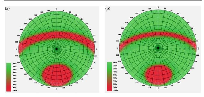
Fig. 3.6 Variation of modulus between original and disturbed state of the slate. **a** E = 10 GPa, v = 0.4, a = 1 m,  $\varphi = 20^{\circ}$ , c = 1 MPa; **b** E = 10 GPa, v = 0.4, a = 1 m,  $\varphi = 20^{\circ}$ , c = 0 MPa
