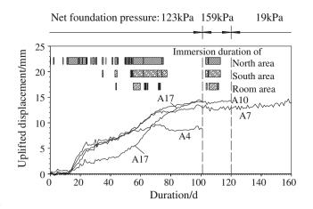
Fig. 37.5 Deformation curve of the most representation marks changing with time
