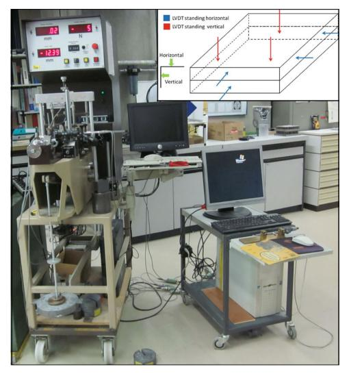
Fig. 163.1 Shear apparatus; position of the LVDTs in the right upper corner
