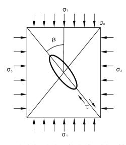
Fig. 78.1 Mechanical mechanism of hydraulic splitting of fissures
