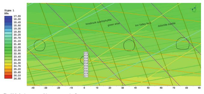
Fig. 80.2 In-situ stress conditions at cross section B
