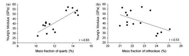
Fig. 12.2 The relation of Young's modulus with (a) the mass fraction quartz (b) the mass fraction orthoclase
