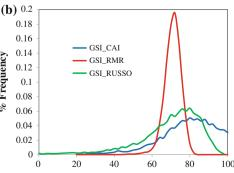
Fig. 152.5 Probabilistic estimates on the rock mass compressive strength (MPa) of a Kizilkaya ignimbrite and b New Zealand greywacke using GSI and RMi systems
