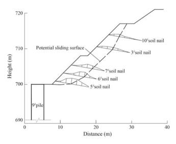
**Fig. 30.12** Location of the potential sliding surface in the slope above piles
