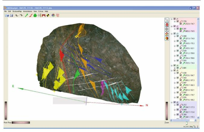
Fig. 166.1 3D documentation of a tunnel face with the structure map
