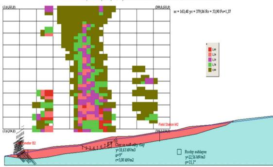
Slope stability analysis, Szymbark Landslide no 5 , Janbu method, after stabilization Fs=1.37
