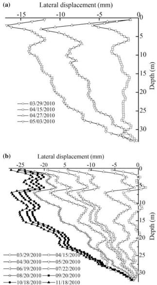
Fig. 29.11 Lateral displacement with time and depth. a Recorded by IT3. b Recorded by IT2
