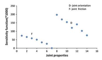
Fig. 79.8 Variation of sensitivity factor with joint dip angle and friction
