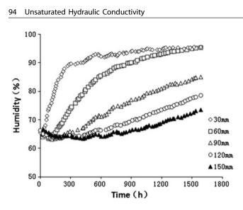
Fig. 94.2 Evolutions of humidity with time of the sand-GMZ01 bentonite mixture
