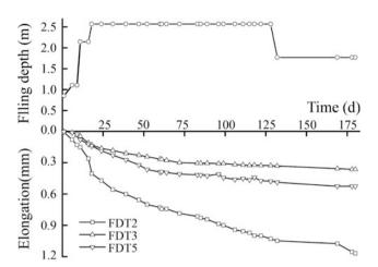
Fig. 29.10 Elongation variations with time and filling height
