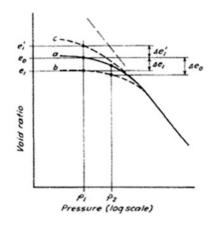
Fig. 1.1 Diagrams obtained in double oedometer tests
