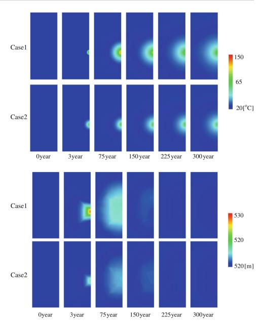
Fig. 86.5 Distribution of water head at specified times (2D)
