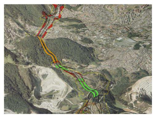
Fig. 195.1 Highway segment. Satellite image overlapped on the DTM. *Green* bridge or overpass; *orange* tunnel; *red* cut and fill; *yellow* right of way
