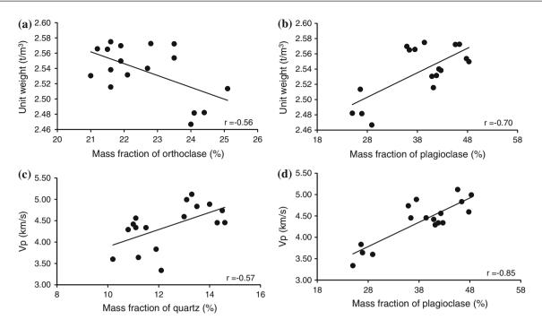
Fig. 12.1 The change of basic physical properties with mass fractions of different minerals. **a** Unit weight versus mass fraction of orthoclase. **b** Unit weight versus mass fraction of plagioclase. **c**  $V_p$  versus mass fraction of quartz. **d**  $V_p$  versus mass fraction of plagioclase
