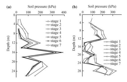
Fig. 30.6 Earth pressure variations with depth and excavation
