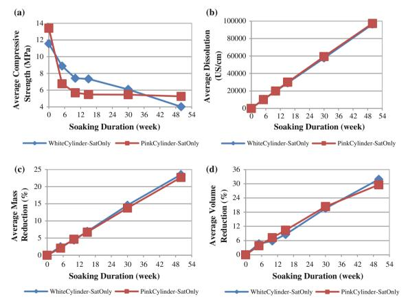
Fig. 139.1 Comparisons among short term loaded cylinders a is for compressive strength b is for dissolution c is for mass reduction and d is forvolume reduction. Each calculated values are the average of three tested cylinders
