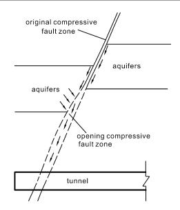
Fig. 78.5 Water inrush due to opening of compressive fault zone (Jiang et al. 2006)
