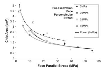
**Fig. 76.5** Chip area compared to face parallel stress for samples with different magnitudes of preconditioning stress and fabric oriented and  $0^{\circ}$  to the tunnel face; UCS  $\approx 100$  MPa
