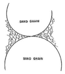
Fig. 1.5 Schematic arrangement of two sand grains with ring aggregation of clay
