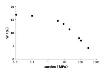
Fig. 94.1 SWRC of confined compacted sand-GMZ01 bentonite mixture
