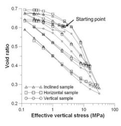
**Fig. 87.2** Void ratio versus effective vertical stress for oedometer test on three Boom Clay samples (vertical, horizontal, inclined 45°)
