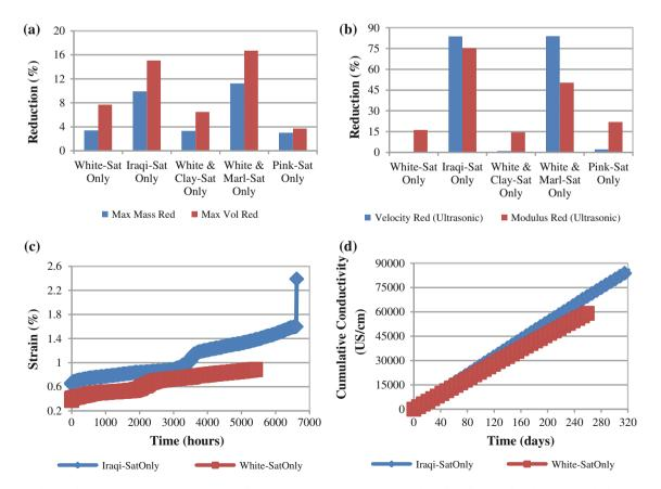
Fig. 139.5 Comparisons among long-term loaded cylinders. a Volume and mass reduction after 60 days. b Ultrasound velocity and modulus reduction after 60 days c, d are for 1 year loaded cylinders, Iraqi cylinder failed after 6,800 h as shown in part (c)
