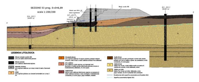
Fig. 51.2 Cross geological section in the damaged site
