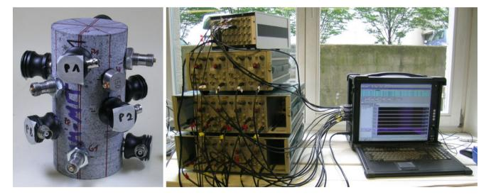
Fig. 81.1 Left 14 piezoelectric transducers attached to diorite sample from Nittenau (Bavarian Forest), Right pre-amplification and data acquisition system connected to the sample
