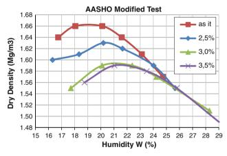
Fig. 112.3 Curve compaction of the AASHO mod. test performed on mixtures
