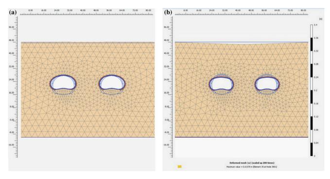
Fig. 55.3 Ground displacements in case of a MC model, b HSsmall model
