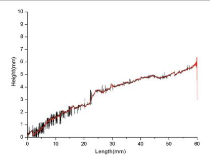
Fig. 160.2 Comparison of the measured roughness data of the left part of GRA (black) with the smoothed roughness data (red)
