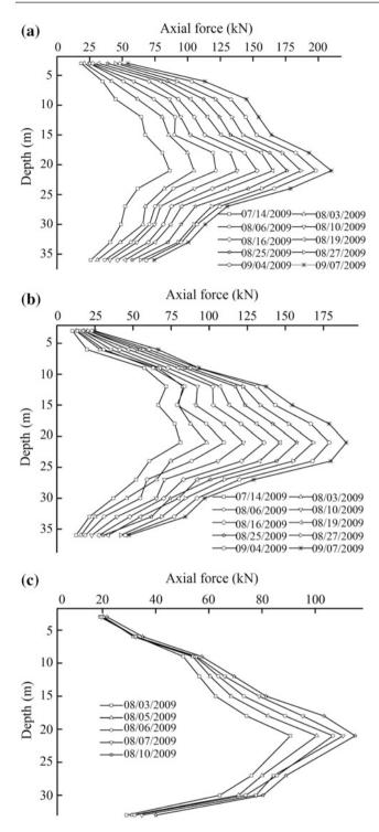
Fig. 29.8 Curves for the axial force as a function of depth. a Measured by TP2. b Measured by TP3. c Measured by TP4
