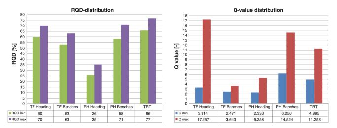
Fig. 100.3 Arithmetic mean of minimum and maximum values for RQD (*left*) and Q-values (*right*) for Transformer Cavern (*TF*), Powerhouse (*PH*) and Tailrace Tunnel (*TRT*)
