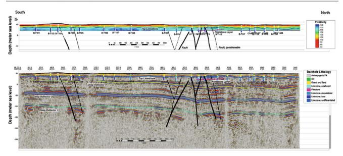
Fig. 189.6 Joint interpretation of geophysical data with integration of borehole results. *Top* refraction tomography, *bottom* combination of cmp refraction and reflection seismic
