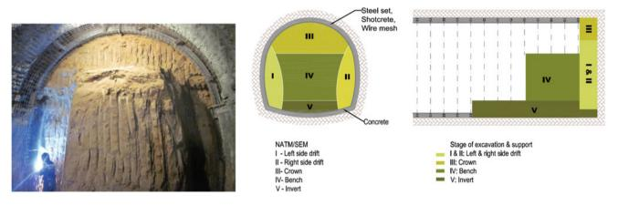
Fig. 107.6 Sequence of construction work
