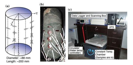
**Fig. 15.1 a** A schematic illustration of an ASR sample shows the X, Y, Z axes of a local coordinate system and the layout of the strain gauges glued on the surface of the cylindrical core sample. **b** A
