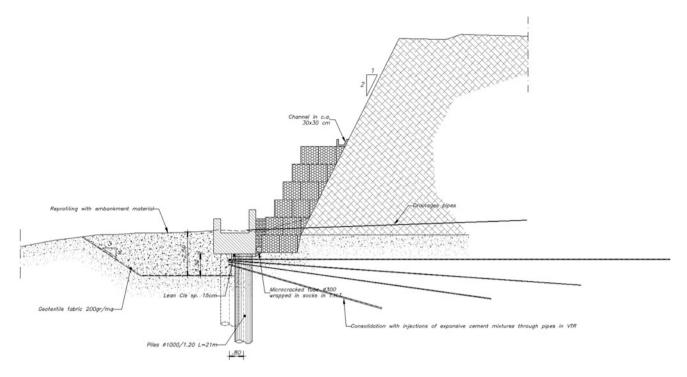
Fig. 51.3 Cross section showing the stabilization works
