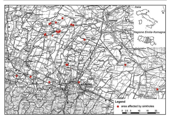
Fig. 73.1 Areas affected by sinkhole phenomena. Most of the areas are located in the Provinces of Modena and Bologna
