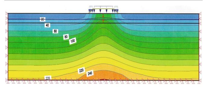
**Fig. 54.2** SIGMA/W solve analysis results with isolines of vertical H = 4 m; water table depth  $h_w = -5$  m; thickness of compressible
