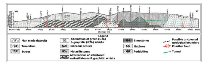
Fig. 71.1 Geological section of Pefka tunnel
