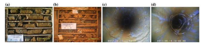
Fig. 146.4 Deformation and failure trends after mining. a Clay, b Sand, c overlaying rock (top) d overlaying rock (middle)
