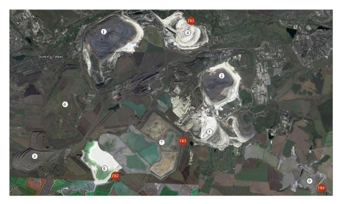
**Fig. 192.1** Space photo of the objects of the Staro-Oskolysky iron-ore distrikt: *1*-open Pit LGOK; *2*-open Pit SGOK; *3*, *4*-overburden dumps LGOK; *5*-overburden dumps SGOK; *6*-reclaiming hydraulic dump
