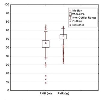
Fig. 8.2 Statistics RMR observed for the west side and east side of the tunnel
