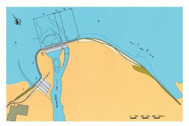
**Fig. 130.1** Types of dams in Itaipu hydroelectrical complex. *1—right* earth dam; 2—spillway; 3—*left* side dam (buttresses); 4—main dam (buttresses); 5—diversion structure (concrete); 6—*left* binding dam
