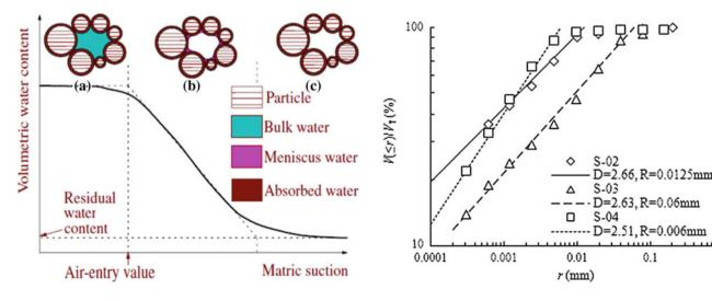
Fig. 92.1 Pore-water formation in soils
