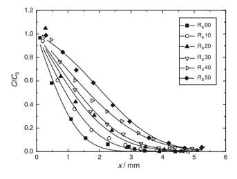
Fig. 89.3 Eu(III) concentration profiles and the fitting curves after 300d permeation
