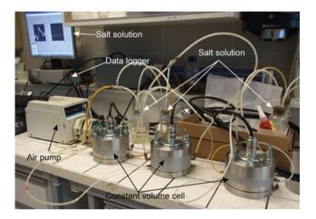
Fig. 85.3 Schematic diagram of the test setup adopted in the investigation
