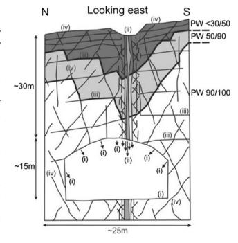
**Fig. 59.2** Conceptual engineering geological cross section of the cavern site, notation: (i) potential block fall, (ii) minor fault with potential for cave-in, (iii) sheeting joints, (iv) subvertical discontinuities, PW—partial weathering (GEO 1988)
