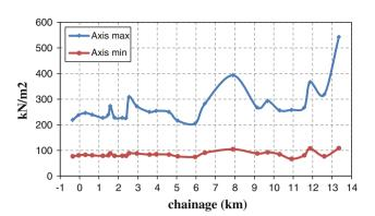
Fig. 53.1 Min and max support pressures at tunnel axis
