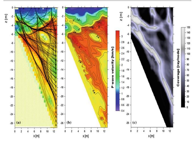
**Fig. 125.2** Result of the cross-hole seismic tomography: **a** acquisition scheme (S are seismic sources and R receivers) and traced rays after the inversion; **b** P wave seismic imaging and **c** ray coverage
