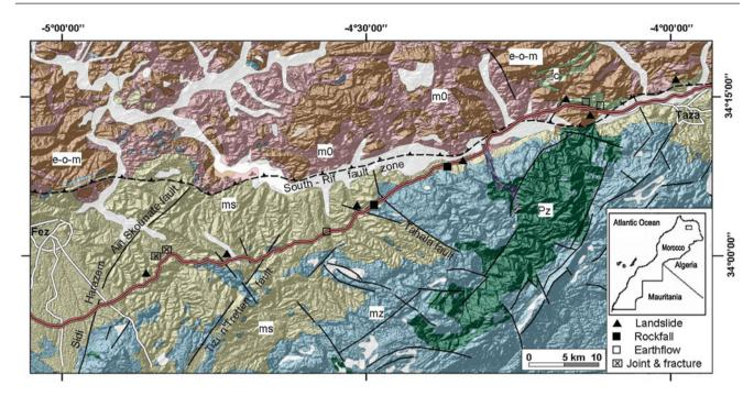
Fig. 17.1 Position of mass movements on the Fez-Taza highway on a geological and geomorphological background. Pz Palaeozoic, mz Mesozoic, c Cretaceous, e-o-m Eocene-Oligocene and Miocene, m0 Middle Miocene, ms Upper Miocene
