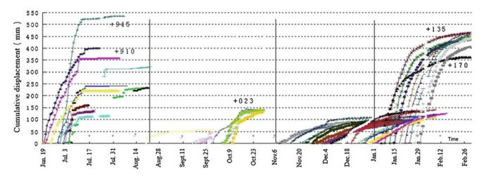
Fig. 3.4 Convergence deformation of the tunnel near Dazhangou shaft from China Railway First Survey and Design Inst
