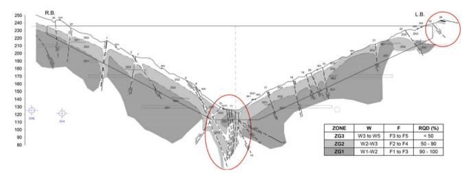
Fig. 10.3 EDP's design phase geological and geotechnical zoning—section through dam reference surface. Fault zones referred in text are inside *red ellipses*
