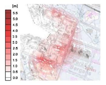
Fig. 52.1 Drawdown in groundwater levels in the Perkkaa area based on the numerical groundwater flow model
