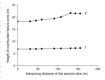
**Fig. 133.3** The height of overburden failure after mining the second slice by backfilling method. 1—caving zone; 2—water flow fractured zone
