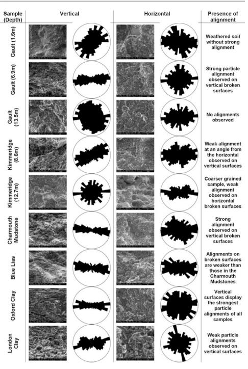
**Table 144.1** The average value of preferred particle orientation based on all images take from a single sample surface using magnifications between X600 and X1500
