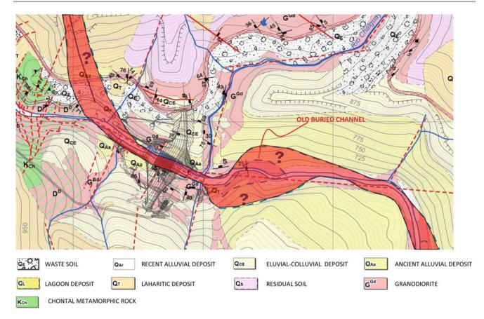
Fig. 106.3 Final layout, dam site with relevant geological characteristics
