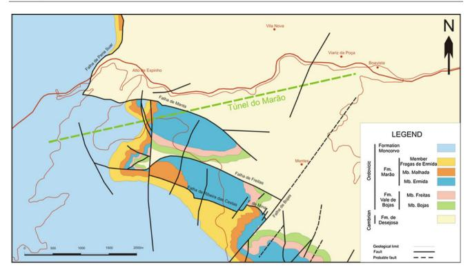
Fig. 8.1 Geological map of the tunnel area (Coke 2000)
