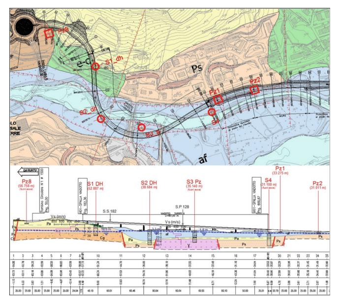
Fig. 112.2 Geological section along the tectonic structure of the Turriti Viaduct
