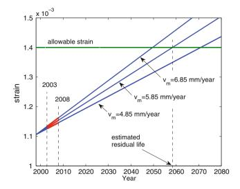
**Fig. 119.2** Maximum pipe strain due to temperature and pressure (year of pose 1998) along with strain due to PGD (velocities extrapolated from ENVISAT data measured in the period 2003–2008)
