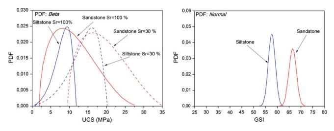
Fig. 148.2 Plots of the PDFs obtained from Monte Carlo simulations for UCS (*left*) and GSI (*right*)
