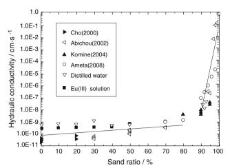
Fig. 89.2 Hydraulic conductivity vs. sand ratio
