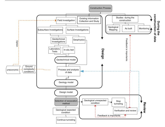
Fig. 107.2 Construction process algorithm (Taromi et al. 2013)
