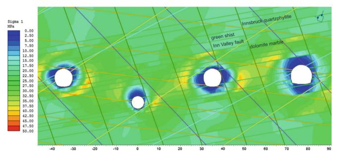
Fig. 80.4 Illustration of  $\sigma 1$  stresses. Minimum stresses are plotted in *dark colors*; maximum stresses are shown in *light colors*
