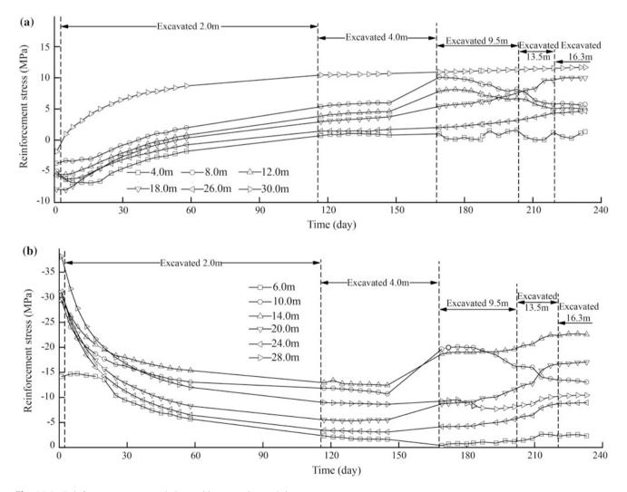
Fig. 30.9 Reinforcement stress variations with excavation and time
