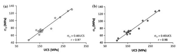
Fig. 12.3 The relation of crack initiation with UCS (a) crack initiation values obtained according to Brace et al. (1966) (b) crack initiation values obtained according to Lajtai (1974)
