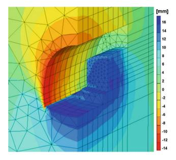
Fig. 107.8 Extreme displacements in tunnel face, Vertical displacements (Uy), Extreme Uy 13 mm (Crown)
