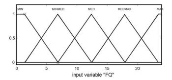
Fig. 185.3 Membership function of the fabric index of Q system, FQ
