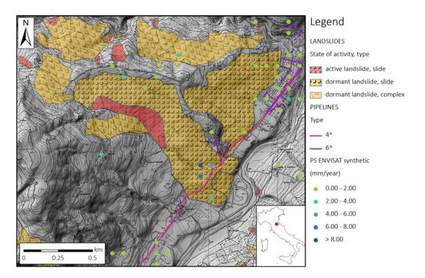
Fig. 119.1 Geographical location and sketch of landslide 35101, in Santa Sofia municipality (Forlì Province, northern Apennines, Italy) and pipelines affected by slope instability processes
