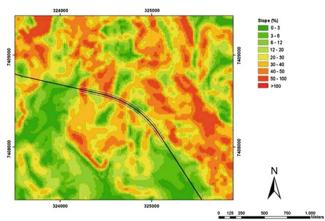
Fig. 195.3 Slope hill map for tunnel area. Note steep decline relief along the west entrance tunnel (in blue), favoring talus bodies occurrence
