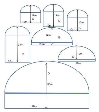
**Fig. 79.1** Arched-roof profile tunnel of different height to width (aspect) ratio investigated in this study. Aspect ratio of A 1.2; B 0.6; C 0.5; D 1.4; E 1.0; F 2.0; and G 0.75 (*Scale* 1 cm: 3 m)
