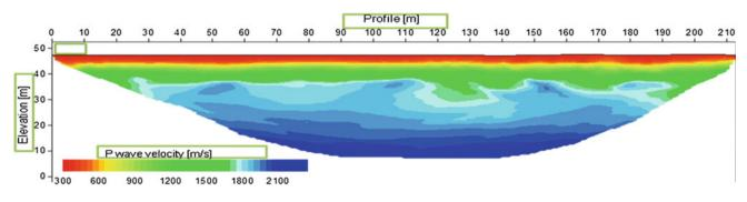
Fig. 189.5 Result of refraction tomography (example)
