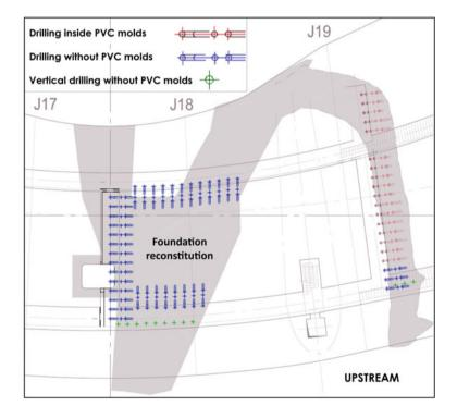
dam, in order to enable an adequate foundation treatment that consisted in fault gouge substitution by cement grout injection along these faults dip direction (Figs. 10.6 and 10.7). When dam concrete reached enough height, these localized treatments were followed by generalized cement grout injection (still ongoing) for foundation rock mass consolidation and waterproofing.
