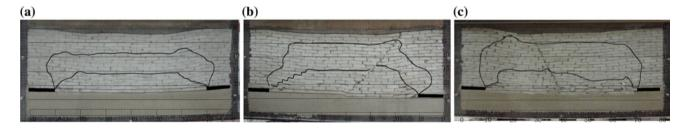
Fig. 146.2 Affect of faults to the deformation of dual structure. a No fault model. b One fault, dip =  $45^{\circ}$ , fall = 2 m. c One fault, dip =  $75^{\circ}$ , fall = 2 m
