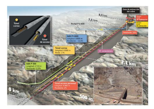
**Fig. 186.2** NML tunnel access system (by CTMSA)
