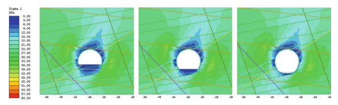
Fig. 80.3 Stress redistribution due to excavation of crown, side wall and invert applying conventional propulsion
