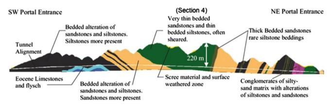
Fig. 7.1 Longitudinal topographic profile and idealized cross section for the Driskos tunnel (modified after Egnatia Odos S.A. 2003, Hoek and Marinos 2000)
