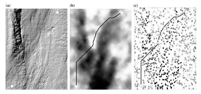
**Fig. 60.1** a Shaded relief seafloor rendering of the study area showing the two hypothetical pipeline termini used in this paper. Illumination is from the northwest. b Smoothed representation of the cost surface used in the real pipeline route selection along with the baseline least-cost
