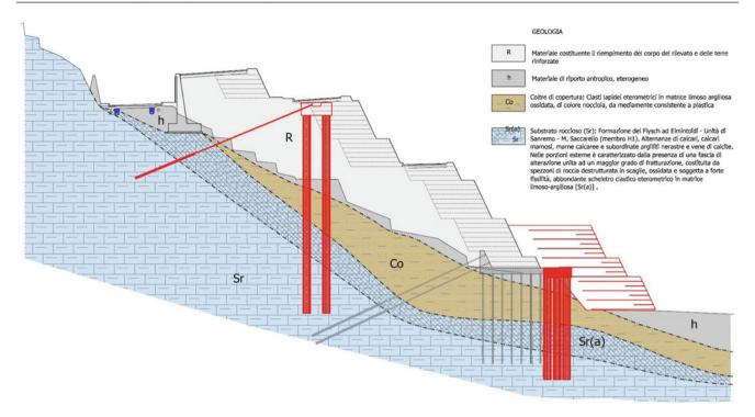
Fig. 51.5 Cross geological section, completed with the designed stabilization works
