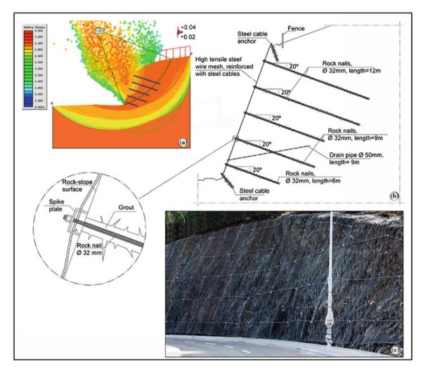
Fig. 147.3 Stabilisation solution design adopted for the studied rock slope. a example of slope stability analysis; b schematic cross-section with the main reinforcement features; c photo of the final stabilisation
