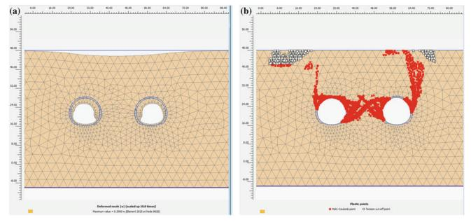
Fig. 55.2 a Deformed mesh showing ground surface settlement and deformations of tunnel contours, b development of plastic tension and shear zones
