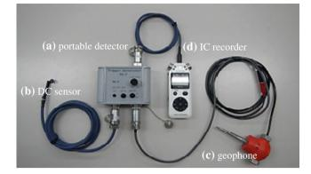
Fig. 187.1 Components of the tunnel face tester
