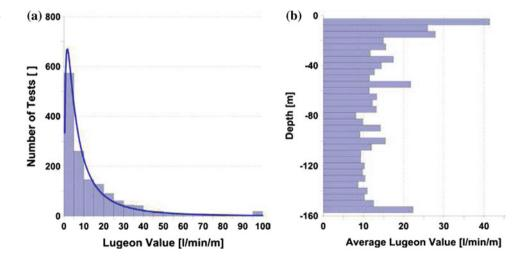
Fig. 138.1 Summary of Lugeon tests in primary holes of Ataturk grout curtain. a Histogram and fitted log-normal distribution. b Bar diagram Lugeon values against depth
