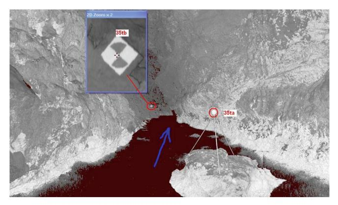
Fig. 121.2 Intensity image of a point cloud with a *flat black* and *white* target as well as a *sphere* on a *tripod*
