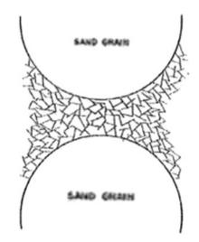
Fig. 1.7 Mud flow type of flocculated clay between two sand grains
