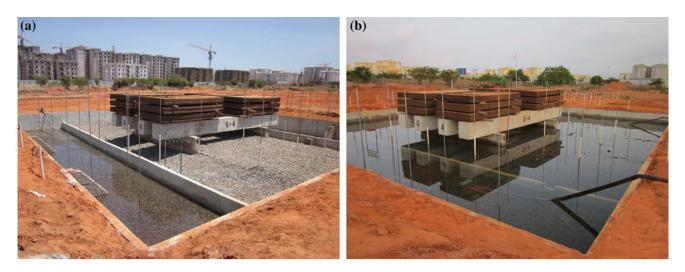
Fig. 37.2 Scene of immersion testing site. a Test pit with only the north area immersed. b Test pit with full water immersion
