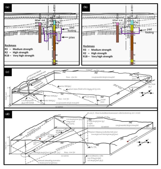
Fig. 67.1 a Original bored piled foundation design for BW11. b Revised pad footing design, c Detailed geological mapping of excavated foundation pad—eastbound. d Detailed geological mapping of excavated foundation pad—westbound
