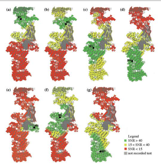
Fig. 123.3 Sensitivity map for: a microphone 1; b microphone 2; c microphone 3; d microphone 4; e microphone 5; f microphone 6; g microphone 7
