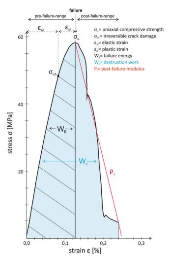
Fig. 82.1 Schematic stress-strain curve of a uniaxial compression test with the toughness defining parameters
