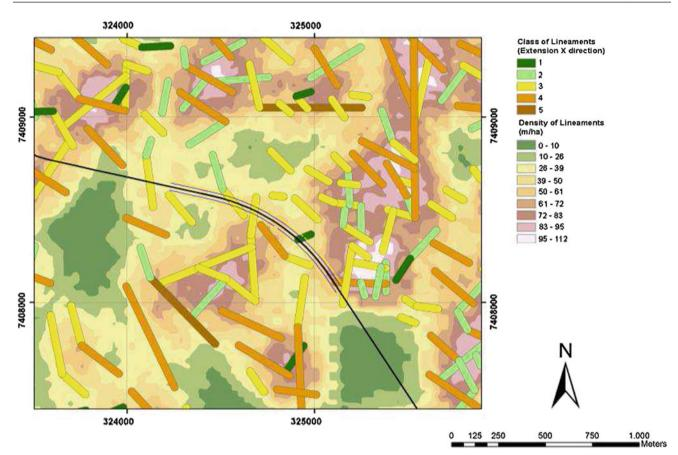
Fig. 195.2 Lineaments analysis in tunnel (in *Blue*) area construction
