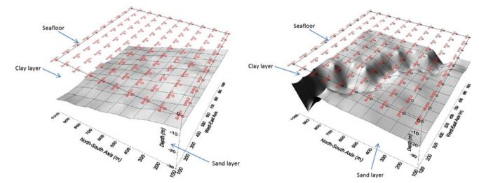
**Fig. 9.1** Scenario 1 a seabed defined by a clay layer and an underlying sand layer. The surface between the two layers is inclined towards the North. For this scenario 100 boreholes are given arranged in an equally spaced grid with separation distance 100 m, aligned to the North–South and East–West directions. *Scenario 2* a seabed defined by a clay layer
