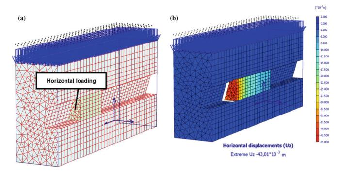
Fig. 77.2 a The modeled dam and b the deformation in axial direction
