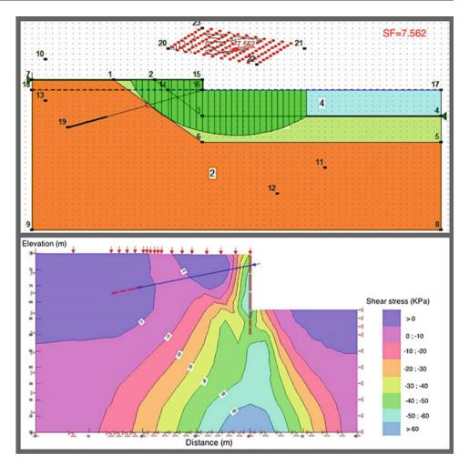
The active static impulses acting on the structure were defined by the Coulomb theory. Seismic impulses were calculated by Mononobe-Okabe method.
