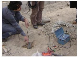
Fig. 49.3 Natural ground temperature measurements
