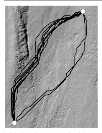
**Fig. 60.3** All 10 simulated routes superimposed on a shaded seafloor rendering. Actual pipeline routing projects use many realizations, perhaps 100 or more, to generate a stochastic cloud of equally probable pipeline routes and highlight areas most sensitive to input uncertainty
