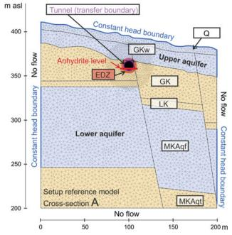
Fig. 75.2 Model setup for cross-section A. Q Quaternary, GKw weathered Gipskeuper, GK Gipskeuper, LK Lettenkeuper, MKAqf, Muschelkalk Aquifer, MKAqt Muschelkalk Aquitard
