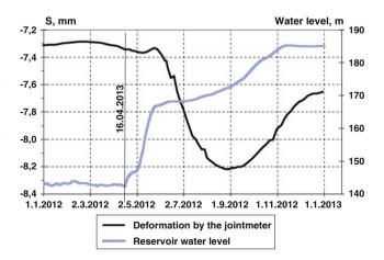
**Fig. 103.5** Deformations near-contact 2 m zones foundation in the section 18 during of the reservoir filling
