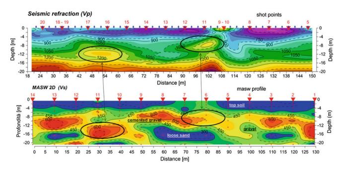
Fig. 190.1 Comparison between seismic refraction and MASW 2D section
