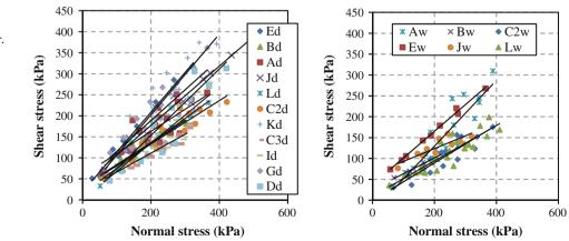
Fig. 145.5 Shear stress versus Normal stress in dry conditions and with joint immersed in water. "d" stands for dry and "w" for wet
