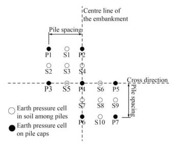
Fig. 29.3 Layout of the earth pressure cells
