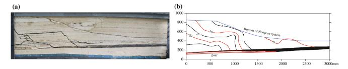
Fig. 146.3 Affect of inclination to the deformation of dual structure. a Deformation and failure. b Displacement offset of overlaying rock
