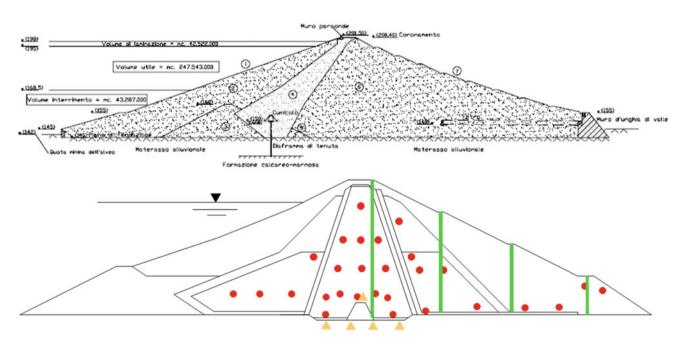
Fig. 131.1 Occhito's earth dam: (top) Geometry; (bottom) localization of sensors: piezometric cells (circles), pressure cells (triangles), inclinometers/assestimeters (vertical columns)
