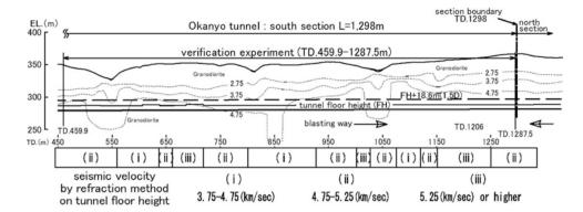
Fig. 187.4 Geological profile of Okanyo tunnel
