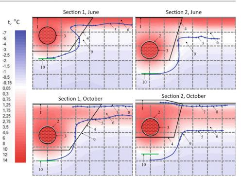
October in the third year of the pipeline's operation. Figure 70.2 demonstrates the agreement between calculated and measured results.
