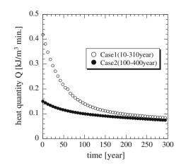
Fig. 86.3 Heat emission of HLW as the input in FEM
