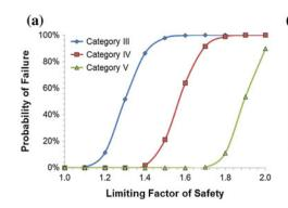
**Fig. 7.3** For Sect. 4.3, **a** liner performance for the shotcrete in the wall based on different limiting factor of safety values and **b** breakdown of support costs and expected costs of failure (monitoring, reprofiling,
