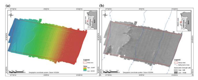
Fig. 69.2 Multibeam processed data: a MDT surface and b backscatter mosaic
