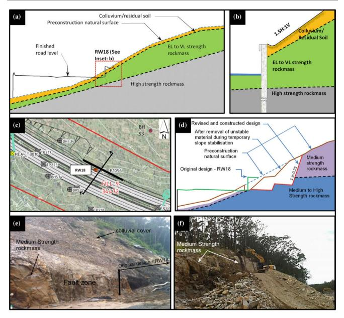
Fig. 67.2 a Original and revised design detail for RW18 and assumed geotechnical model. b Inset, with details of geotechnical model used for design at highest section of the wall c Location of geotechnical investigations used for original design. d Section detailing original
