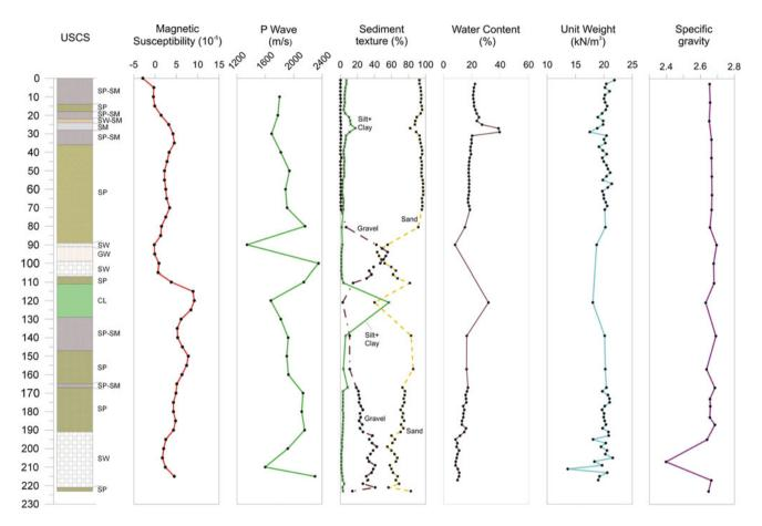
Fig. 69.5 Geotechnical proprieties of the marine deposits versus depth
