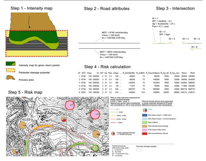
**Fig. 120.1** Explanation of the major steps in the risk calculation tool. *I* Import of the intensity map for a given process and return period; 2 Importation of the road axis lines and accompanying attributes; *3*
