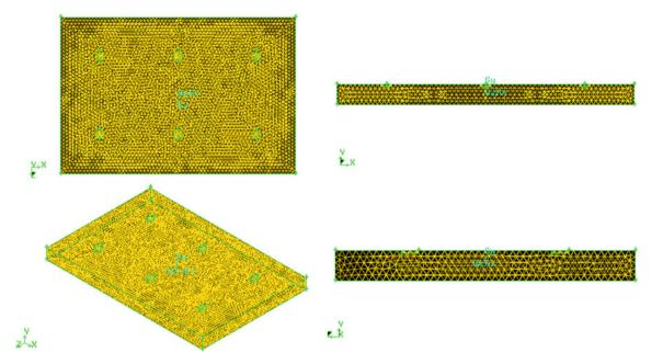
Fig. 132.5 The meshing of the pond of aeration of the treatment plant for Souk Ahras
