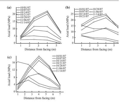
axial load along each nail shows in an parabola form with its maximum registered at the mid of nails.
