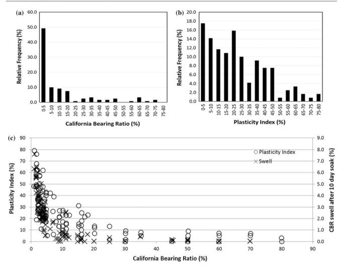
Fig. 45.4 California bearing ratio and plasticity index data. a Relative frequency of CBR. b Relative frequency of PI. c Correlation between 10 day soaked CBR and plasticity index and swell
