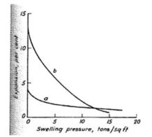
Fig. 1.8 Typical results obtained in swelling tests
