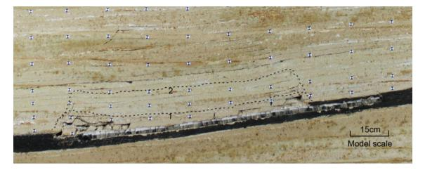
Fig. 133.2 After mining the second slice. 1-caving zone; 2-water flow fractured zone
