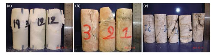
Fig. 139.3 The failed cylinders after short-term loading: a The white/Bantycock gypsum. b The pink/Bantycock gypsum. c The Iraqi gypsum
