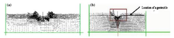
Fig. 68.4 a Field of displacement vectors of particles with no reinforcement geotextiles (the maximum displacement % 13.26 mm. b With geotextile reinforcement at a depth of 25 mm (max % 11.9 mm), Bhandari and Han (2010)
