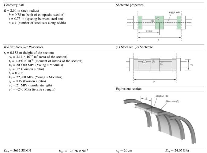
Table 107.2 Input data for the analysis of a semi-circular liner comprised of shotcrete and steel sets according to the 'equivalent section' approach (Carranza-Torres and Diederichs 2000)
