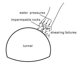
Fig. 78.3 Water inrush due to shearing failure of impermeable rock wall
