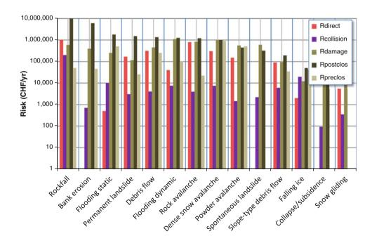
**Fig. 120.3** Risk details per hazard and damage type for all analysed road sections
