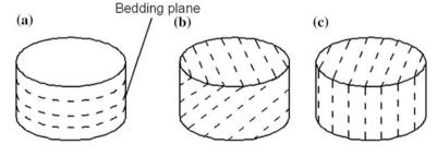
**Fig. 87.1** Three types specimens used in oedometer test: **a** vertical sample ( $\alpha = 0^\circ$ ); **b** inclined sample ( $\alpha = 45^\circ$ ); **c** horizontal sample ( $\alpha = 90^\circ$ ).  $\alpha$ : angle between the axis of specimen and the axis perpendicular to the bedding plane
