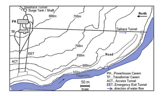
**Fig. 100.1** Layout of the Powerhouse Complex at Dagachhu Project
