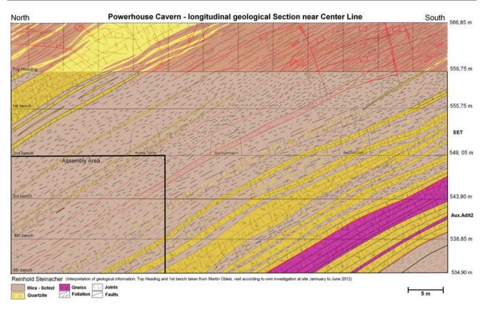
Fig. 100.2 Longitudinal section at center line of Powerhouse Cavern (brown Mica-Schist; yellow Quartzite; magenta Gneiss; red faults)
