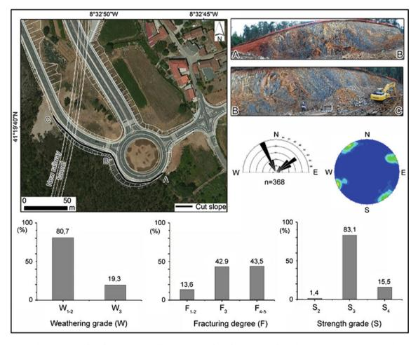
Fig. 147.2 Location and view of Trofa cut slope (ABC), (*upper part* of the figure); main discontinuity sets and other geotechnical parameters (*lower part* of the figure)
