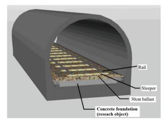
Fig. 115.1 Sketch map of the cross section of the tunnel structure under the rails (*unit* cm)
