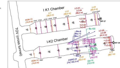
**Fig. 166.2** The in situ measurement and monitoring system in the first two chambers at Bátaapáti NRWR
