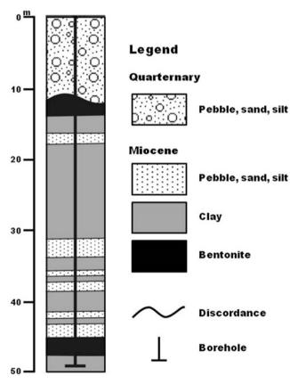
Fig. 153.4 Typical engineering geological borehole at the studied area
