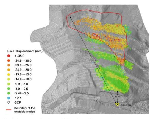
Fig. 126.2 GBInSAR displacement map projected over a digital elevation model
