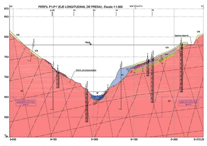
Fig. 106.4 Geological profile along the dam axis
