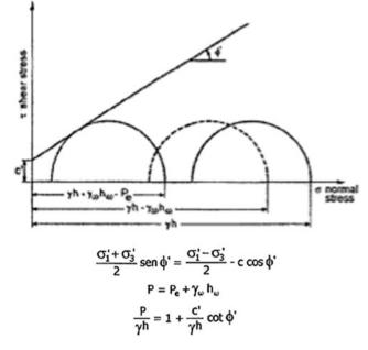
Fig. 1.14 Assumed mechanism for hydraulic fracture
