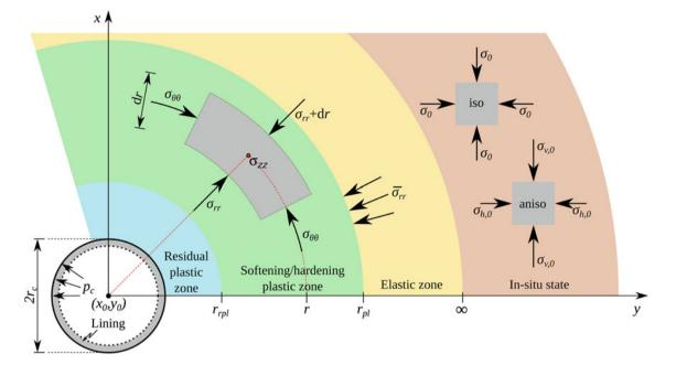
**Fig. 98.1** Schematic description of stresses around a cavity opening where  $r_c$  is the excavated cavity radius,  $p_c$  is the cavity pressure (i.e. acting on the liner),  $r_{pl}$  is the plastic radius,  $r_{rpl}$  is the residual plastic
