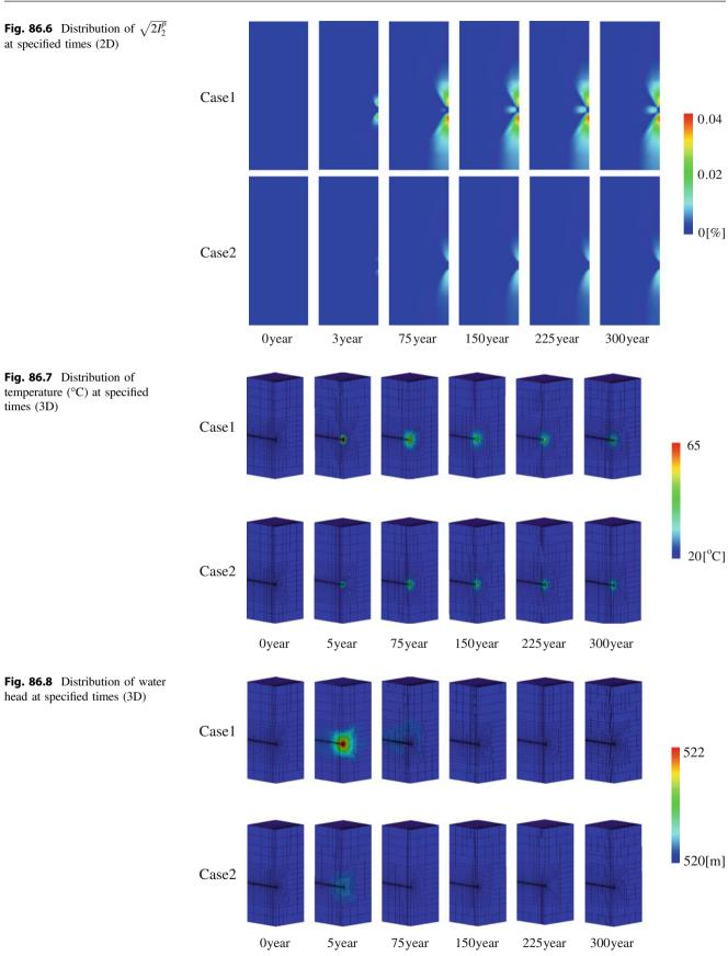
Fig. 86.7 Distribution of temperature (°C) at specified times (3D)
