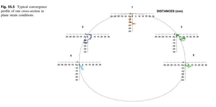
If HSsmall model is used for convergence predictions (accounting for arching effect and deformations of the tunnel face) values of approx. 1 cm are obtained.
