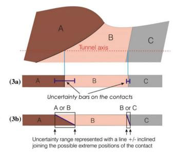
**Fig. 183.3** Representation 3. Geological longitudinal profile and strips showing the location of contact points for the elevation of the project, with an uncertainty bar (type 3a) or oblique line (type 3b)
