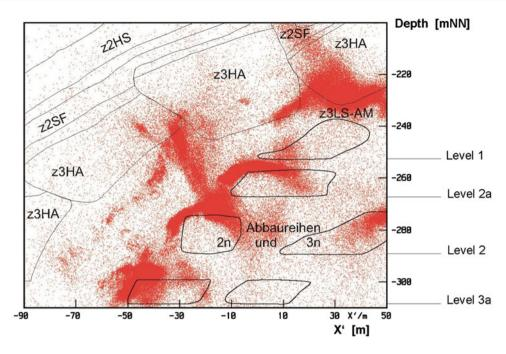
Fig. 99.2 Locations of AE events in the year 2010 in a vertical cross section in the central area of the salt mine with a sketch of the excavation chambers and the geological units
