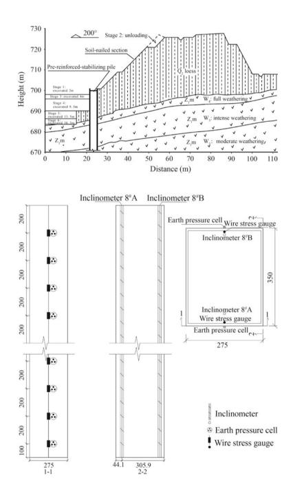
**Fig. 30.2** Layout of monitoring instruments along pile 8<sup>#</sup> (unit: cm)
