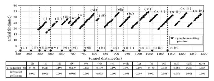
Fig. 187.5 Travel time curve in Okanyo tunnel
