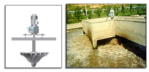
Fig. 132.3 The system of aeration of surface
