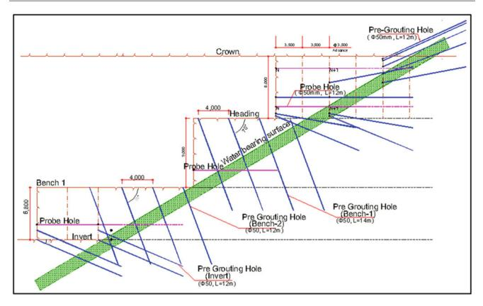
Fig. 167.1 Scheme for grouting
