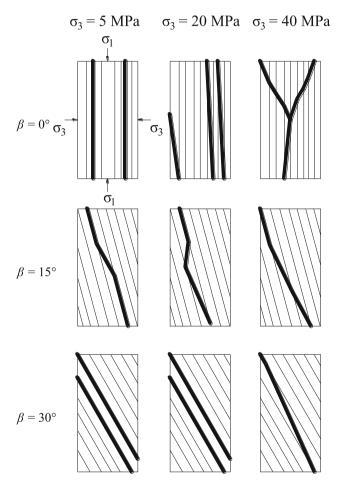
Fig. 149.5 Typical failure patterns
