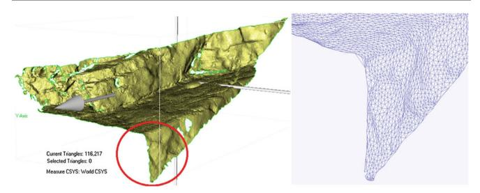
Fig. 121.3 Section of the meshed point cloud, 8 m long (left); view of the area inside the red circle, triangle with 2 cm edge length (right)
