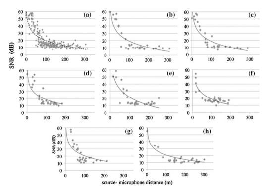
Fig. 123.2 SNR, in dB, as a function of the source-microphone distance for: **a** all the microphones; **b** microphone 1; **c** microphone 2;
