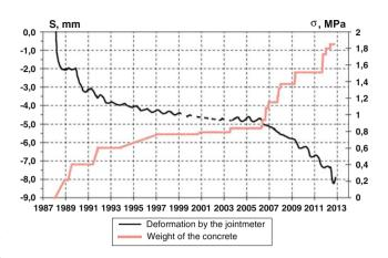
Fig. 103.3 Deformations near-contact 2 m zones foundation in the section 18 during the construction of the dam
