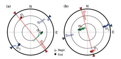
**Fig. 15.3** Stereo projections (lower hemisphere) of orientations of three-dimensional principal stresses which are same as those of the principal anelastic strains from ASR measurements with respect to the true north coordinate system. The stress orientations were calculated from anelastic strain values at a certain range of elapsed times, thus the
