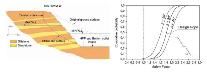
Fig. 148.3 Left Slope geology and typical slip surface analyzed; Right probability of failure obtained by varying the overall slope angles
