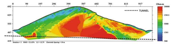
Fig. 184.3 Geophysics results and the tunnel axis indicated by the dashed line
