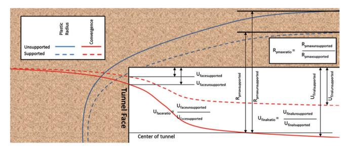
Fig. 157.4 Illustration of the change of the plastic radius, final convergence of the tunnel and displacement of the tunnel face due to support, where U displacement and R radius)
