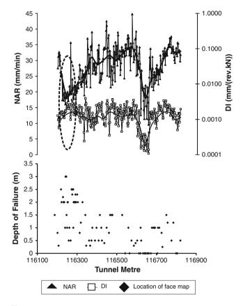
**Fig. 76.2** Comparison between TBM NAR and DI (*above*) and depth of face failure (*below*) along a section of deep tunnel. High depth of failure occurs at low NAR and high DI locations (*dashed ellipse*), and no face failure occurs at low NAR and low DI
