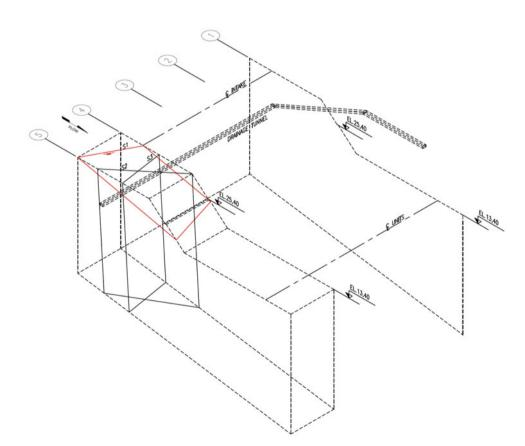
**Fig. 111.2** Isometric model of intake excavation—spatial arrangement of the major sets of joints
