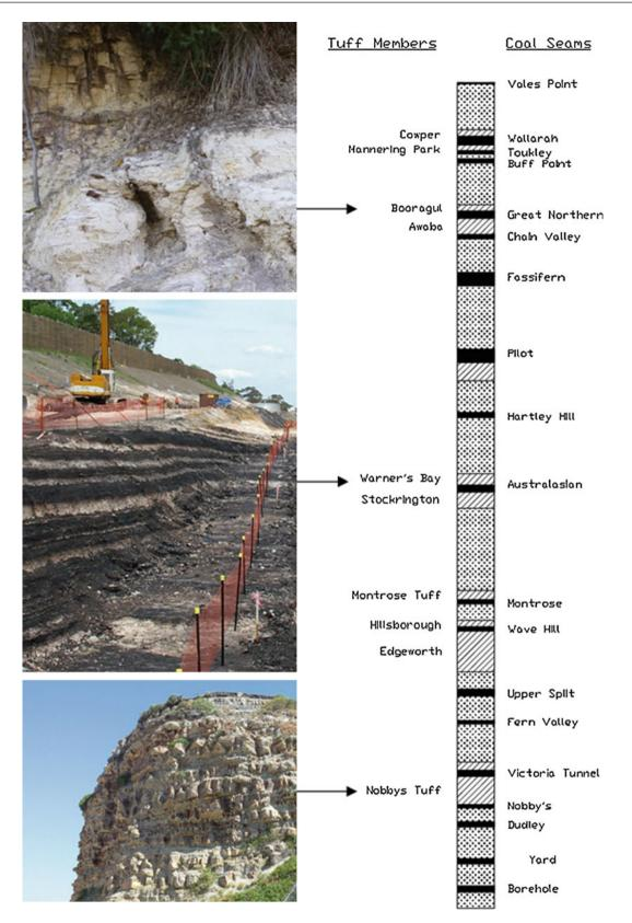
Fig. 45.1 Stratigraphic column of the Newcastle coal measures showing named and unnamed tuff units, with photographs of some well-known units
