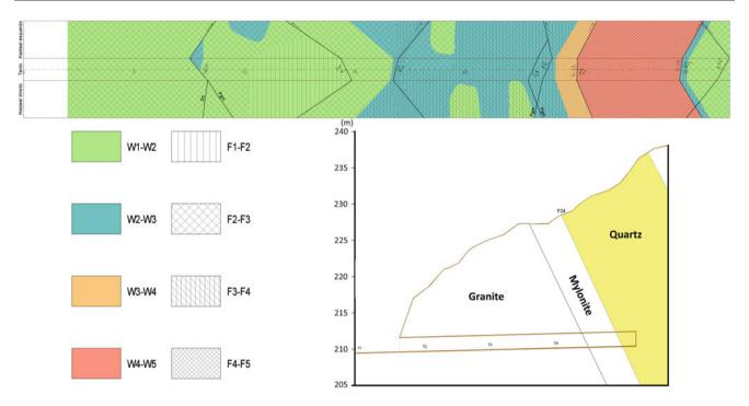
Fig. 10.2 Ceiling and wall mapping of GE1 gallery (walls folded to horizontal). W4-W5 zone corresponds to fault's mylonitic footwall, below quartz vein
