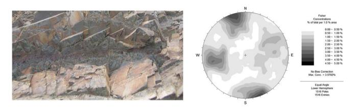
Fig. 152.2 A view of the New Zealand greywacke and discontinuity orientations
