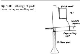
When the zone of seasonal variations in moisture extends to a depth greater than that below which drilled piers have been designed, attempts to form the bells of such piers may be unsuccessful because the clay in the zone of moisture changes likely to be highly slicken sided and successive caving of the blocks between slickensides might occur.
