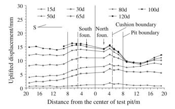
Fig. 37.6 Settlement section connected by A series of deformation marks at different times
