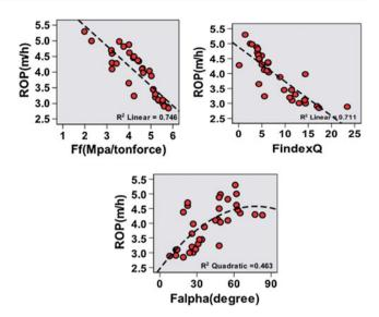
Fig. 185.2 Relationship between measured ROP and three input parameters
