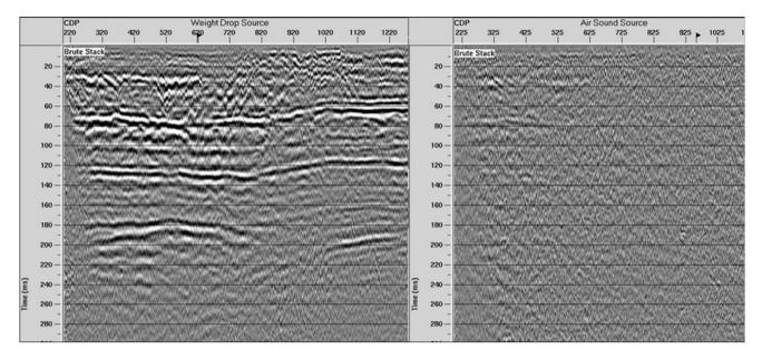
Fig. 189.3 Comparison of Brute stacks for weight drop (left) and air sound source (right)
