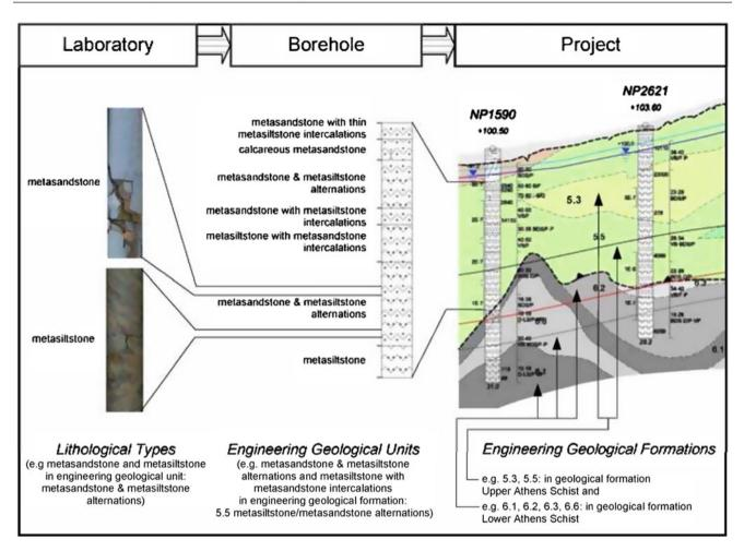
**Fig. 151.2** Explanatory graph showing the "flow" of the approach from the laboratory sample scale to the project site scale, namely from the lithological type to the engineering geological formation. In reality, two processes that feed one another, are simultaneously undertaken;
