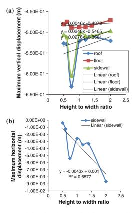
Fig. 79.5 a Variation of maximum vertical displacement with varied tunnel aspect ratio. b Variation of maximum horizontal displacement with varied tunnel aspect ratio
