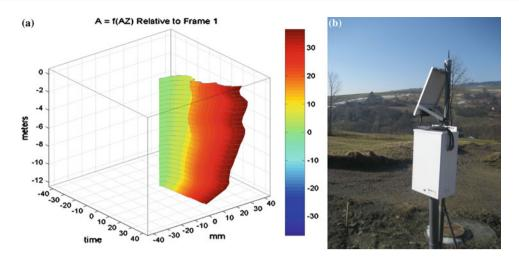
Fig. 32.6 On-line monitoring. a 3D displacements plot. b Field Station
