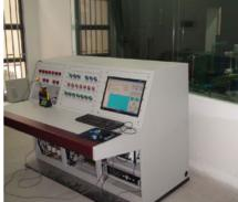
Fig. 5. Pump performance tester
