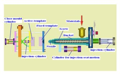
**Fig. 1.** Injection moulding
