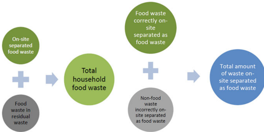
Fig. 4.13 Graphical illustration of the terms on-site sorting ratio ( left ) and ratio of mis-sorted waste ( right )
