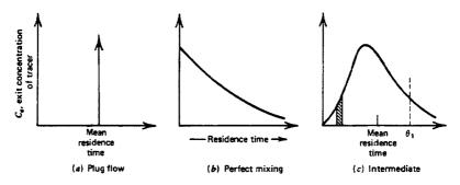
Figure 12.2-1 Exit concentrations of tracer observed in vessel when input stream is tagged at time zero.
