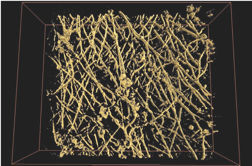
Figure 2. Reconstructed volume from the above tilt series (by weighted back projection using iMod) visualized with an isosurface, using amira.
