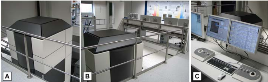
Figure 1. The Titan Krios as installed at the MPI of Biochemistry (A and B). The control unit of the microscope is seated on the 'bridge' (B upper right and C).
