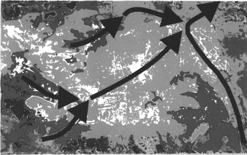
Figure 2.11 In Stuttgart, air is encouraged to flow from cool hill-top areas, shown dark, down into the town. Stuttgart suffers from temperature inversions and becomes very hot in summer.
