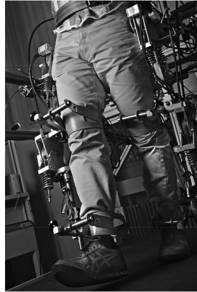
Figure 28.1 Recently developed gait robots, such as the LOwer extremity Powered ExoSkeleton (LOPES), sense the forces generated by the subject and adjust their imposed forces accordingly. In this way, training programs can be administered taking optimal account of the individual functional capacities of the subject. Figure provided courtesy of G. van Ouwerkerk (CTW, University of Twente) and the manufacturers (Dept. of Biomechanical Engineering, Faculty of Engineering Technology, University of Twente, The Netherlands)
