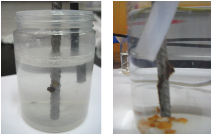
Figure 3. Left: a pit with the oxides of dark color growing upwards of a bar. Right: other stage of the process in which the oxides which have fallen down can be appreciated in the bottom of the flask
