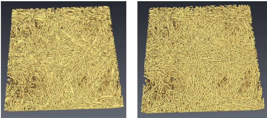
Fig. 4.16 Cut-out ( 830 \times 830 \times 200 \mu\text{m}^3 ) of experimental data gained by synchrotron tomography (left) and extracted fibers (right)
