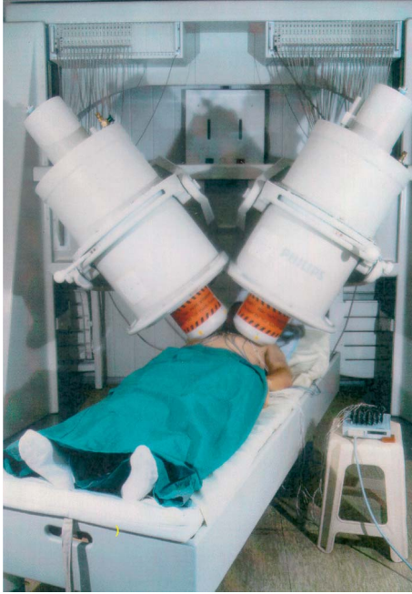
Fig. 2.28. 62-channel twin dewar biomagnetometer during MCG-recording (Philips).
