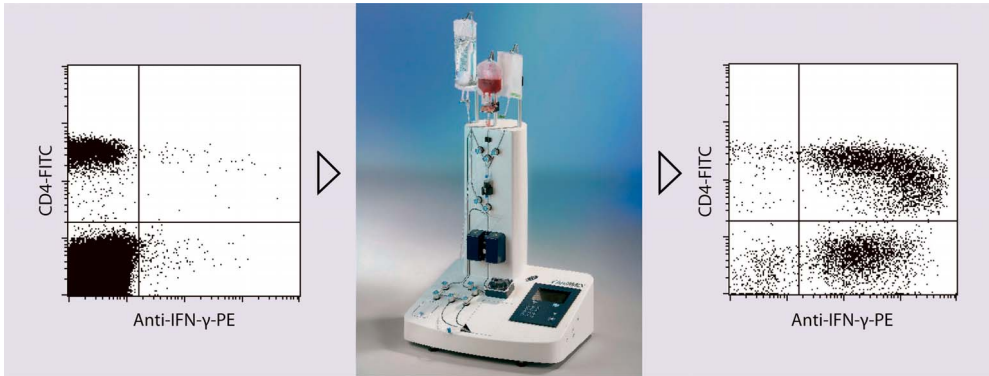
Fig. 4.47. Typical enrichment of IFN- \gamma producing CMV-specific T cells using the CCS. IFN- \gamma producing CMV-specific T cells are enriched from <0.3% to >90% of the T cell population after CliniMACS enrichment.
