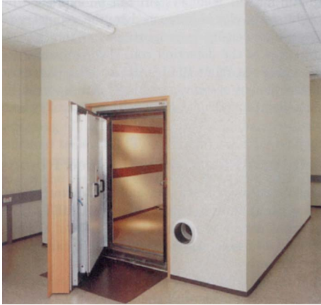
Fig. 2.6. Vacuumschmelze Hanau: magnetically shielded room AK 3b.
