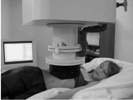
Fig. 4.29. SQUID biosusceptometer at the Children's Hospital and Research Center at Oakland. An 11-year-old girl, covered by the waterbag, lies under the dewar tail before a 10-s vertical scan.
