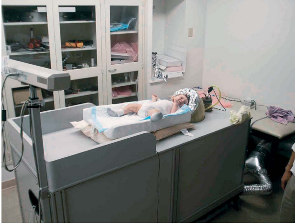
Fig. 2.27. BabySQUID® Neonatal Biomagnetometer. The magnetometer is located in the infant bed. Electronics and data acquisition system is located in the cart. The rectangular device at the end of the infant bed is the projector for the optical positioning system.
