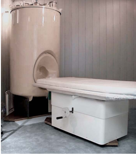
Fig. 2.25. Argos 500 with patient bed inside a magnetically shielded room.
