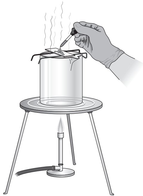
FIG. 5.2. Slide on beaker. Heat acid-fast slide over a beaker of boiling water.
