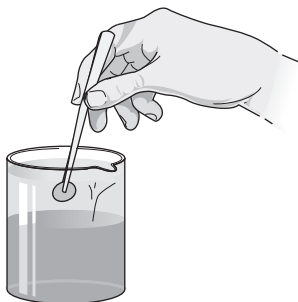
FIG. 10.8. Get sample of disinfectant or antiseptic by placing paper disk in the test solution.
