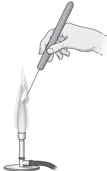
FIG. 2.1a. Heating the loop.
