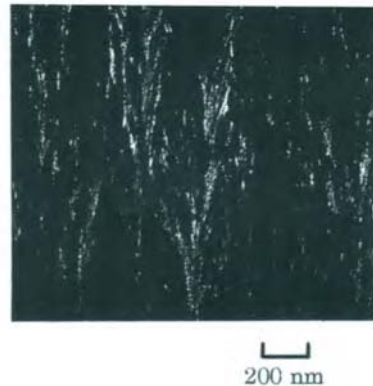
Fig.4. The cross sectional dark field TEM micro-graphs of 520 °C annealed FeSiAlTiON films.
