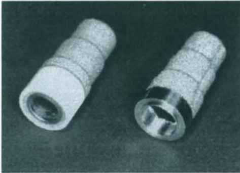
Fig. 4. Dental implants made from a Ti/Al 2 O 3 composite (left) and from titanium (right).
