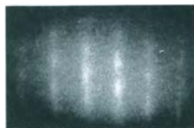
Figure 4. RHEED pattern of the BaTiO 3 thin film deposited at V_a=+50 V and V_b=-100 V. The pattern was observed from [100] azimuth.
