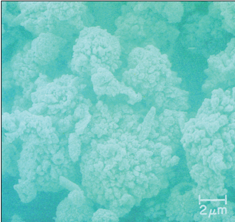
PLATE 11 Gold-loaded zinc precipitate (ex solution) (SEM photo courtesy of FMC Gold Co.; Merrill-Crowe precipitate provided by Coeur d'Alene Mines).
