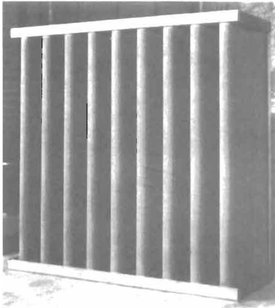
Figure 12-53. Corrugated bed-type activated charcoal air-purification cell. This unit contains 35 lb of 50-min. activated coconut-shell charcoal and handles 1,000 cfm of air with a pressure drop of 0.25 in. of water. Courtesy of Barnebey & Sutcliffe Corp.
