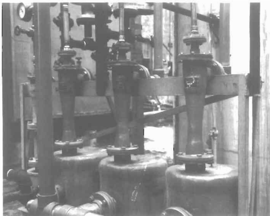
Figure 6-20. Jet Venturi scrubber system for removing HCl vapor from exhaust gas. Croll-Reynolds Co., Inc.
