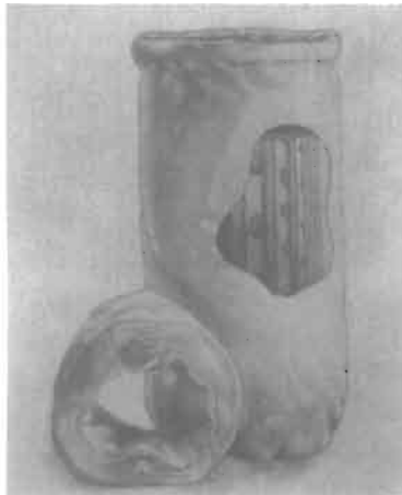
Figure 3-24. Proprietary polypropylene bag filter for amine service. Each bag has multiple layers with internal bypasses which provide 32 ft 2 of filtration surface per bag. Courtesy 3M Filter Products
