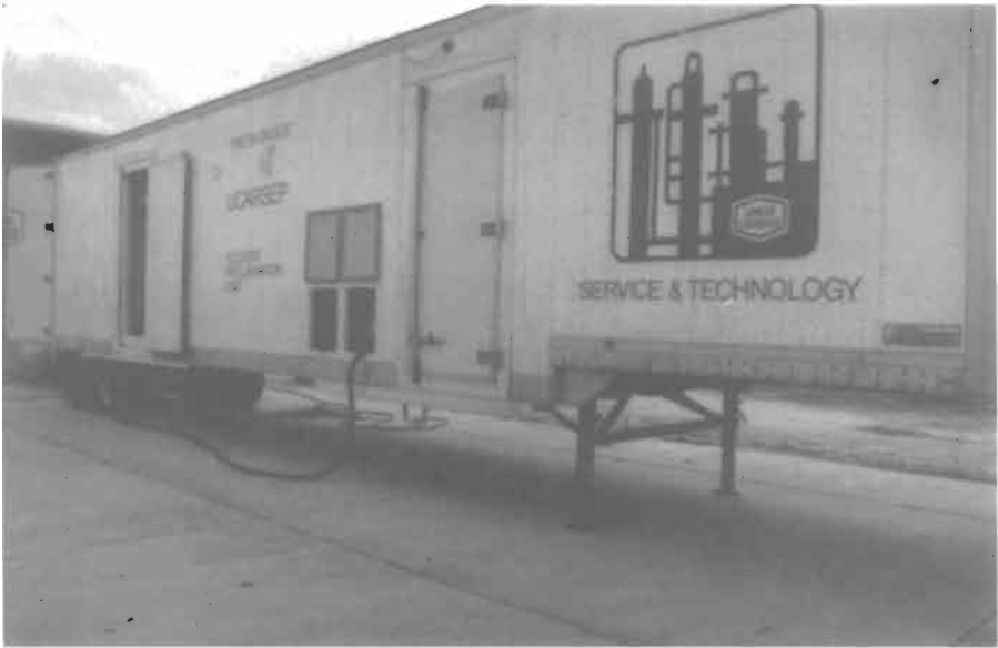
Figure 3-35a. Mobile electro dialysis unit for amine reclaiming. Courtesy Union Carbide Corporation
