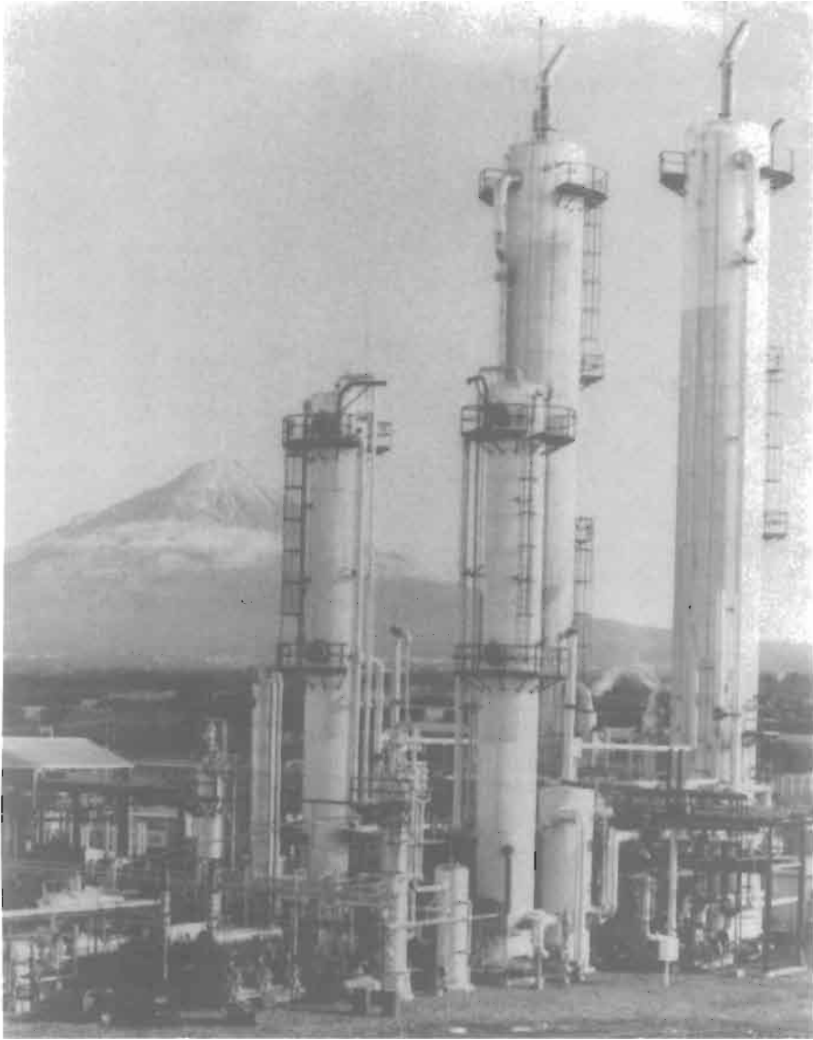
Figure 5-2. Two Benfield trains for natural gas purification. Courtesy of UOP and Natural Gas Corporation of New Zealand
