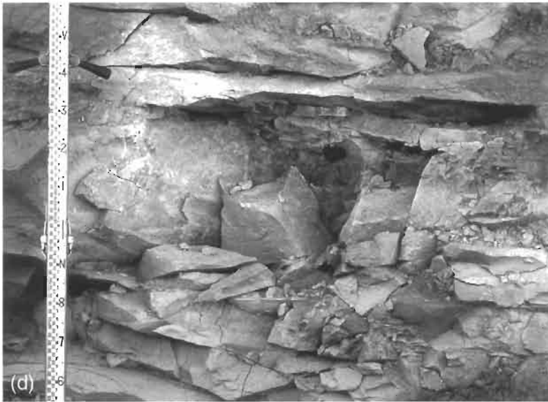
Figure 8.1 (left and above) Examples of fractured rock masses. (a) Folded rock mass in Crete illustrating that the mechanical behaviour will be a function of both the intact rock and the fracture geometry. (b) Fractured limestone rock mass, relatively unaffected during excavation by tunnel boring machine. (c) Jointed granitic rock mass with joints dilated by bulk blasting. (d) Heavily jointed chalk rock mass, with joint dilation resulting from weathering.
