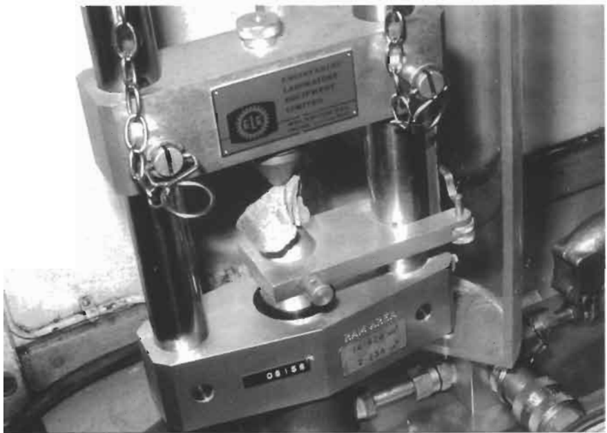
Figure 11.5 The Schmidt hammer and point load test equipment.
