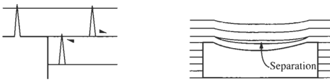
Figure 19.21 Composite instability around excavations in stratified rock.
