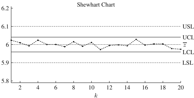
Figure 1.4 Upper and lower specification limit as well as upper and lower control limits and set point value for key variable z .
