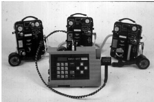
Figure 3.3.9 Organic vapour analyser. (Courtesy Quantitech Ltd)
