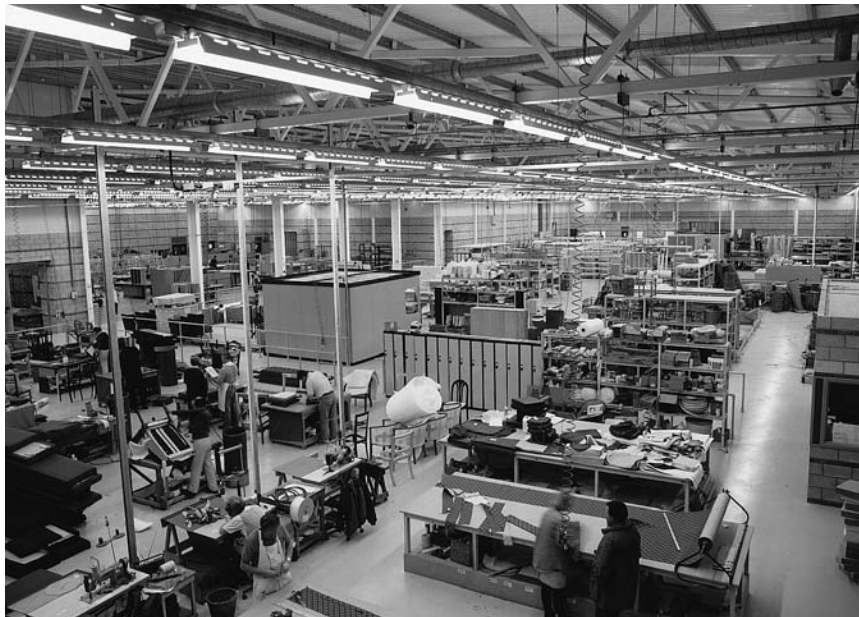
Figure 3.7.1 Factory lighting where fine work is carried out and colour rendering is important, making use of reflector luminaires with tubular fluorescent lamps. (Courtesy Lighting Industry Federation)
