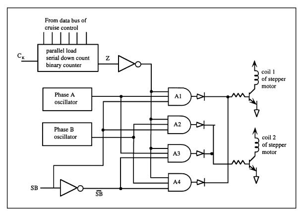
This signal is, in effect, a signed number (i.e., a positive or negative numerical value). A sign bit indicates the direction of the throttle movement (advance or retard). The numerical value determines the amount of advance or retard.
