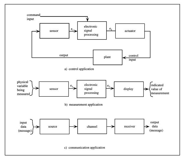
block are identified. In electronic systems, these input and output variables are electrical signals, except for the system input and system output. One benefit of this approach is that the subsystem operation can be described by functional relationships between input and output. There is no need to describe the operation of individual transistors and components within the blocks.
