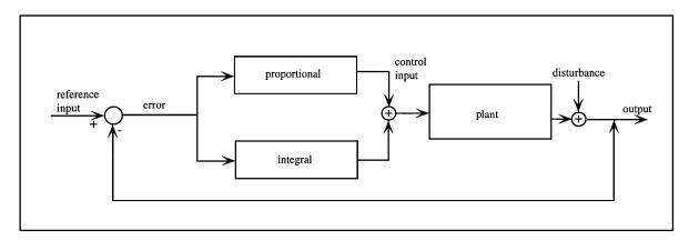
digital controllers. The relative ease and low cost of implementing PI controllers is part of the motivation for the trend toward electronic control in automotive systems.
