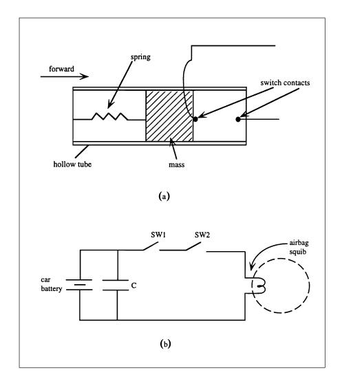
Under normal driving conditions the acceleration at the accelerometer locations is less than 1 g. However, during a collision at a sufficiently high speed the signal increases rapidly. Signal processing can be employed to enhance the collision signature in relation to the normal driving signal. Such signal processing must be carefully designed to minimize time delay of the output relative to the collision deceleration signal.
