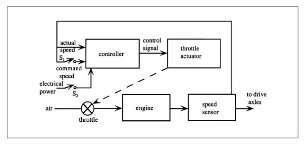
Whenever the actual speed is less than the desired speed the throttle opening is increased by the actuator, which increases vehicle speed until the error is zero, at which point the throttle opening remains fixed until either a disturbance occurs or the driver calls for a new desired speed.
