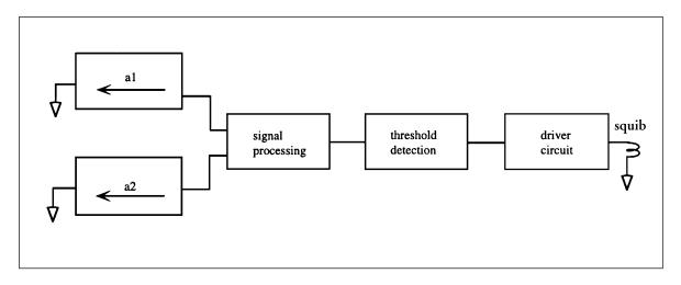
threshold, the driver circuit sends a current of sufficient strength to activate the squib and inflate the airbag.
