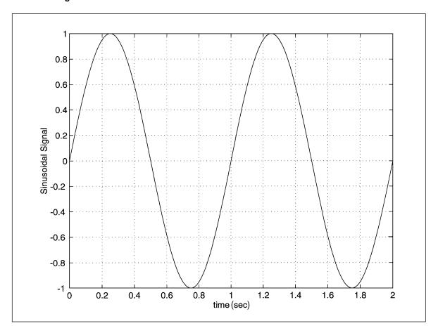
The input fluctuates through a complete cycle beginning at zero, increasing positively to a maximum, then moving symmetrically negatively back to zero in T seconds. It then repeats periodically in intervals of T seconds. The frequency f of the input is the number of cycles in one second, or
