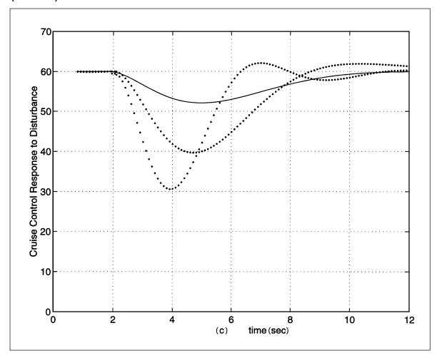
When a new speed is requested, the time required for the vehicle to reach that speed is affected by the control system's damping coefficient.
