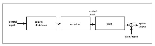
The control electronics generates the electrical signal for the actuator in response to the control input and in accordance with the desired relationship between the control input and the system output. The operation of the plant is directly regulated by the actuator (which might simply be an electric motor). The system output may also be affected by external disturbances that are not an inherent part of the plant but are the result of the operating environment.
