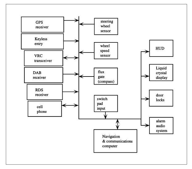
include a switch pad for data/command input, a compass, antilock braking, and wheel steering sensors. This system is to have an active matrix liquid crystal display (AMLCD) as well as a heads up display (HUD).
