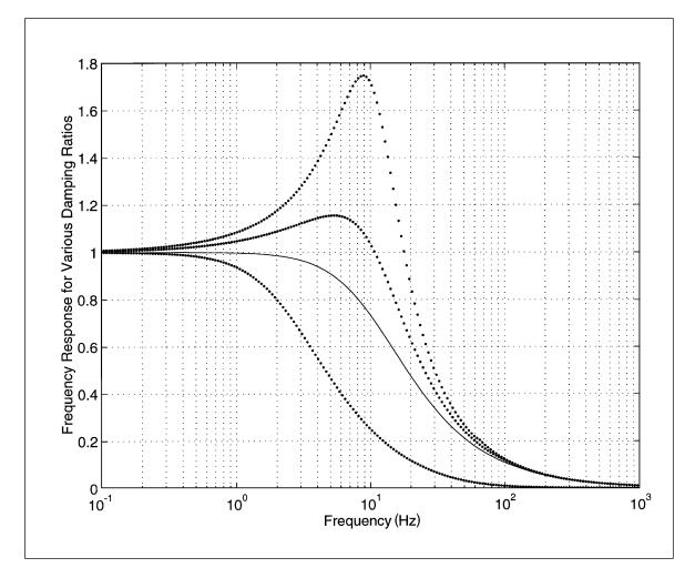
A car with a so-called soft suspension yields relatively good ride characteristics. Unfortunately, a soft suspension tends to have relatively poor handling. The situation is depicted by the next highest dotted curve in Figure 2.11.
