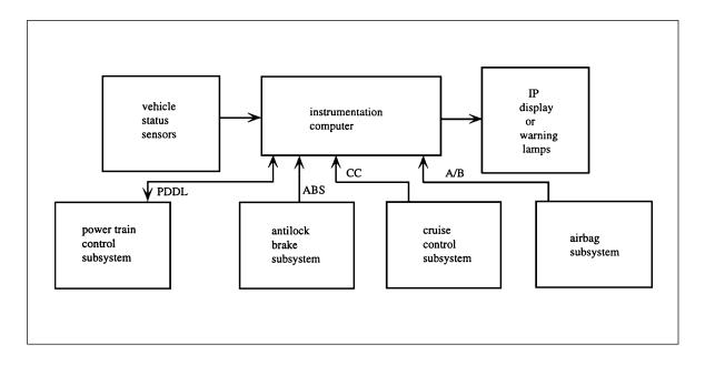
In addition to these variables, the input may include switches for detecting open doors and trunk, as well as IP selection switches for multifunction displays that permit the driver to select from various display modes or measurement units. For example, the driver may be able to select vehicle speed in miles per hour (mph) or kilometers per hour (kph).
