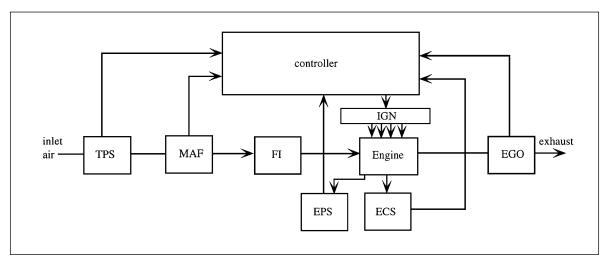
The signals from the various sensors enable the controller to determine the correct fuel flow in relation to the air flow to obtain the stoichiometric mixture. From this calculation the correct fuel delivery is regulated via fuel injectors. In addition, optimum ignition timing is determined and appropriate timing pulses are sent to the ignition control module (IGN).
