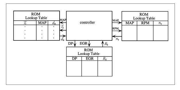
flow rate ( $R_{\rm E}$ ). The volumetric efficiency is read from ROM with an address determined from RPM and MAP measurements. The intake air density is read from another section of ROM with an address determined from MAP and  $T_{\rm i}$  measurements. The EGR volume flow rate is read from still another section of ROM with an address determined from differential pressure (DP) and EGR valve position. These variables are combined to yield the mass air flow rate:
