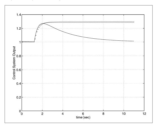
dynamic response is also affected by *G*. Raising the gain too far will cause the system response to become oscillatory. Often if the gain is too large, the system becomes unstable. This property of having a steady error in response to a steady disturbance is fundamental to all control systems incorporating a proportional controller, but can be eliminated by use of a proportional-integral controller.
