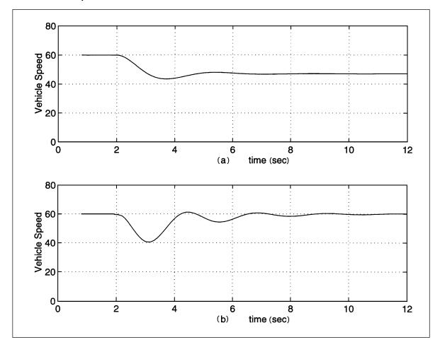
increase. In this case the actuator output will increase until the error is reduced to zero. The response of the cruise control with PI control is shown in Figure 8.3b.
