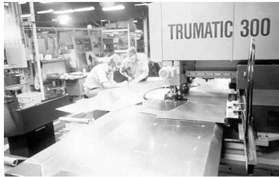
► 4.23 Hong Kong Bank. CNC machines used in fabrication of cladding. Photo: Cupples.
