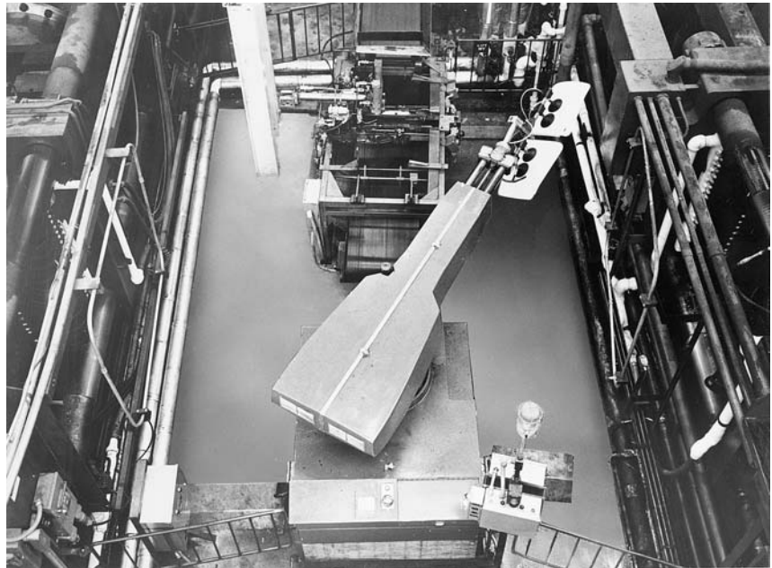
► 3.17 Unimate industrial robot. One of first of its kind, variations of Unimate model have been in widespread use in factories since 1960s. Photo: Versatile Technology.
