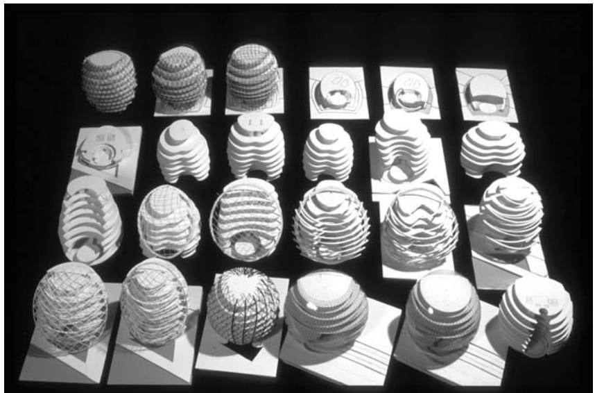
▲ 4.61 Greater London Authority Headquarters, London, UK. 3D models showing changes in geometry from pure sphere to lens shape. Norman Foster, 1998–2002. Source: Foster and Partners.
