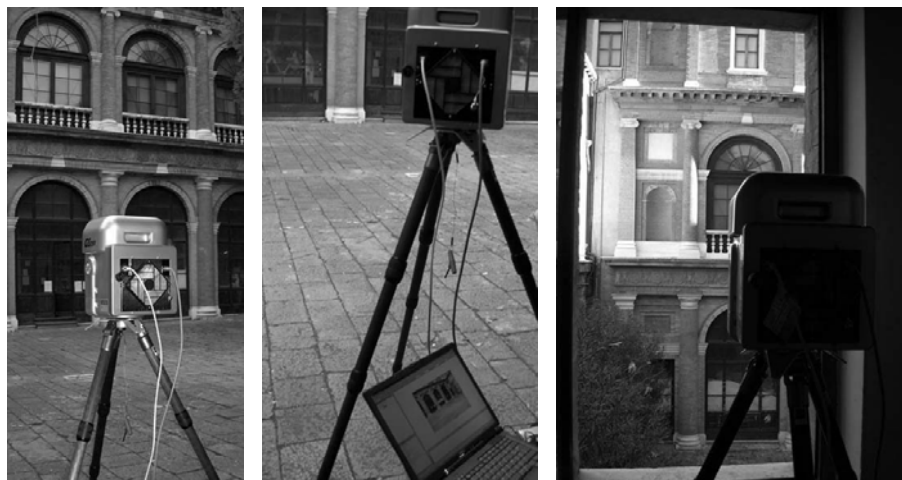
Figure 5-7 3D Laser scanning
