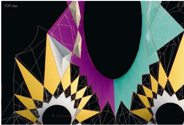
Figure 10 Comparison of trimmed ruled-surfaces as intersected ‘optimised’ hyperboloids of revolution shown against the wireframe of actual data
