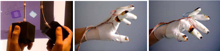
Figure 6 Haptic (tactile) manipulable cubes in Reed Kram’s Three Dimensions to Three Dimensions (left) are creative tools for expression while sensors attached to digits and limbs can be used as gestural controllers for music (right) (Choi, 2000; Pottier and Stalla, 2000; Rovin and Hayward, 2000)
