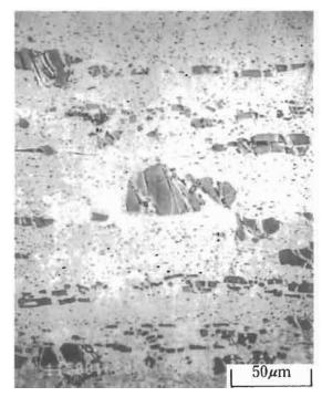
Figure 9.3 Microstructure of SKD-11 tool steel after heat treatment (Natsume et al. [4]).
