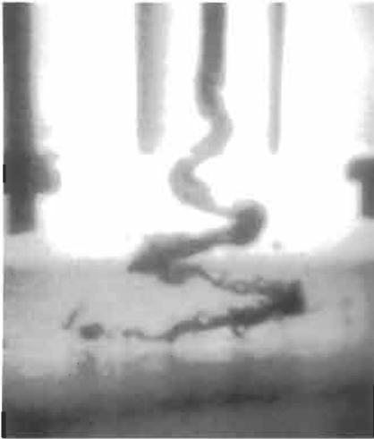
Figure 7.10 Structural elements of self-resonating water jets (photographs: Dynaflo ® Inc., Jessup).
