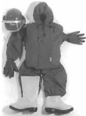
Figure 4.21 Protective clothing for hydroblasting operators (photographs: WOMA GmbH, Duisburg).
