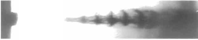
Figure 7.9 Appearance of a self-resonating water jet, v_j = 83.8 m/s, f_p = 4.6 kHz (photograph: Dynaflo ® Inc., Jessup).
