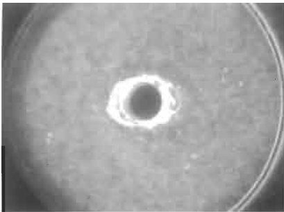
Figure 3.22 Characteristic wear types in hydroblasting sapphire nozzles.
