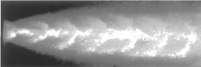
Figure 7.5 Structure of an ultrasonically modulated water jet (photograph: VLN Advanced Technologies Inc.).
