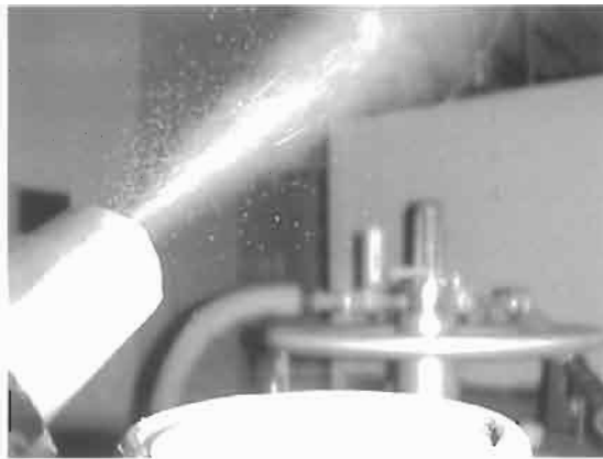
Figure 7.21 Exiting ice-air-jet; air pressure: 0.544 MPa, ice mass flow rate: 20 g/min (photograph: New Jersey Inst. Technology, Newark).
