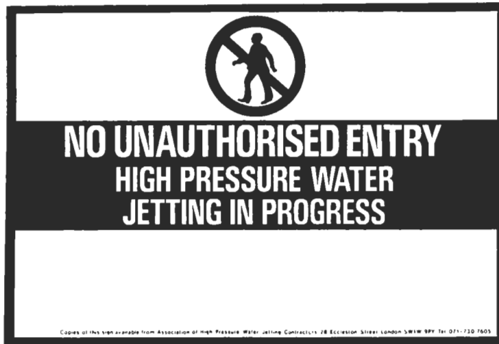
Figure 4.7 Warning (no entry) sign for hydroblasting site (Association of High Pressure Water Jetting Contractors, London).
