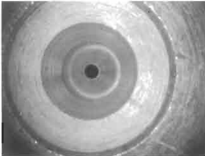
(c) Increased diameter and edge chipping ( d_N = 0.25 mm).
