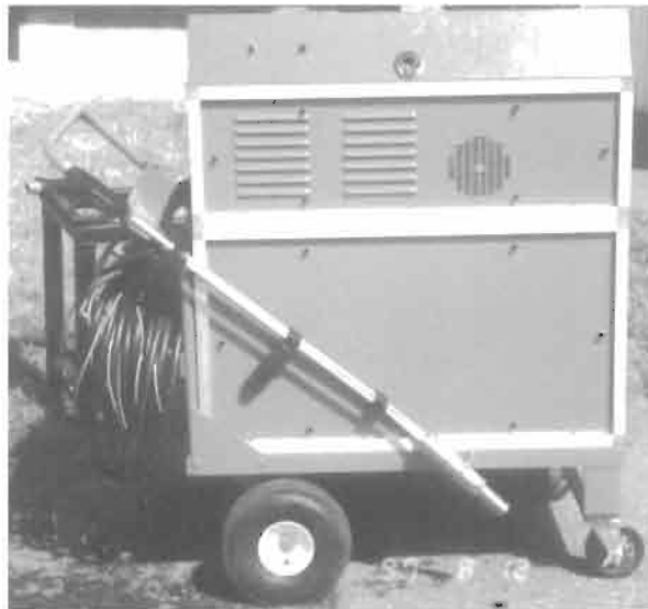
Figure 7.6 On-site device for the formation of ultrasonically modulated jets (photograph: VLN Advanced Technologies Inc.).
