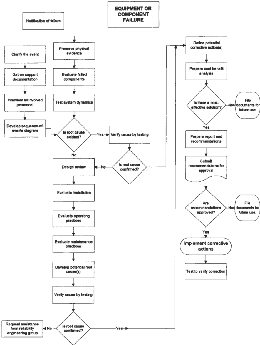
Figure 3-5 Flow diagram for equipment failure investigation.
