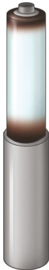
Fig. 31.1 The Bion implantable neurostimulator device. For investigational use only. Not approved for sale in the United States
