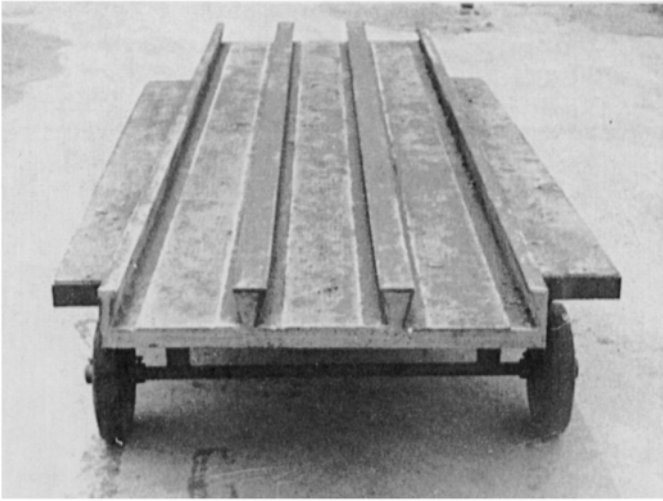
FIG. 10.31. Typical ferrocement deck.
