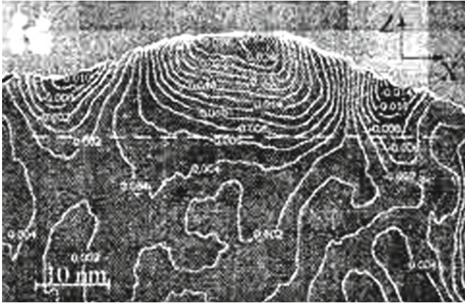
Fig. 2.9 Strain distribution obtained from the TEM images of InGaAs islands in GaAs by using the method of digital analysis of lattice images (after [9])
