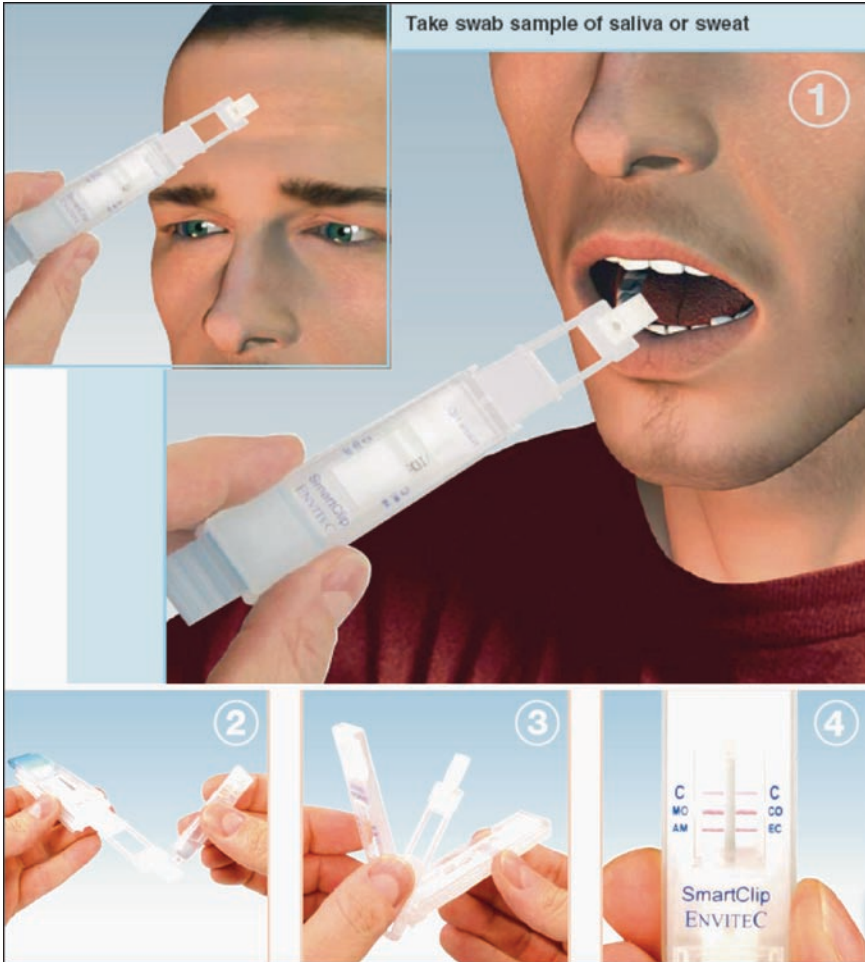
Fig. 21 Sequence of steps for use se of the SmartClip: (1) taking specimen (sweat or saliva), (2) insertion of buffer solution, (3) closing of SmartClip and (4) obtain reading
