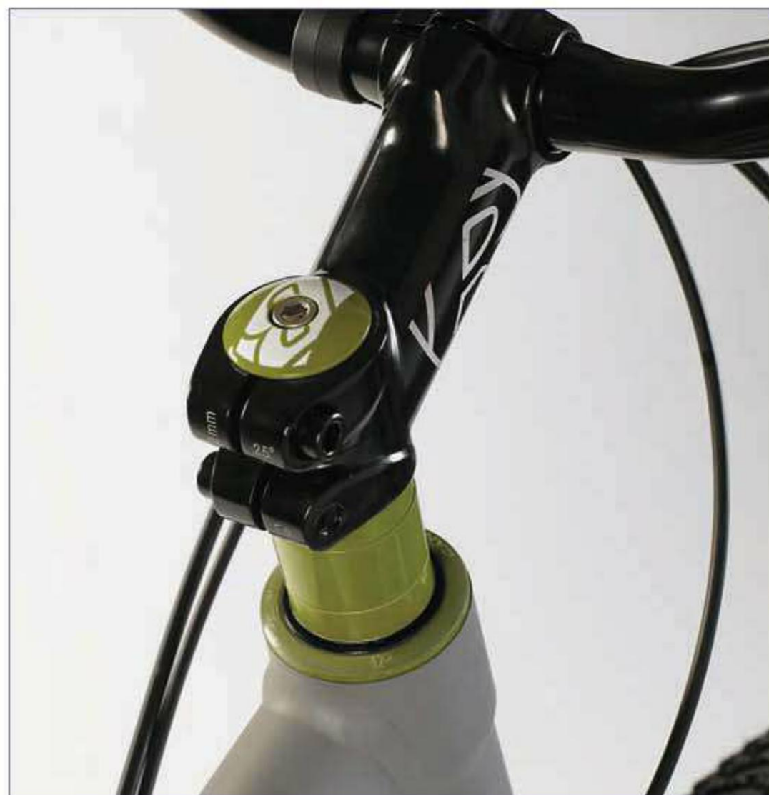
Most new bikes have a threadless headset. The stem clamps onto the outside of the steerer tube.
