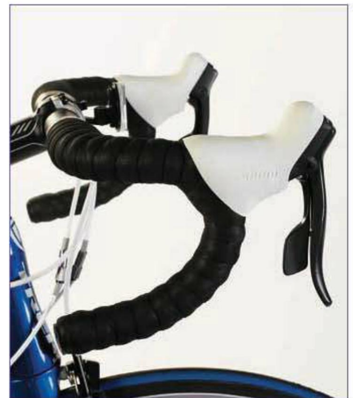
Most road bikes now have shift levers integrated with brake levers.
