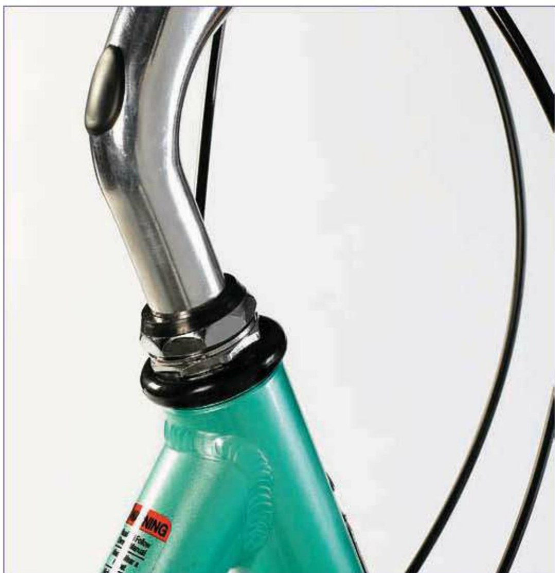
A threaded headset is held in place with a nut, and the stem is called a quill stem and is held in place with an interior clamp.
