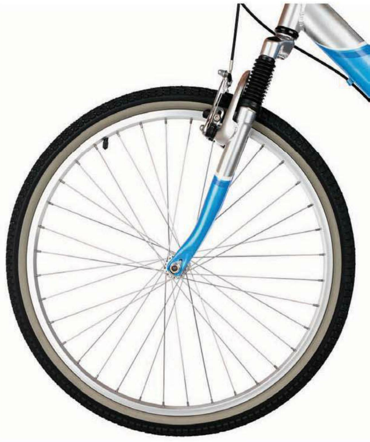
A typical front wheel has spokes laced together and anchored in the hub and the rim.
