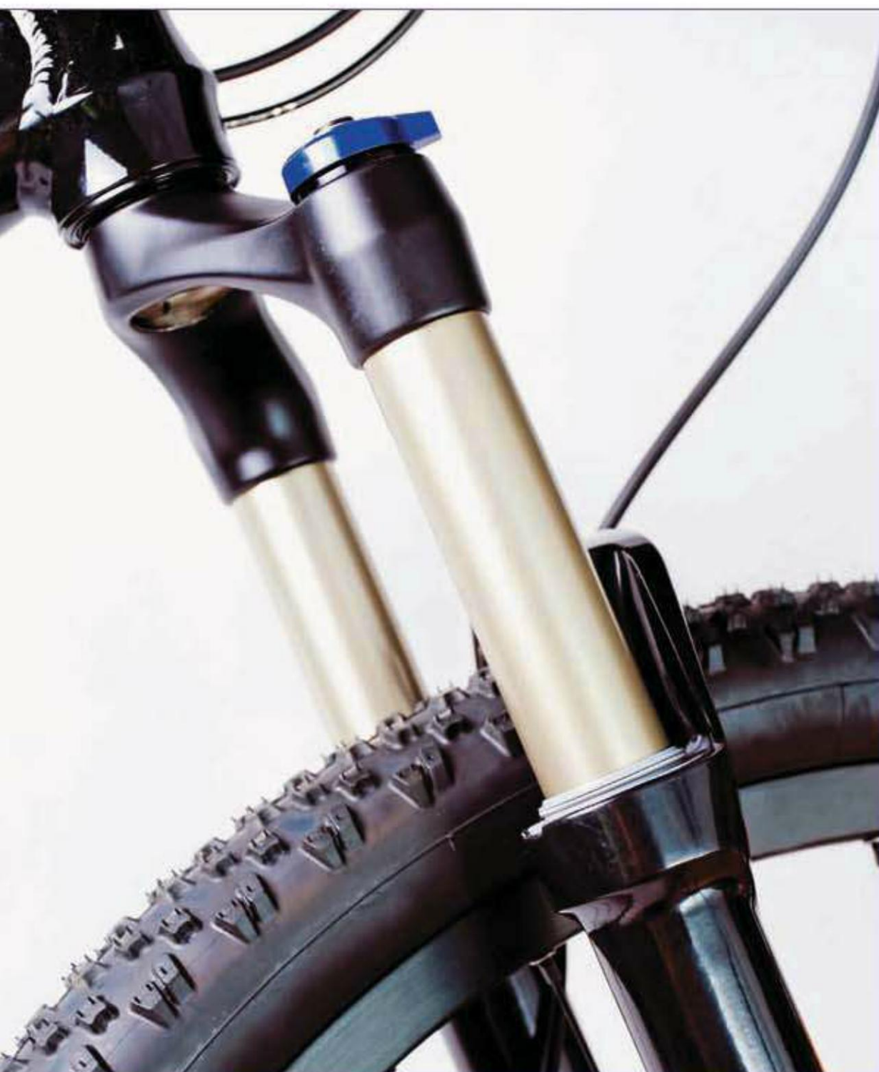
A suspension fork on a mountain bike absorbs much of the shock so it doesn't transmit to the rider's hands. Suspension forks also can be installed on hybrid bikes to make rough commutes more comfortable.
