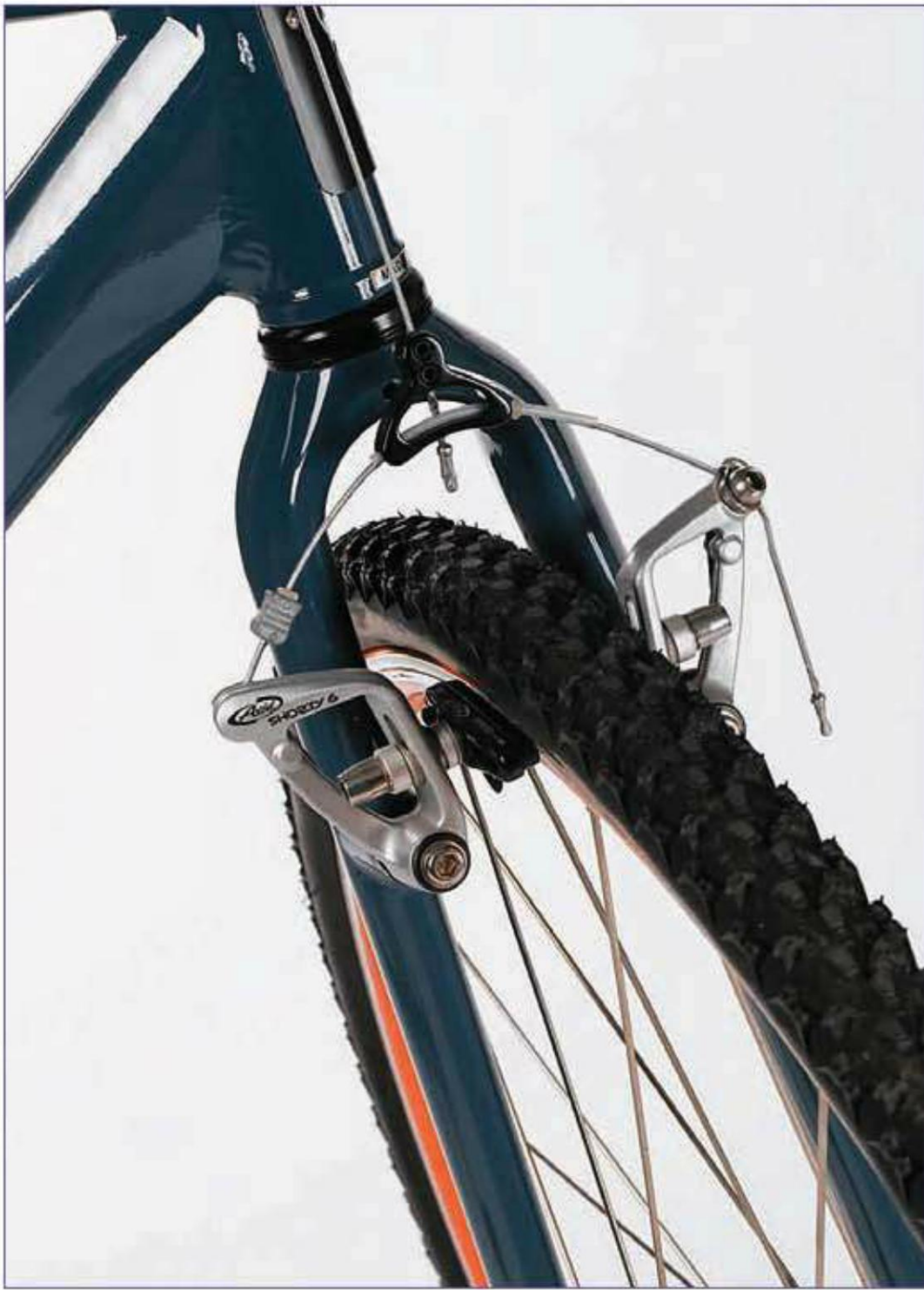
The cantilever brake has clearance for large tires and mud.
