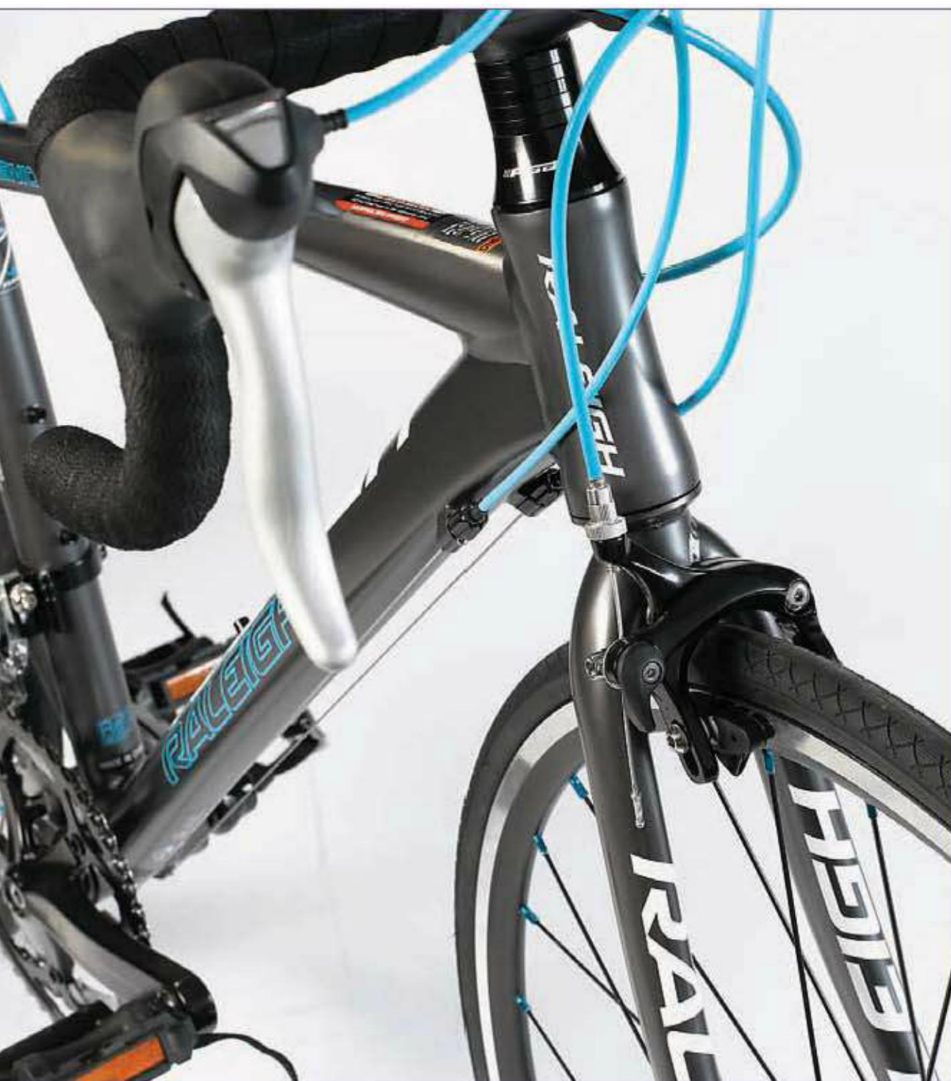
Road bikes usually have dual-pivot caliper brakes. The brakes have low clearance, so they aren't suitable for fat tires or muddy conditions.
