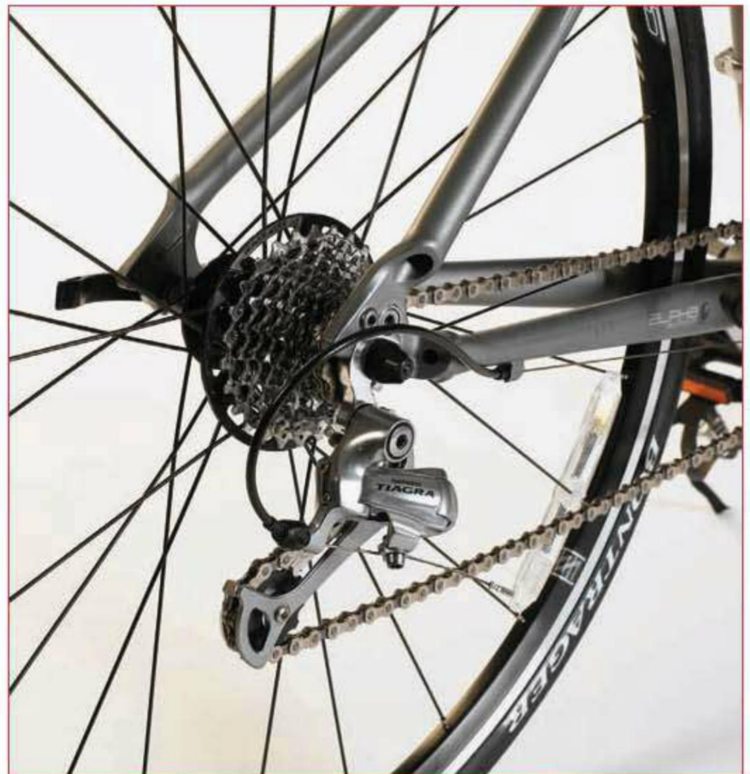
When the chain is on the smallest chainring and the smallest sprocket, the derailleur rides very close to the sprockets and the loose chain slaps around.
