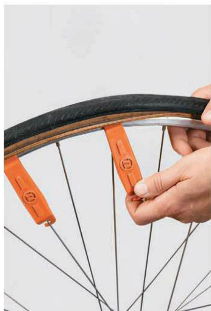
5 Move about four or five inches away from the first lever and insert a second lever. Pry the tire bead over the rim and hook the lever to a spoke.
