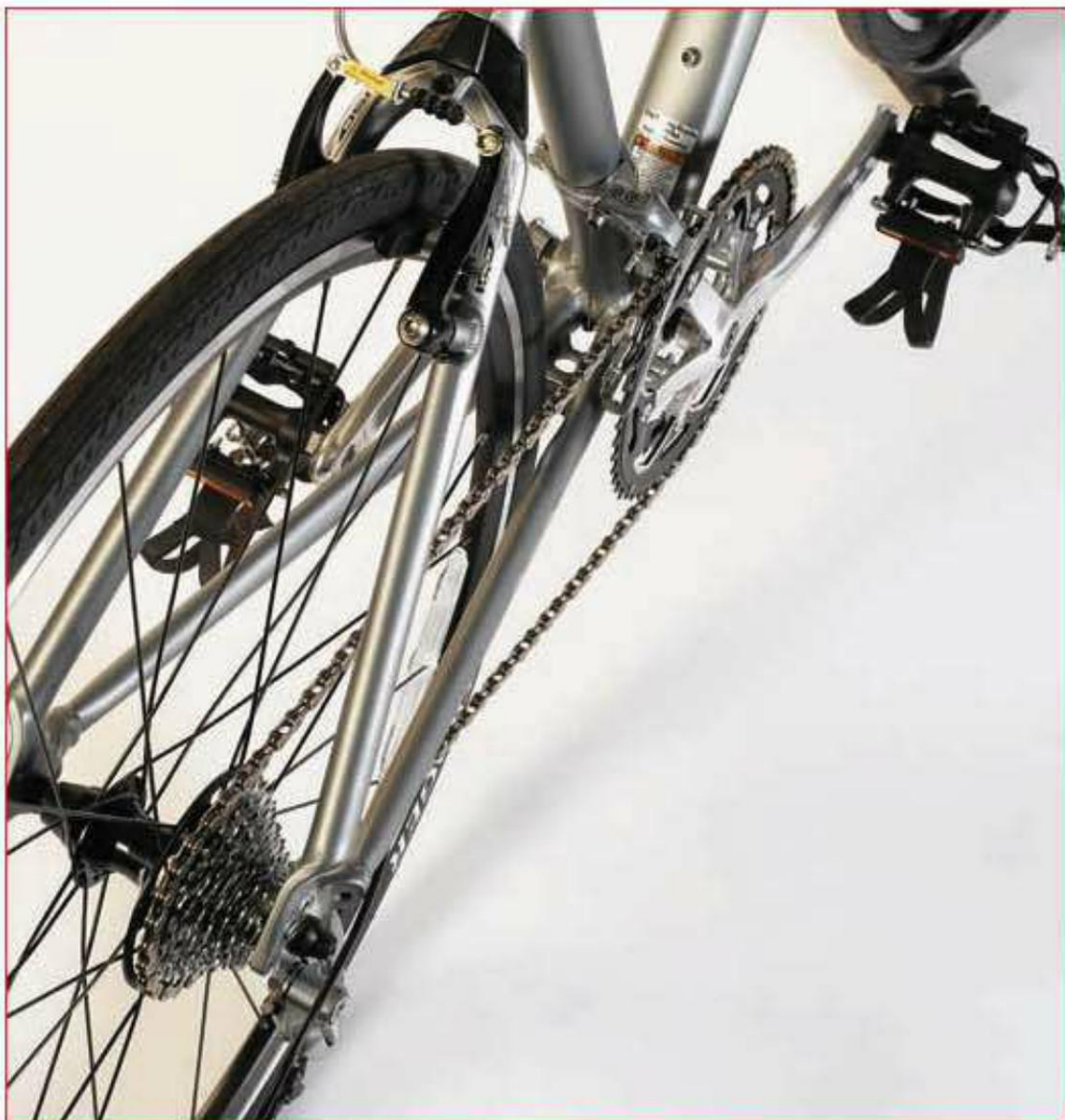
Cross chaining happens when the chain is on the largest chainring and largest sprocket or when the chain is on the smallest chainring and smallest sprocket. Cross chaining damages the chain, and is usually noisy.
