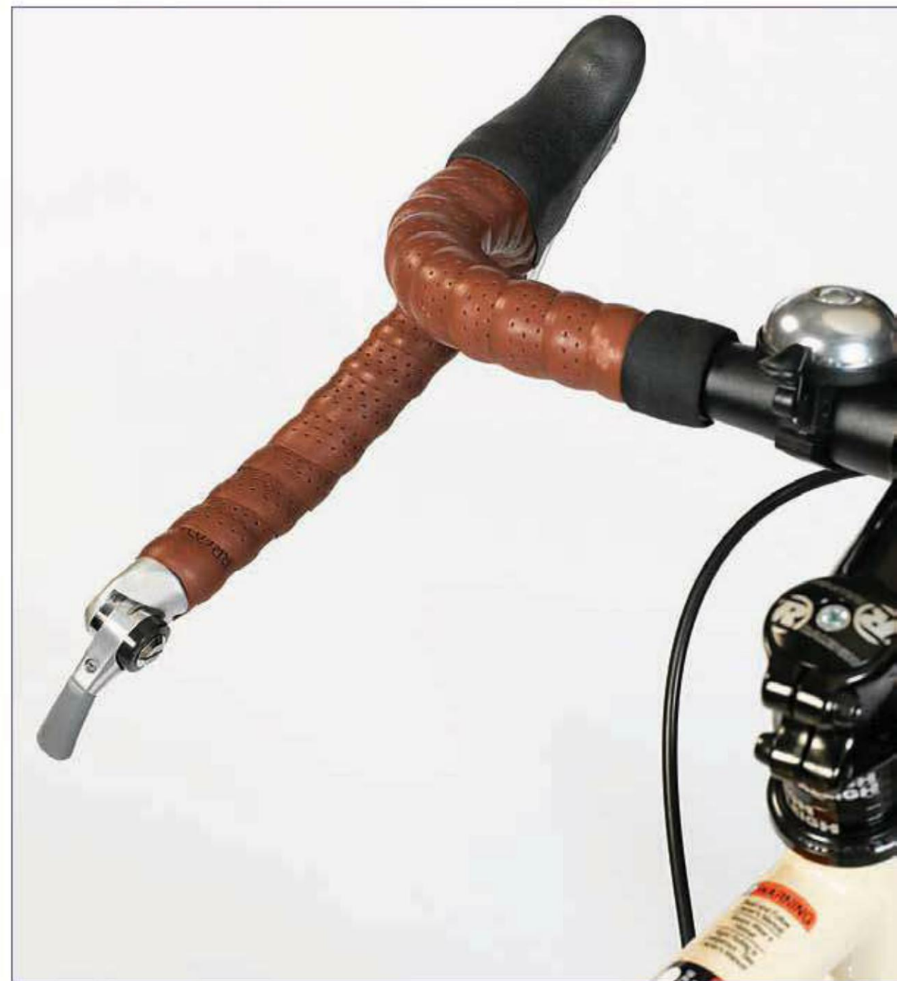
Bar end shifters are popular with those who enjoy touring. The shift levers are conveniently close so that minimal effort is needed for shifting.
