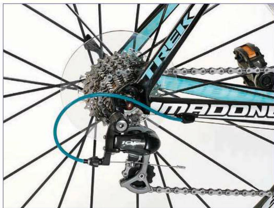
Most road bikes have a short cage derailleur because the difference between the highest and lowest gears is small so there is not as much chain slack.
