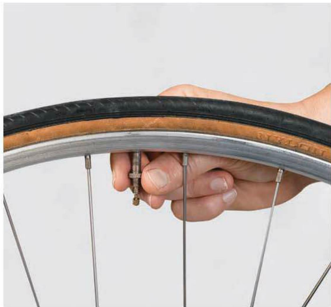
2 Remove the wheel from the bike (see pages 106 to 109). If the tube is a Presta tube, remove the valve nut.
