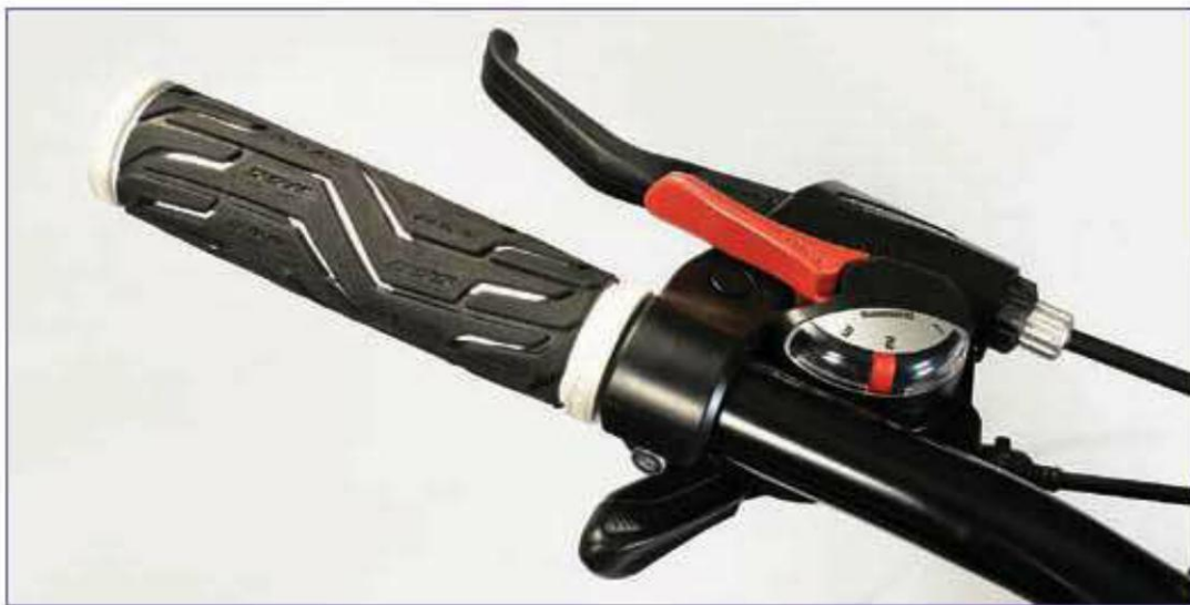
Thumb shifters usually have two levers, one operated by the thumb and one by the forefinger.
