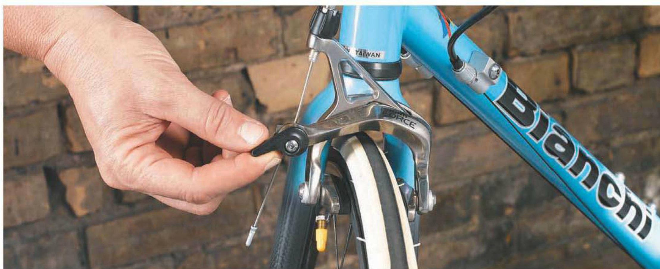
Side pull or dual pivot caliper brakes: Rotate the brake quick release arm upward. Some brakes of this type may have a button on the brake lever.
