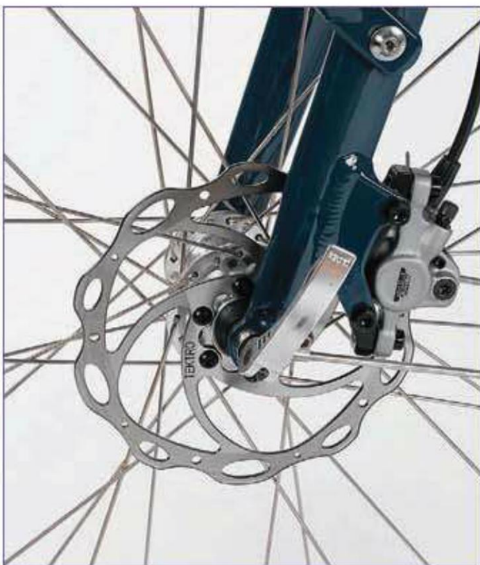
Disc brakes are very powerful , are not as affected by moisture as rim brakes, and do not require sturdy wheel rims to operate.
