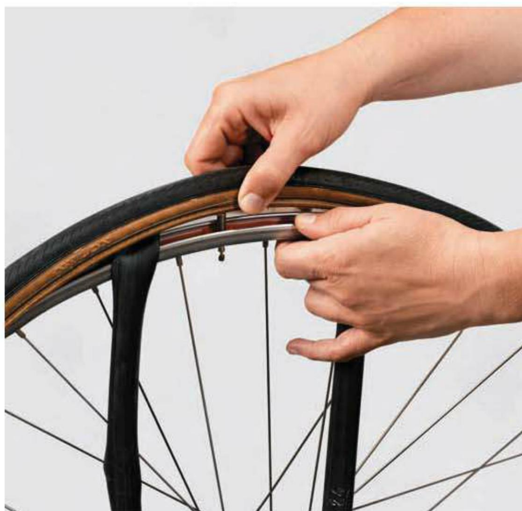
9 To remove the valve, push the tire back over the rim so you can pull the valve straight out to remove it.
