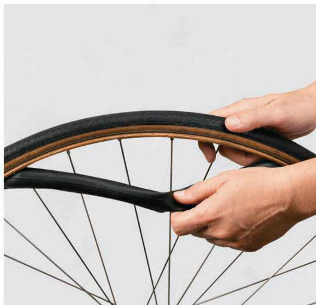
8 Remove the inner tube. It is not necessary to remove the tire except to fully inspect the inner lining of the tire and to inspect the rim tape.
