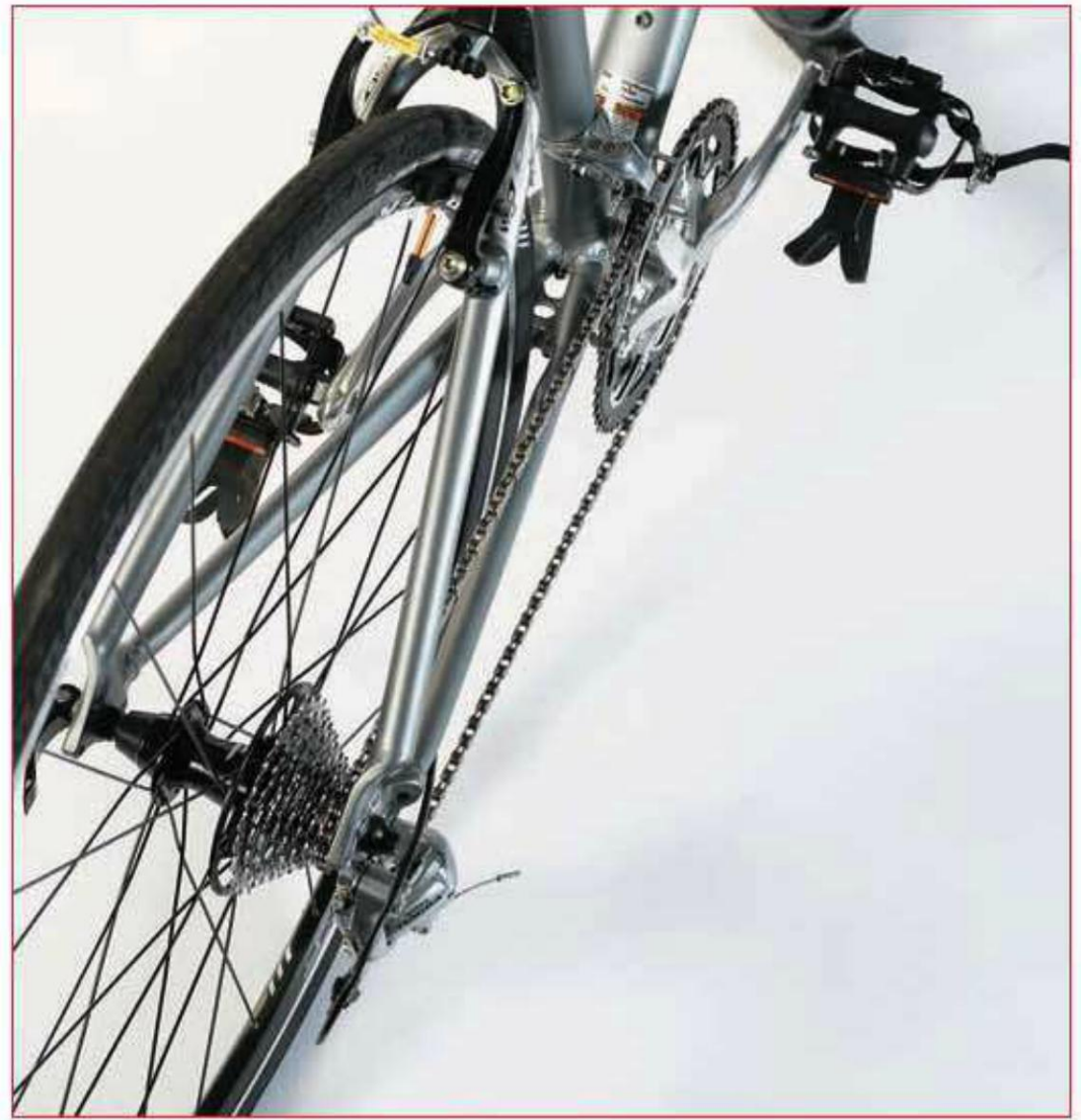
The bike is in the highest (hardest) gear when the chain is on the largest chainring in front and the smallest sprocket in back.
