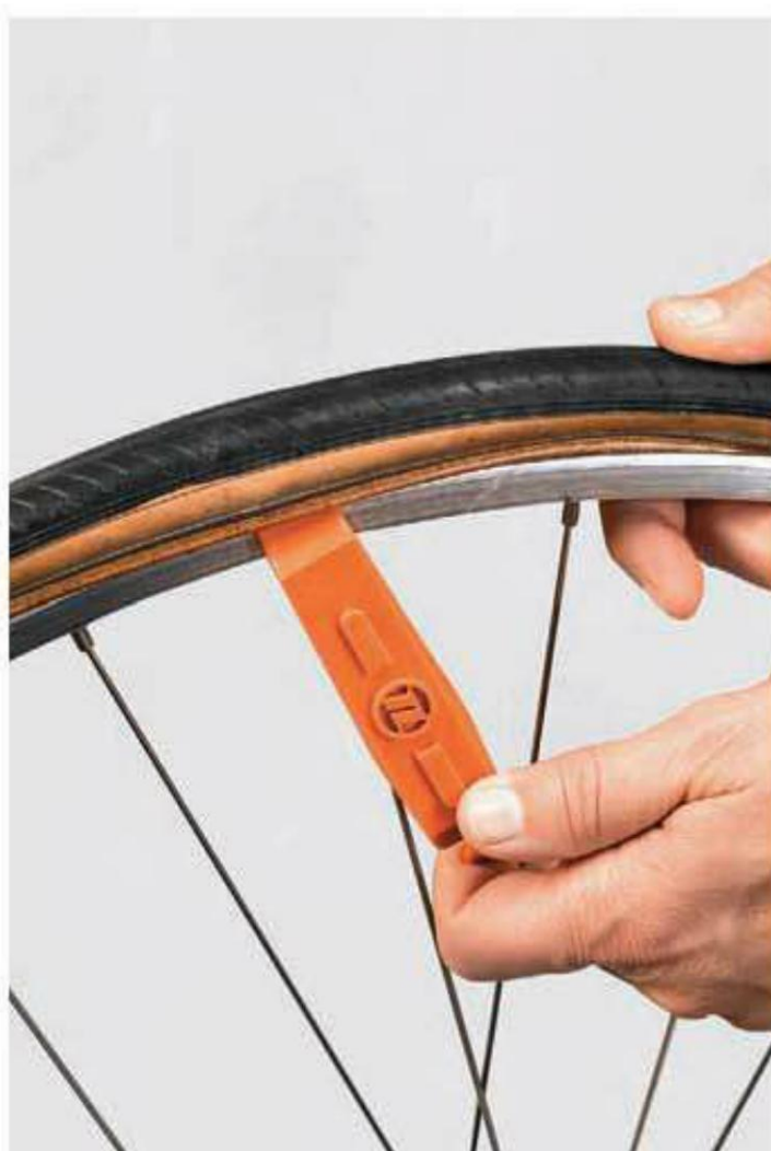
4 Push down on the lever to pry the tire bead over the wheel rim. Hook the end of the tire lever around a spoke.
