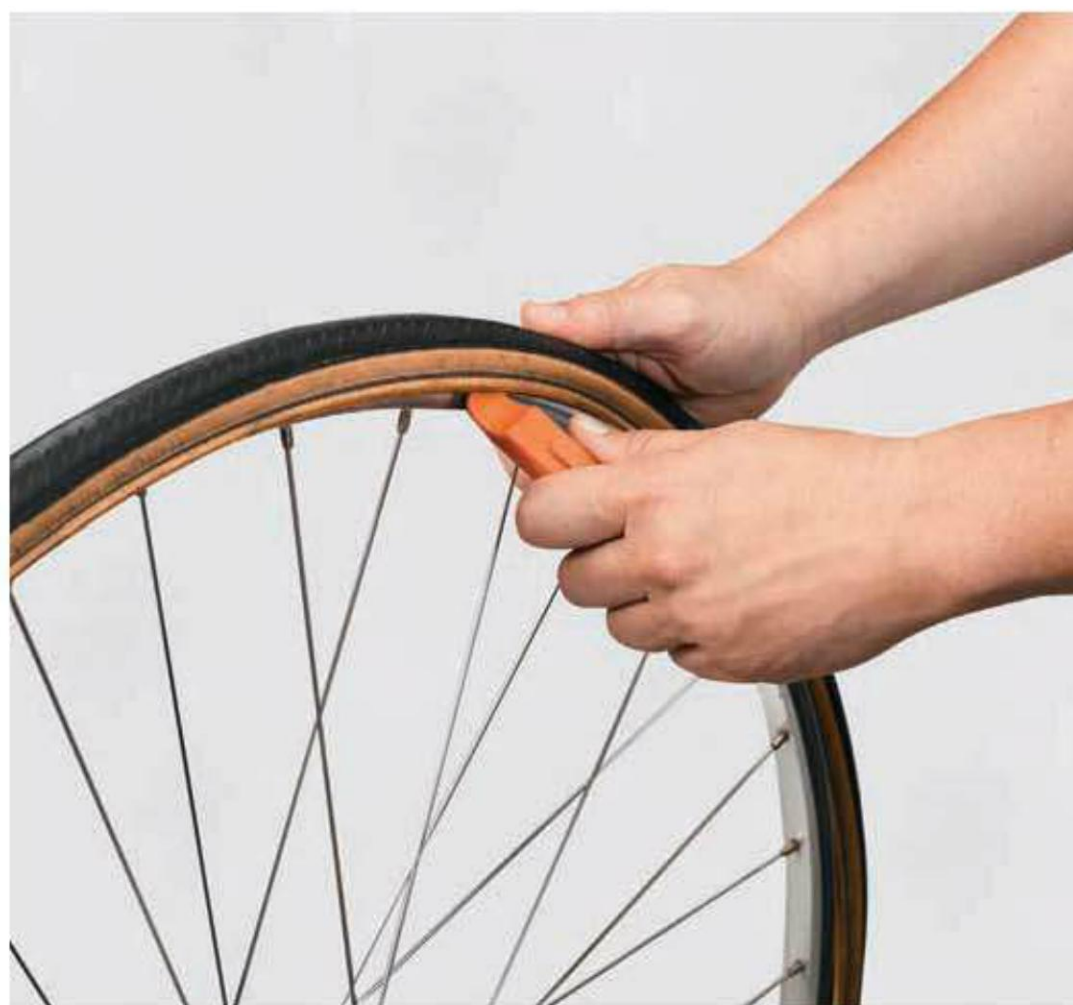
7 The tire should now be loose enough that you can run the tire lever around the entire tire and lift it over the rim.
