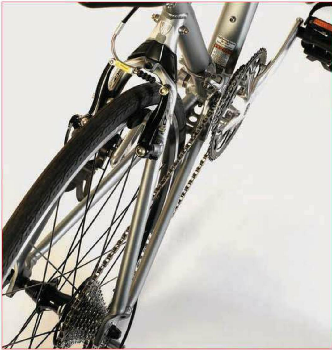
The bike is in the lowest (easiest) gear when the chain is on the smallest chainring in front and the largest sprocket in back.
