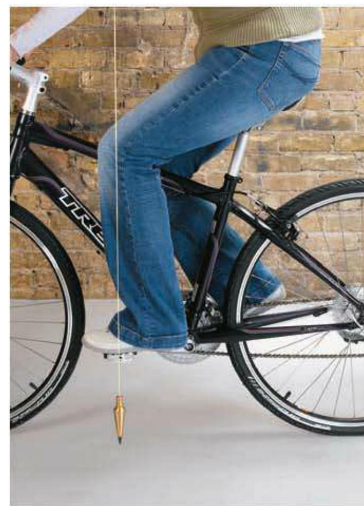
3 The plumb bob test. Suspend a plumb bob (any small, heavy object tied to string will do) downward with the string held next to your knee. Ideally, when the pedals are parallel to the ground (3 o'clock and 9 o'clock position) your knee and the pedal axle should be on the same vertical line. Have a helper steady the bike for you.
