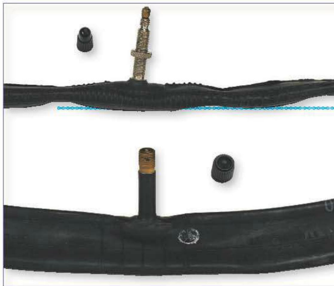
Two styles of valves are found on bicycle inner tubes. The Schrader valve (bottom) is rubber covered and is the same as a car tire valve. The Presta valve (top) is threaded metal and has a locking stem. If you've never used a Presta valve, ask for a demo at your bike shop. They require some explanation.
