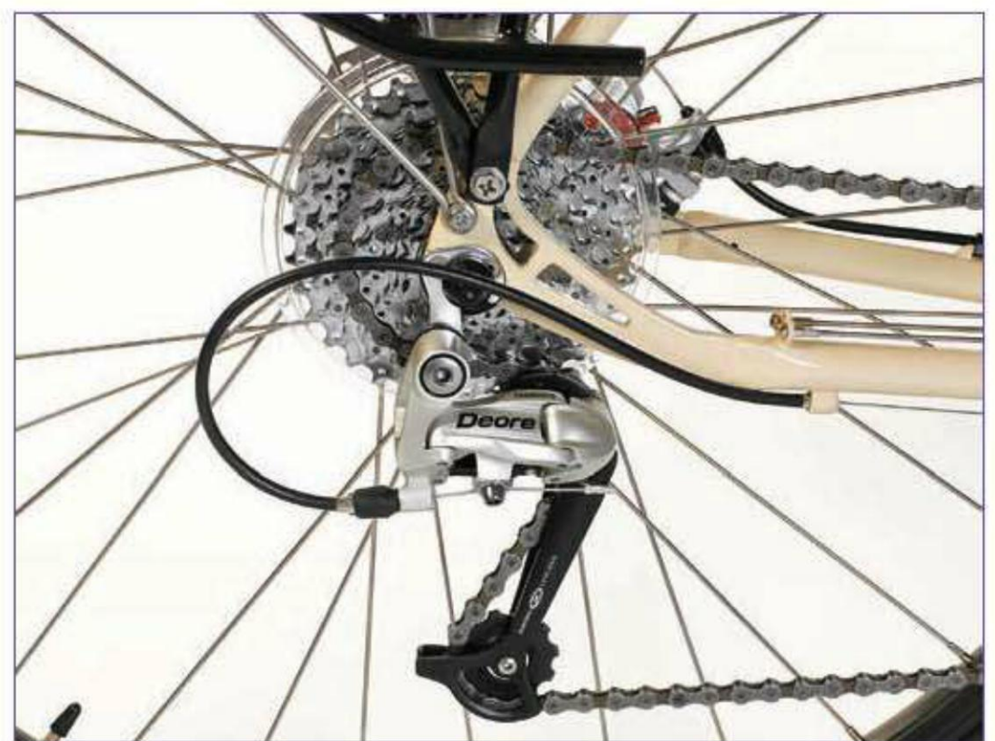
Mountain bikes and many hybrid and comfort bikes have a very wide range of gears. The cage on the derailleur is longer to take up the extra chain length.
