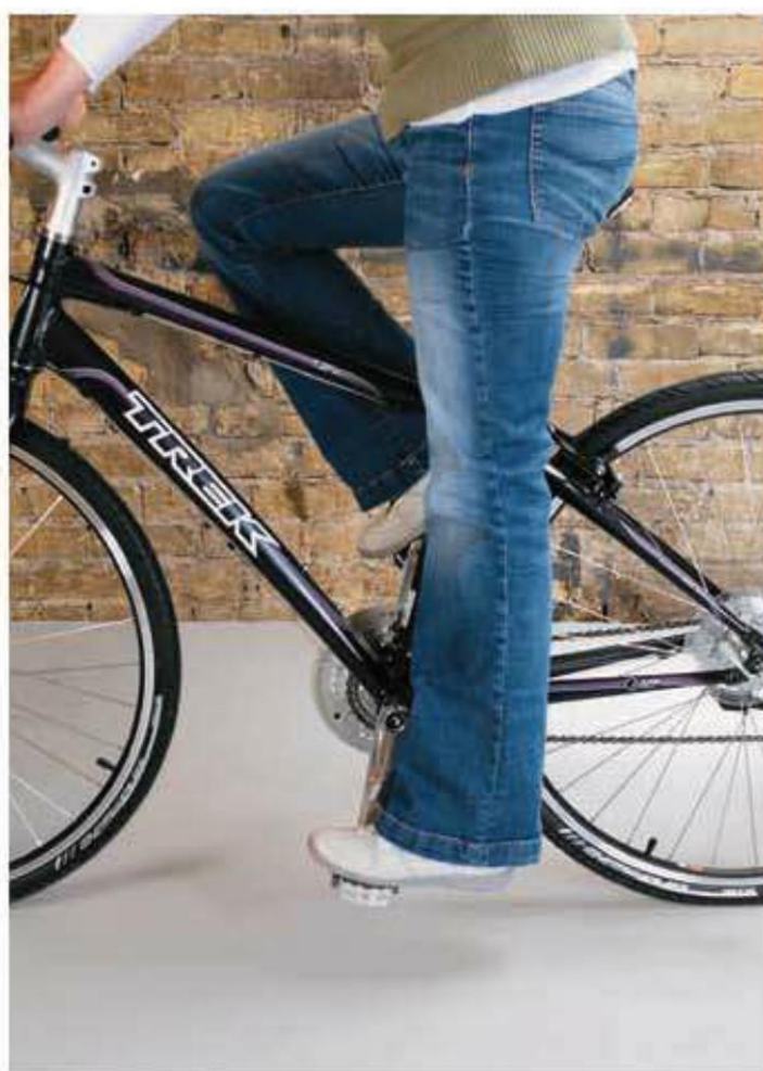
2 The pedal test. Put your foot flat on the pedal. When the pedal is at the lowest point in its revolution, your leg should be fully extended and your foot should remain flat on the pedal. Have a helper steady the bike for you.
