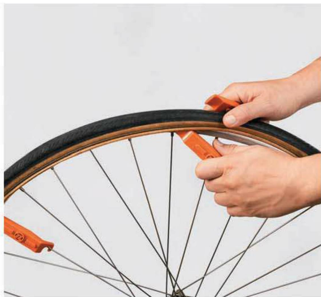
6 Repeat with a third lever. (The second lever will drop out at this time.)
