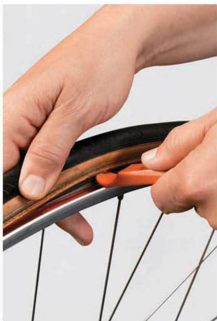
3 Starting opposite the valve , push the tire toward the middle of the rim. Slip the smooth end of a tire lever under the bead of the tire.
