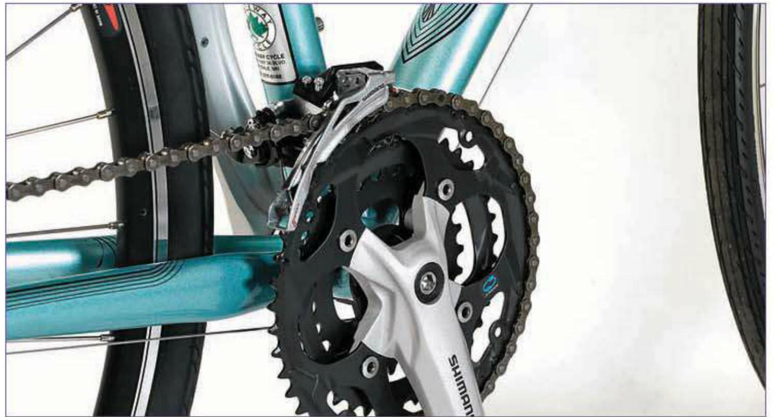
The front derailleur pushes and lifts or drops the chain between chainrings.
