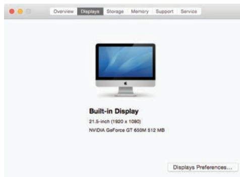
Figure A.2 The Displays tab in the About This Mac window showing the presence of an NVIDIA GPU
